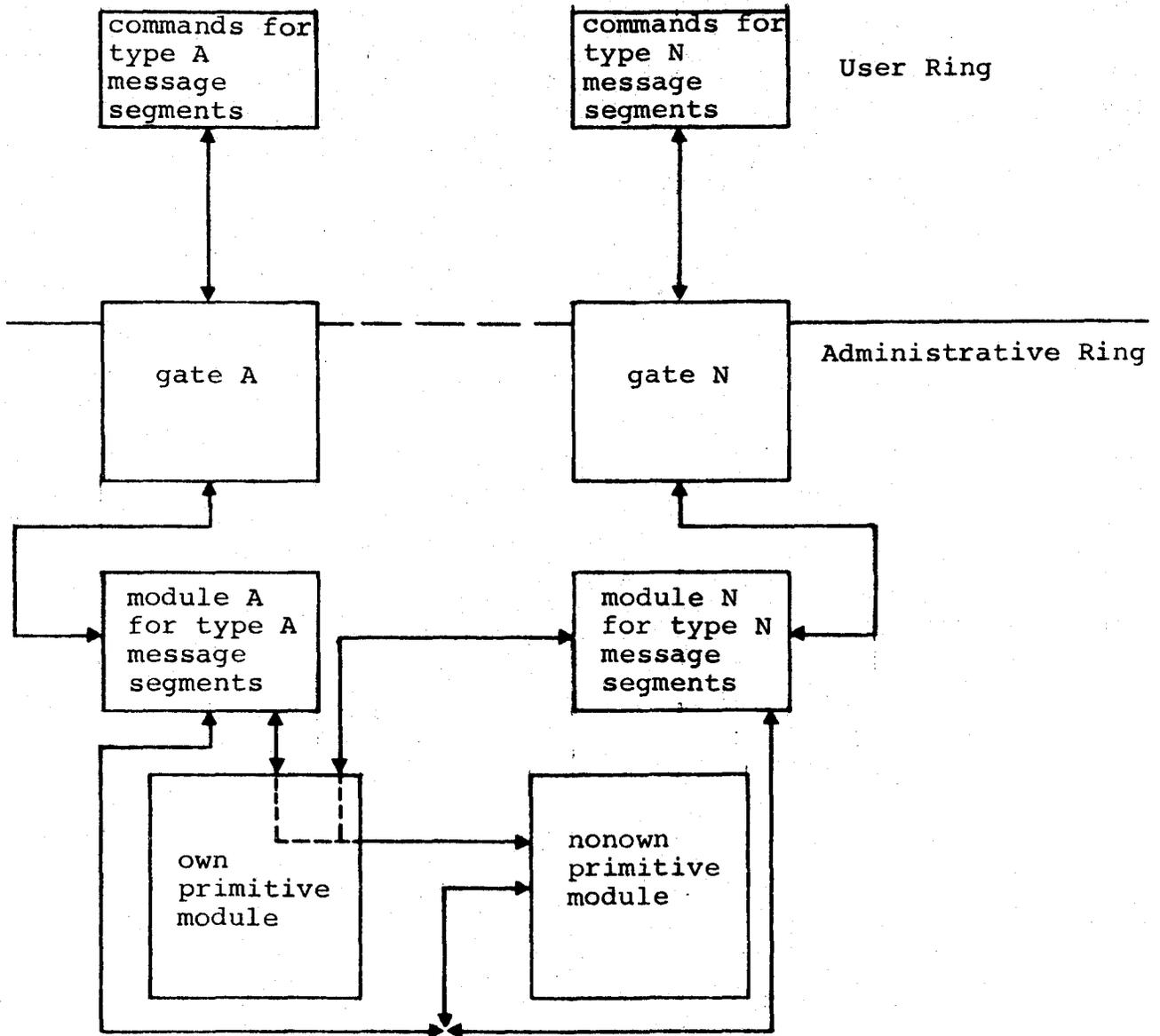
Figure 2-1. Sample Message Segment Facility Configuration
