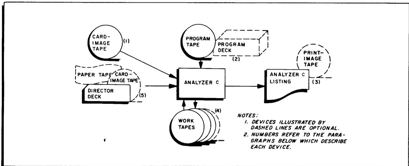
Figure 2-1. Configuration for Analyzing a Symbolic Program Tape
