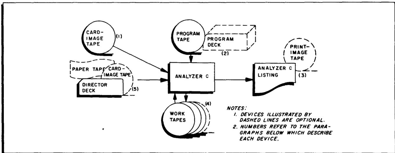
Figure 2-2. Configuration for Analyzing a Card-Image Tape
