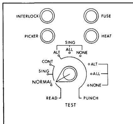
Figure 5-2. Auxiliary Control Panel Controls and Indicators
