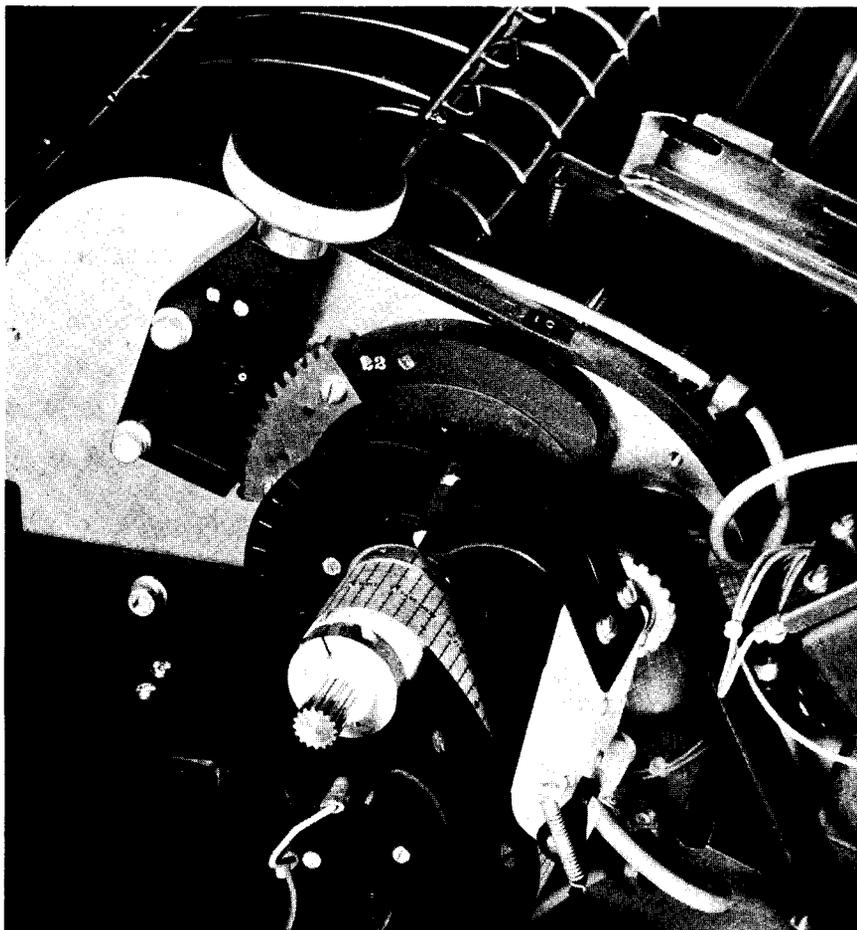
Different tapes must be used for either six- or eight-lines-per-inch printing, with the exception noted in the operating procedures on page 6-15. The vertical format tape in the Type 122 enables the program to print and space, print without spacing, or space without printing until a hole in channel one or two is sensed. The photo above shows the vertical format control assembly in detail.
