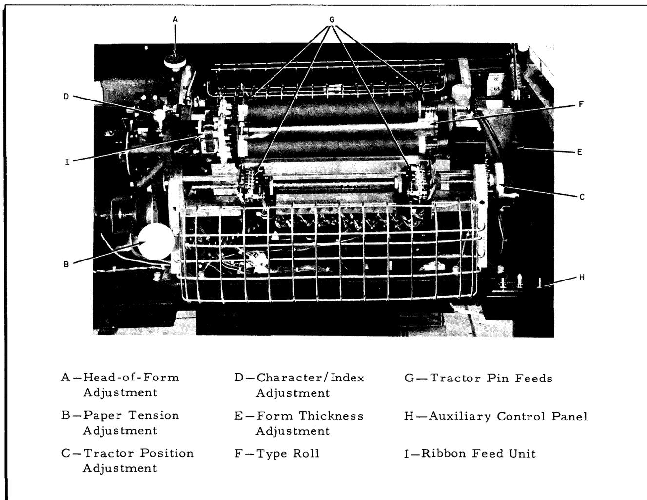
Figure 6-1. Printer Mechanical Controls and Adjustments
