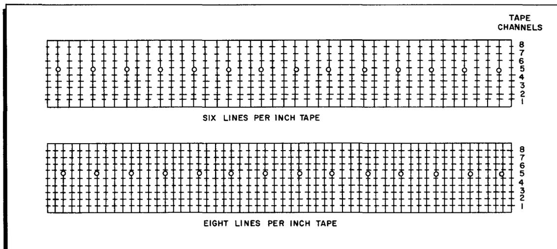
Figure 6-2. Type 122 Printer Vertical Format Control Tape
