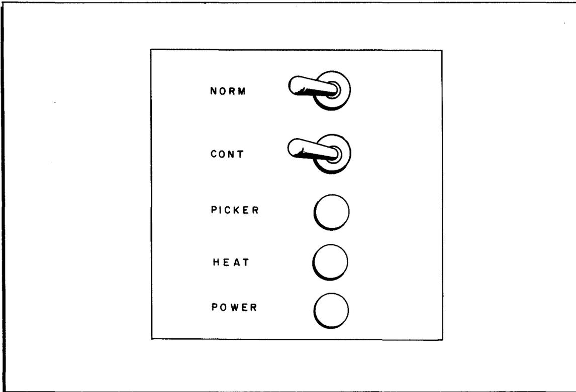
Figure 3-2. Auxiliary Control Panel Controls and Indicators
