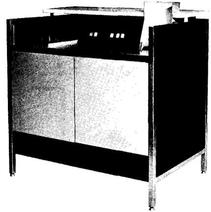
For card reading on the Type 214-2, information is read optically by means of 12 photo-cells, starting with column one. All columns are read serially until column 80 has been read. The information contained in each column is decoded (i. e. , translated into a six-bit character) by the integrated card control and is transferred by this control to main memory. Data transfer is terminated when the last column is read or when a record mark is sensed in memory, whichever occurs first.
