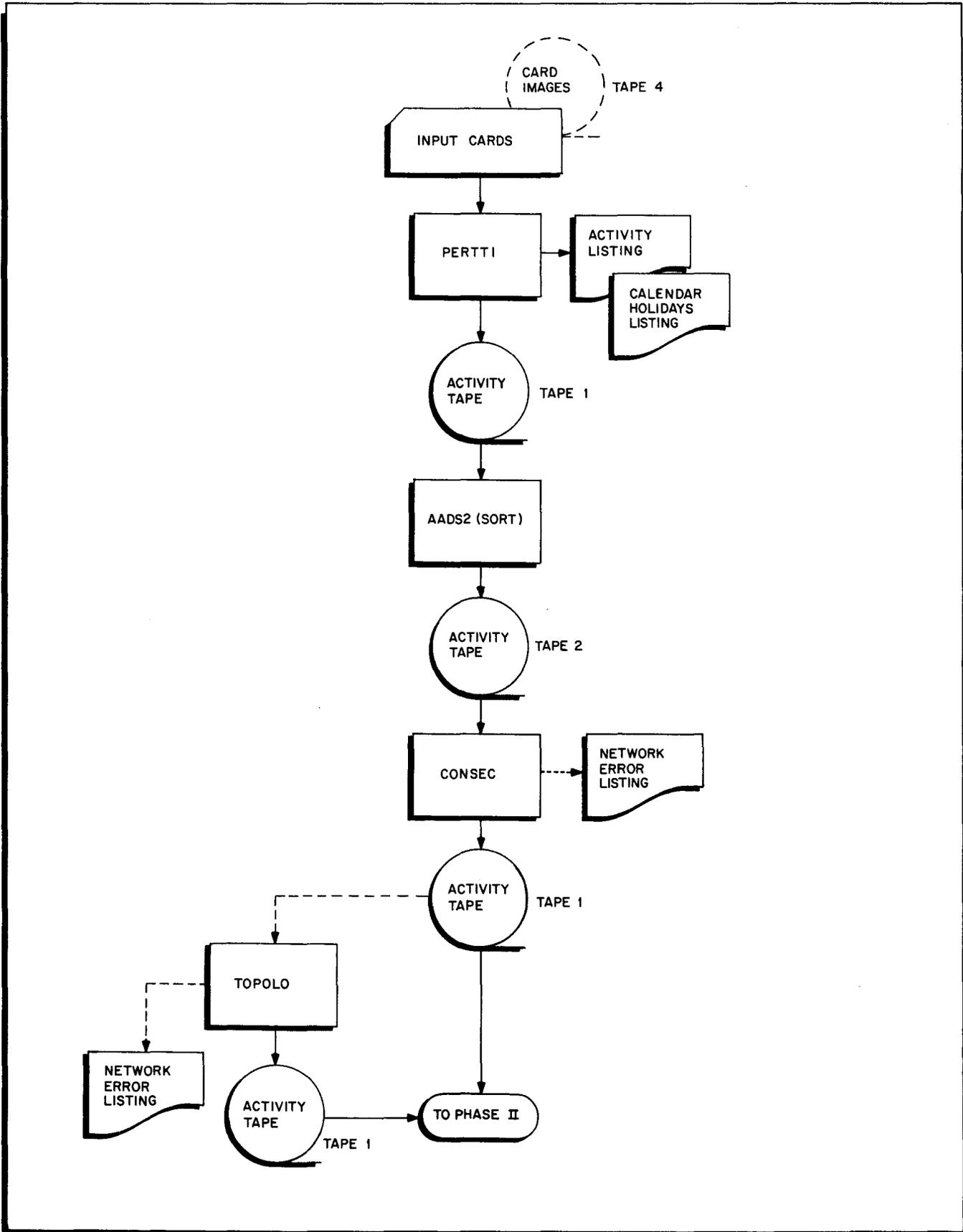
Figure 5-1. PERT Time C Operation Sequence - Phase I
