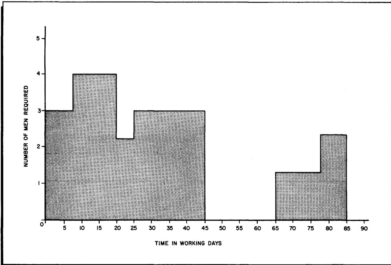
Figure 4-14. Histogram of Manpower Accumulation for Craft A
