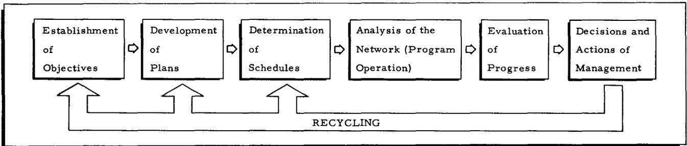
Figure 1-1. PERT Time C System Cycle
