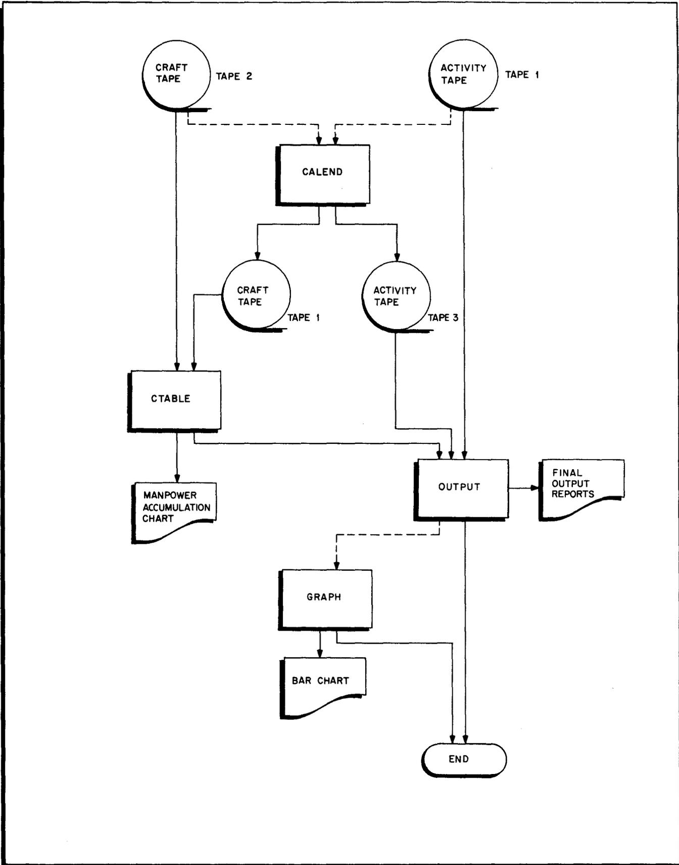
Figure 5-3. PERT Time C Operation Sequence - Phase III
