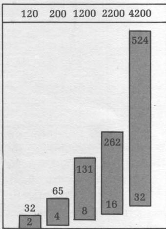
Figure 1. PROCESSOR SIZE SELECTOR — Memory capacity is given in thousands of characters (nominal).
