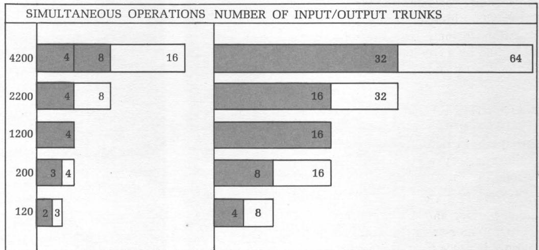
Figure 2. PERIPHERAL INTERFACE SELECTOR — Basic capabilities are shown in color. Additional capabilities shown in incremental sizes. (The number of input/output trunks determines the number of peripheral controls that can be connected to a processor model.)
