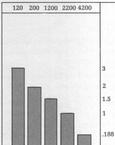
Figure 3. PROCESSOR SPEED SELECTOR — Speed is given in microseconds per character.
