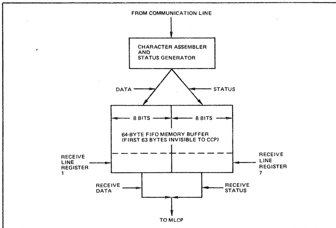
Figure H-14. Receive Line Registers 1 and 7 and FIFO Memory
