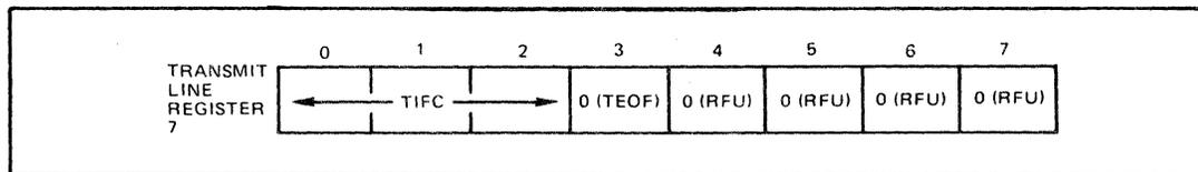
**Figure H-10. Transmit Line Register 7, Interframe Format**
