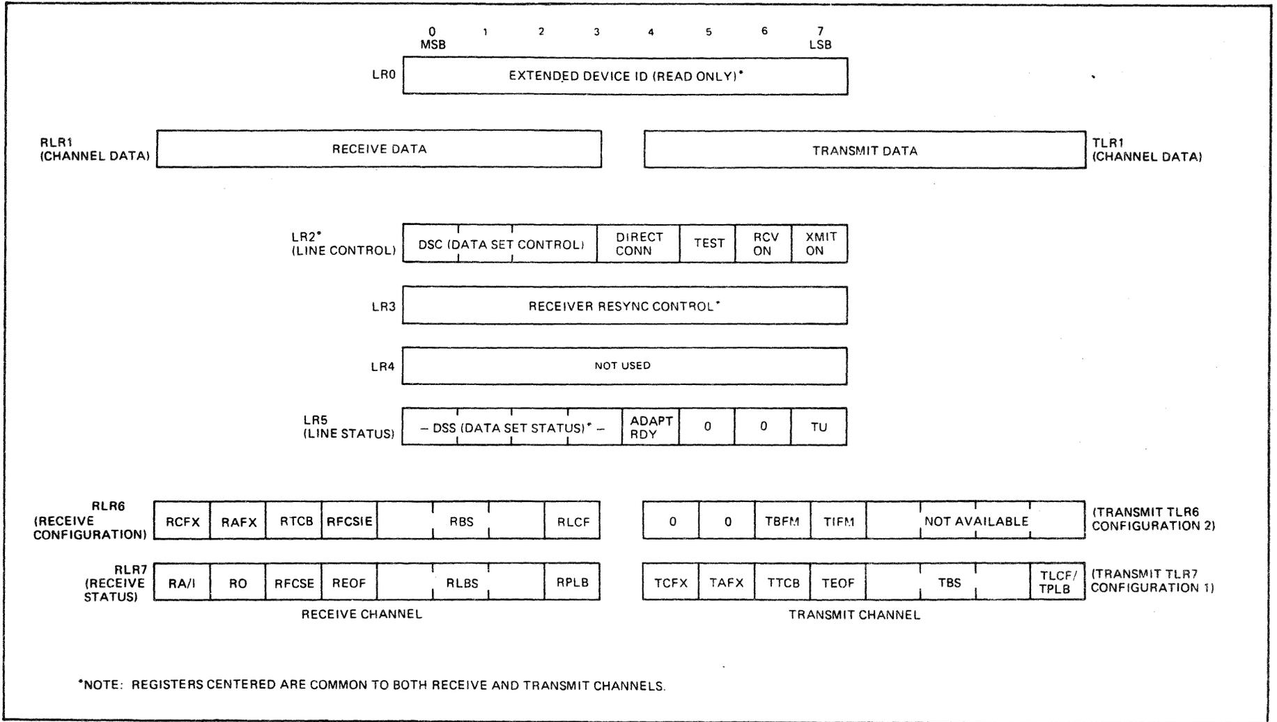
Figure H-3. Synchronous Broadband HDLC Communications-Pac Line Registers
