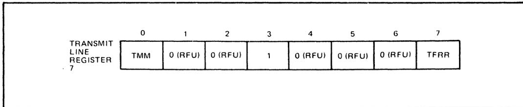
**Figure H-13. Transmit Line Register 7, Initialization Format**
