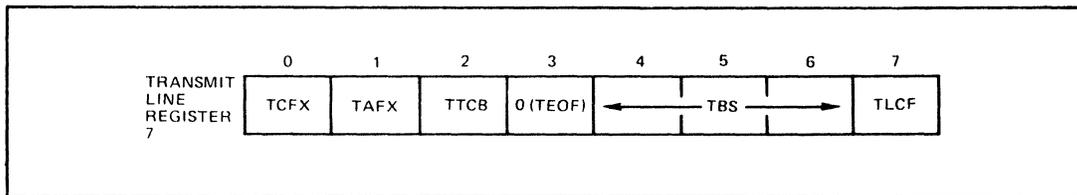
**Figure H-11. Transmit Line Register 7, Start-of-Frame Format**
