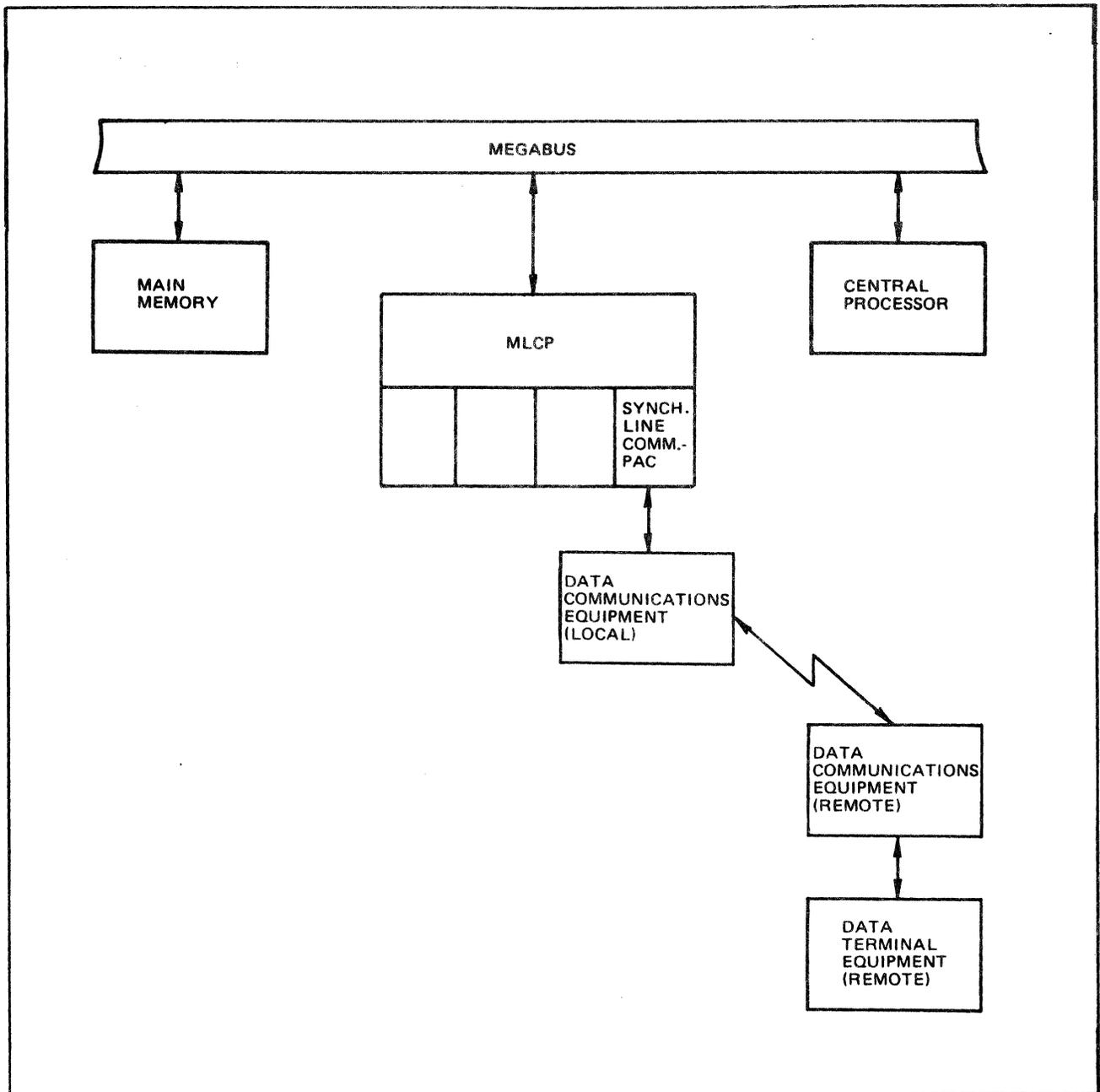
Figure D-1. Interface Provided by Synchronous Line Communications-Pac (MLCP)
