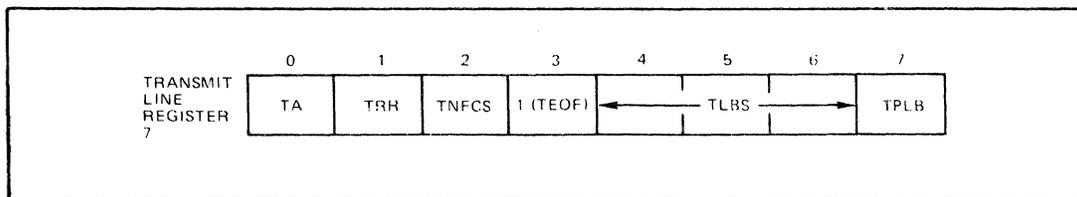
Figure H-12. Transmit Line Register 7, End-of-Frame Format
