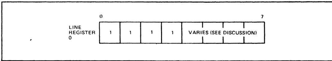
Figure H-4. Line Register Zero
