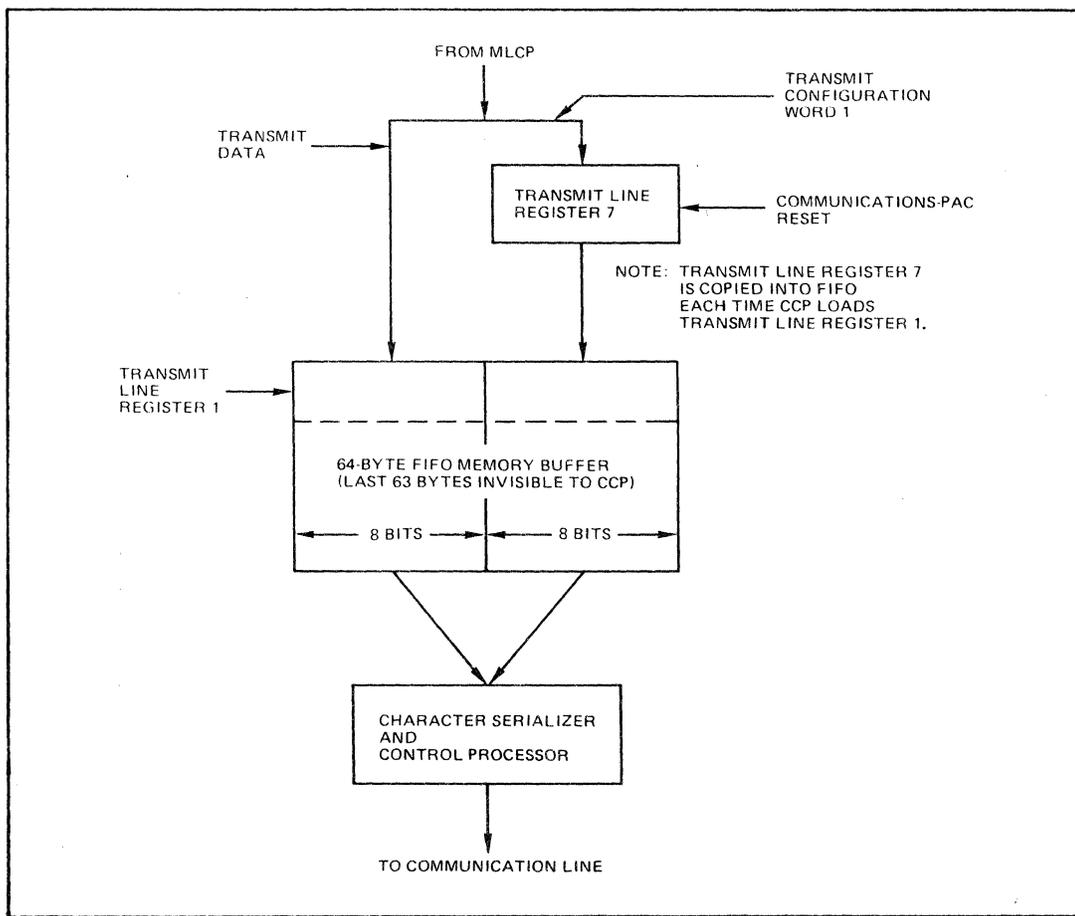
Figure H-8. Transmit Line Registers 1 and 7 and FIFO Memory
