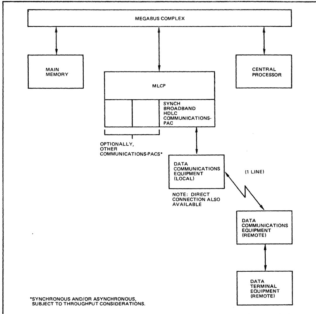
Figure H-1. Interface Provided by Synchronous Broadband HDLC Communications-Pac
