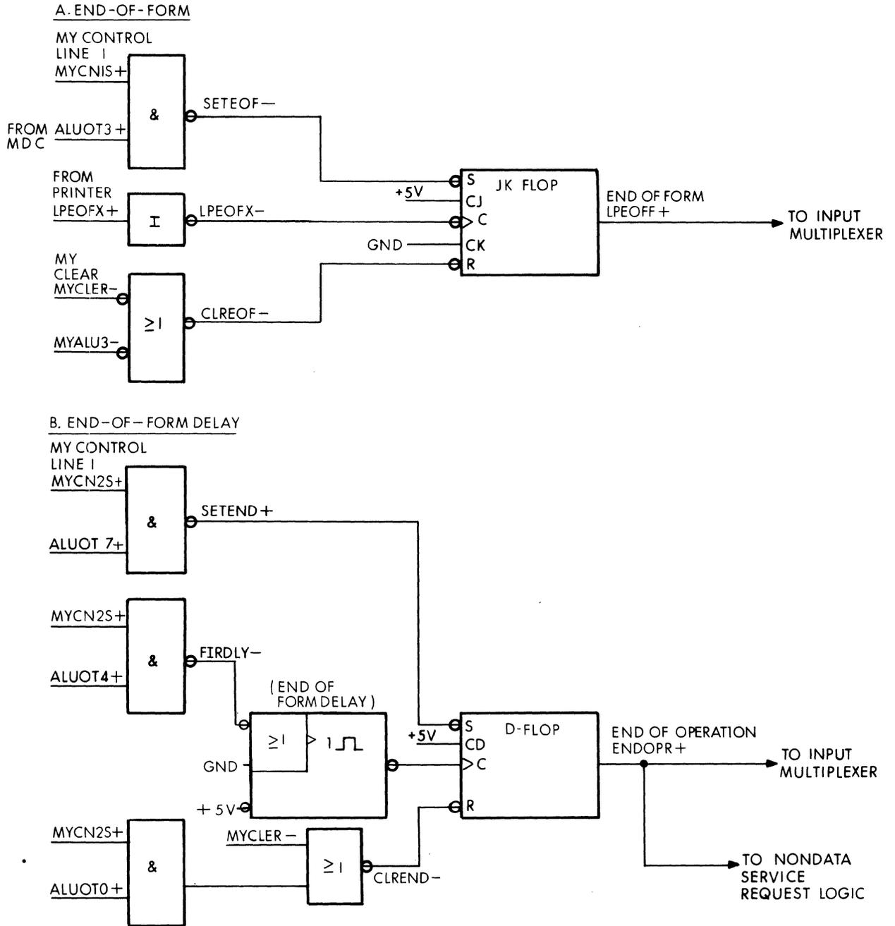
Figure 2-3 Control Logic (Sheet 1 of 2)
