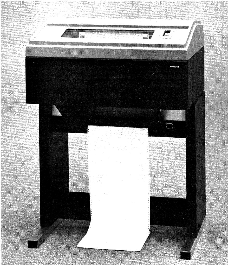
Figure 1-4 Line Printer
