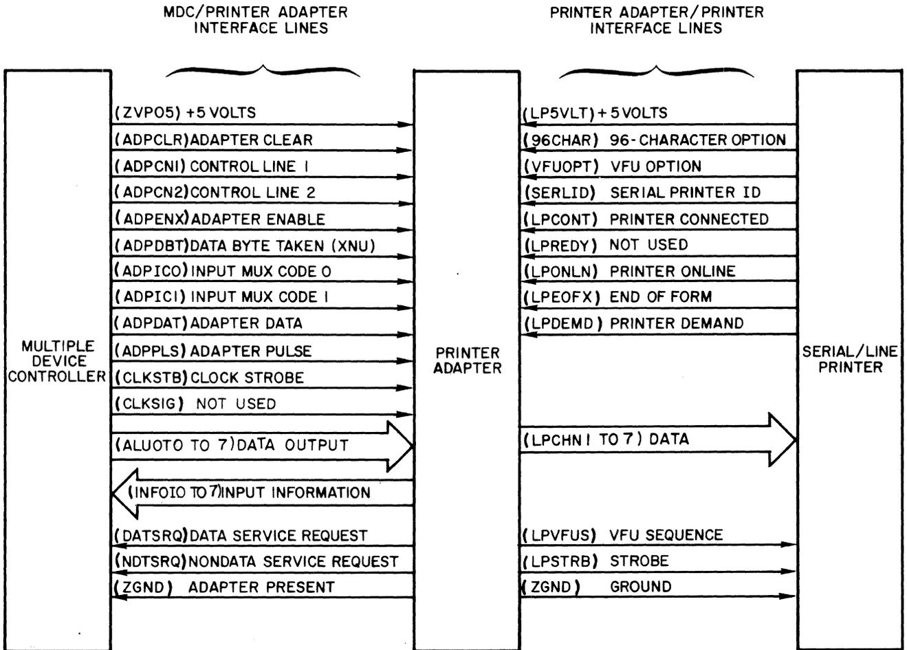
Figure 2-2 MDC/Adapter/Printer Interface
