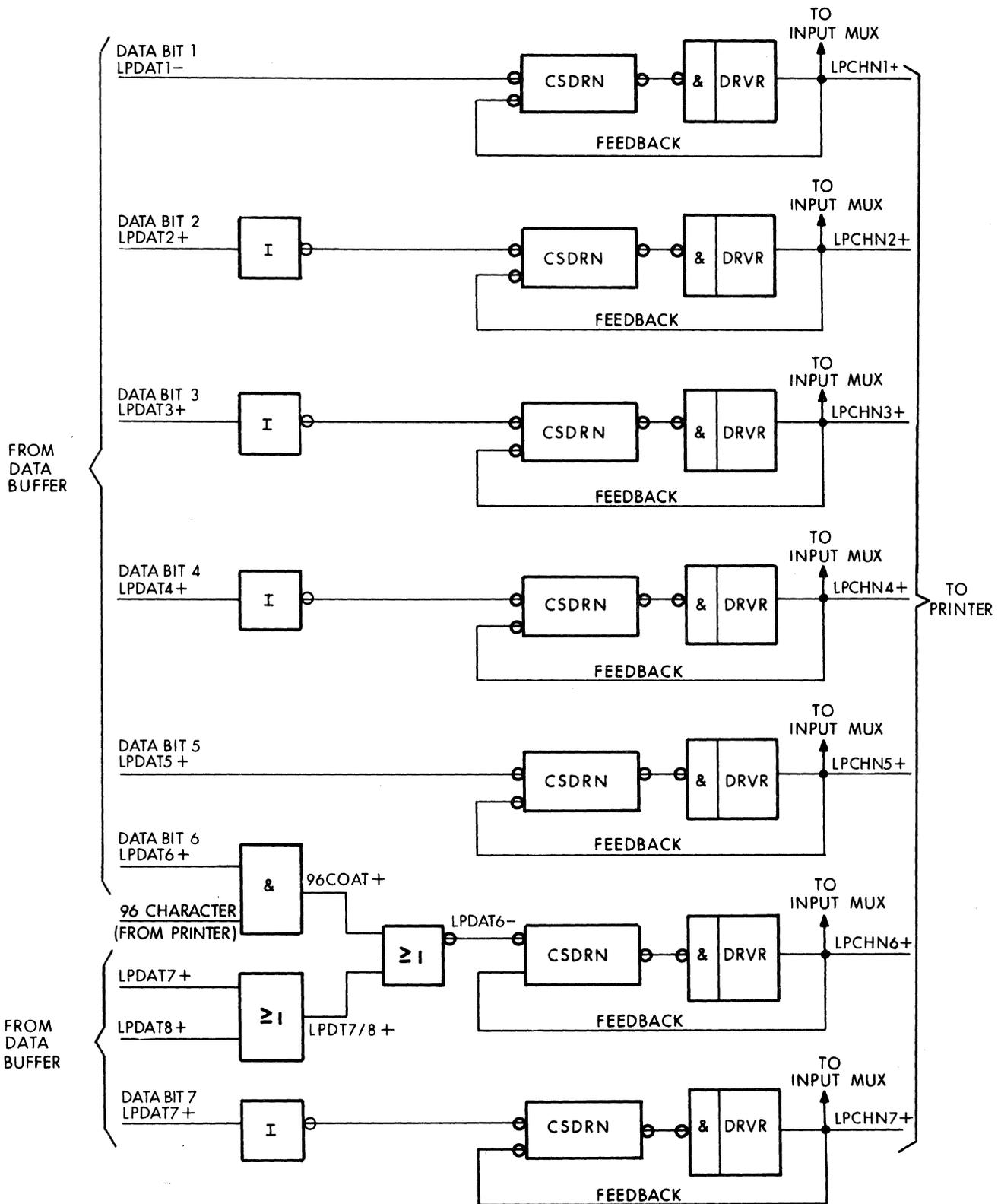
Figure 2-6 Line Driver Logic
