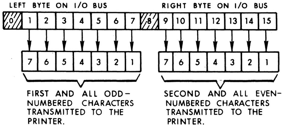
Figure 1-3 Data Transfer to Printer
