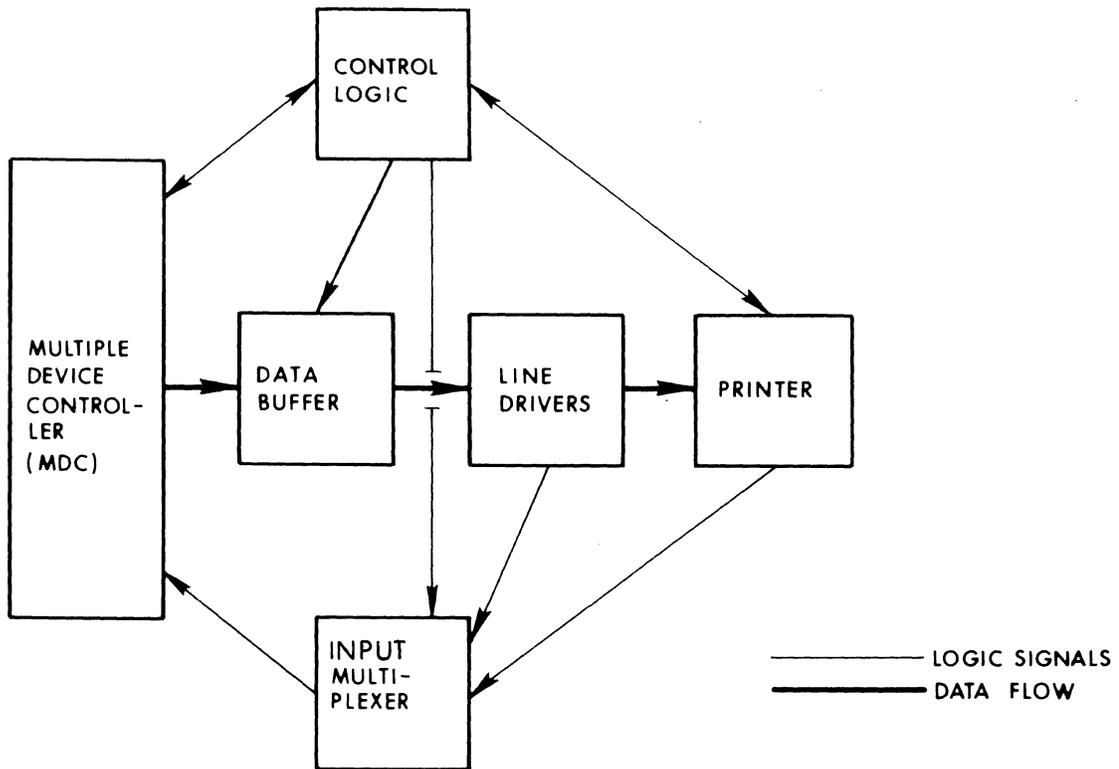
Figure 1-2 Data Flow Through Printer Adapter
