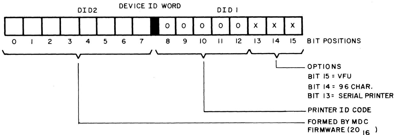
Figure 3-1 Device-Specific Word Bit Structures
