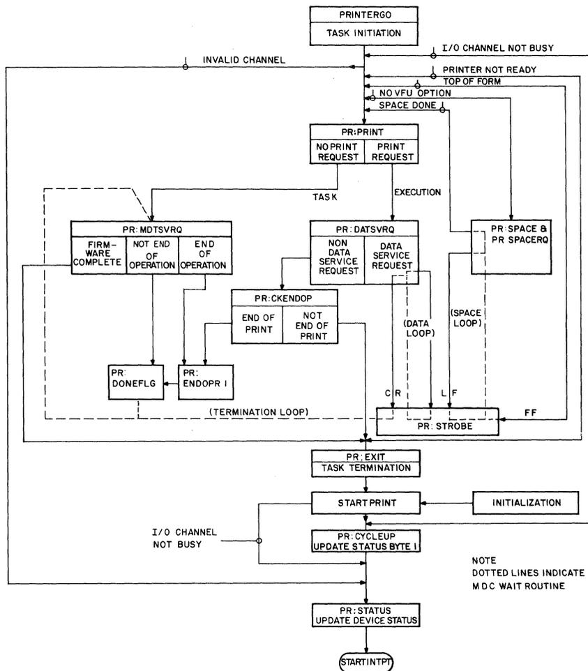
Figure 3-2 Functional Flow Chart for Printer Adapter Firmware
