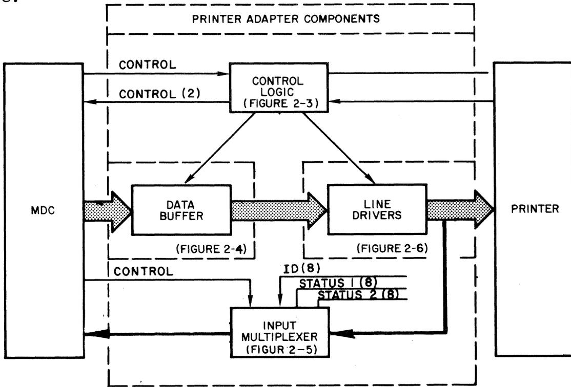
Figure 2-1 Printer Adapter, Major Block Diagram
