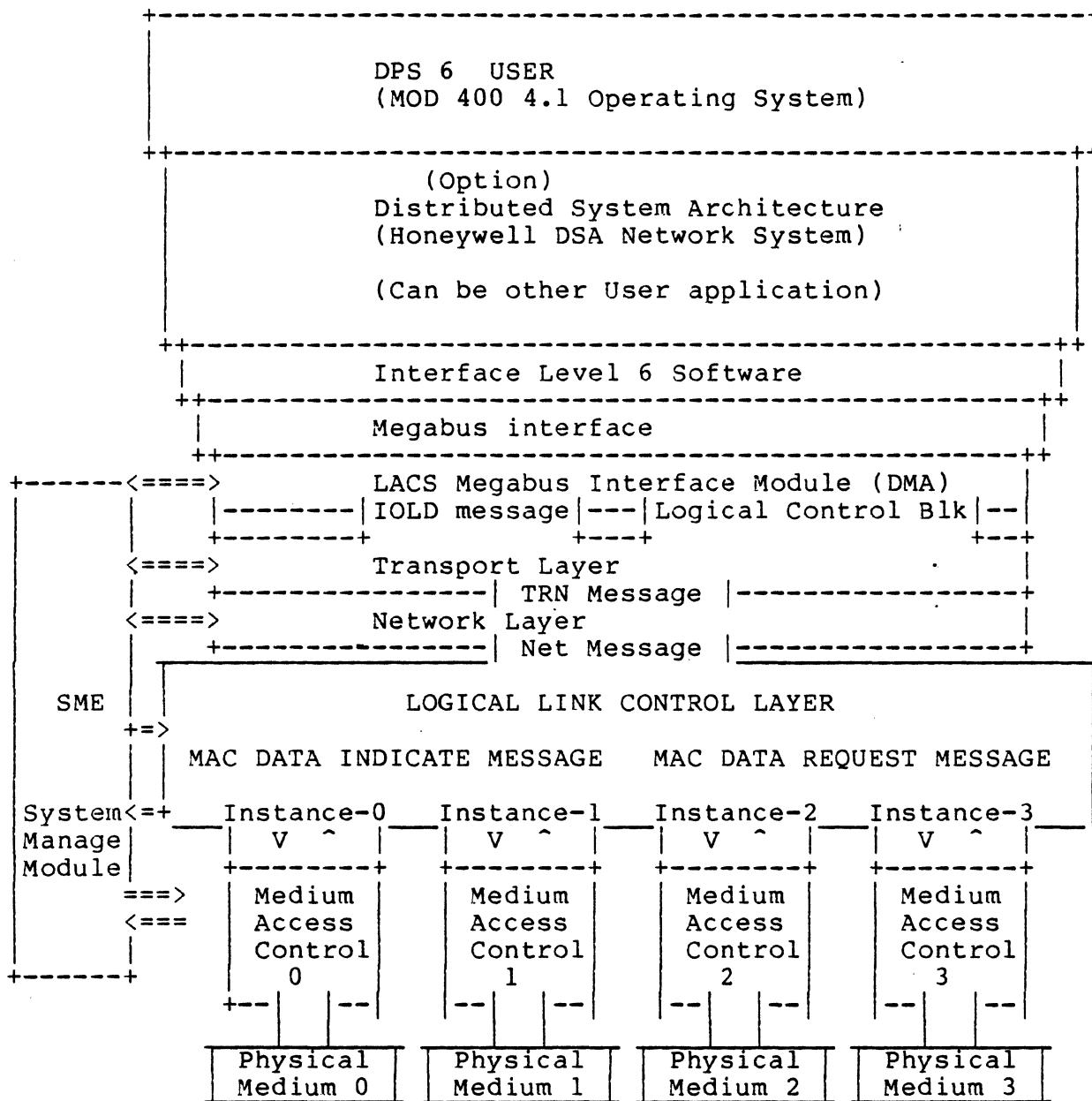
LOGICAL LINK CONTROL LAYER (IEEE 802.2, in LACS) Component Specification
