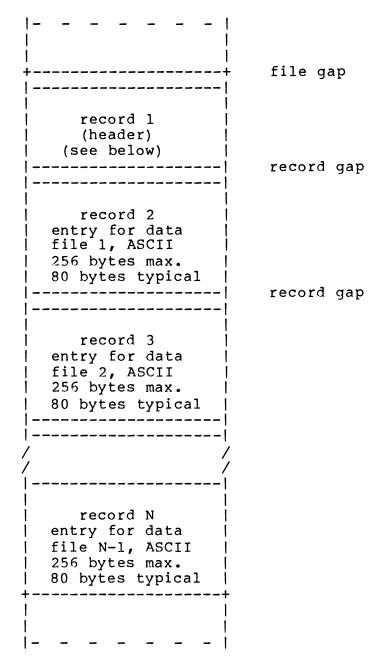
Record 1 is the Header record of ASCII 80 bytes. It contains the time of creation of the tape, the number of files on the tape, the total number of RTE blocks (128 words) in all the files, the record length in words for the packed data file records, and the reel number.
