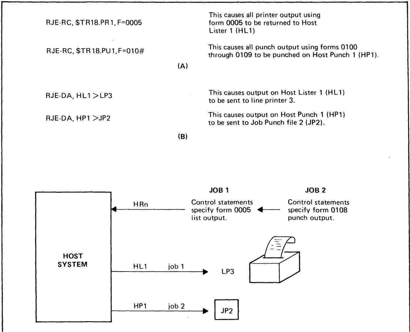
Figure 6-4. IBM-MRJE/WS Forms Assignment (Used to Route Output)
