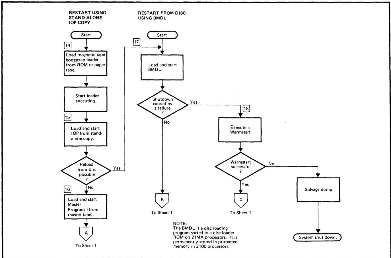
Figure 4-1. Operating Procedures Overview, Flow Diagram (Sheet 2 of 2)
