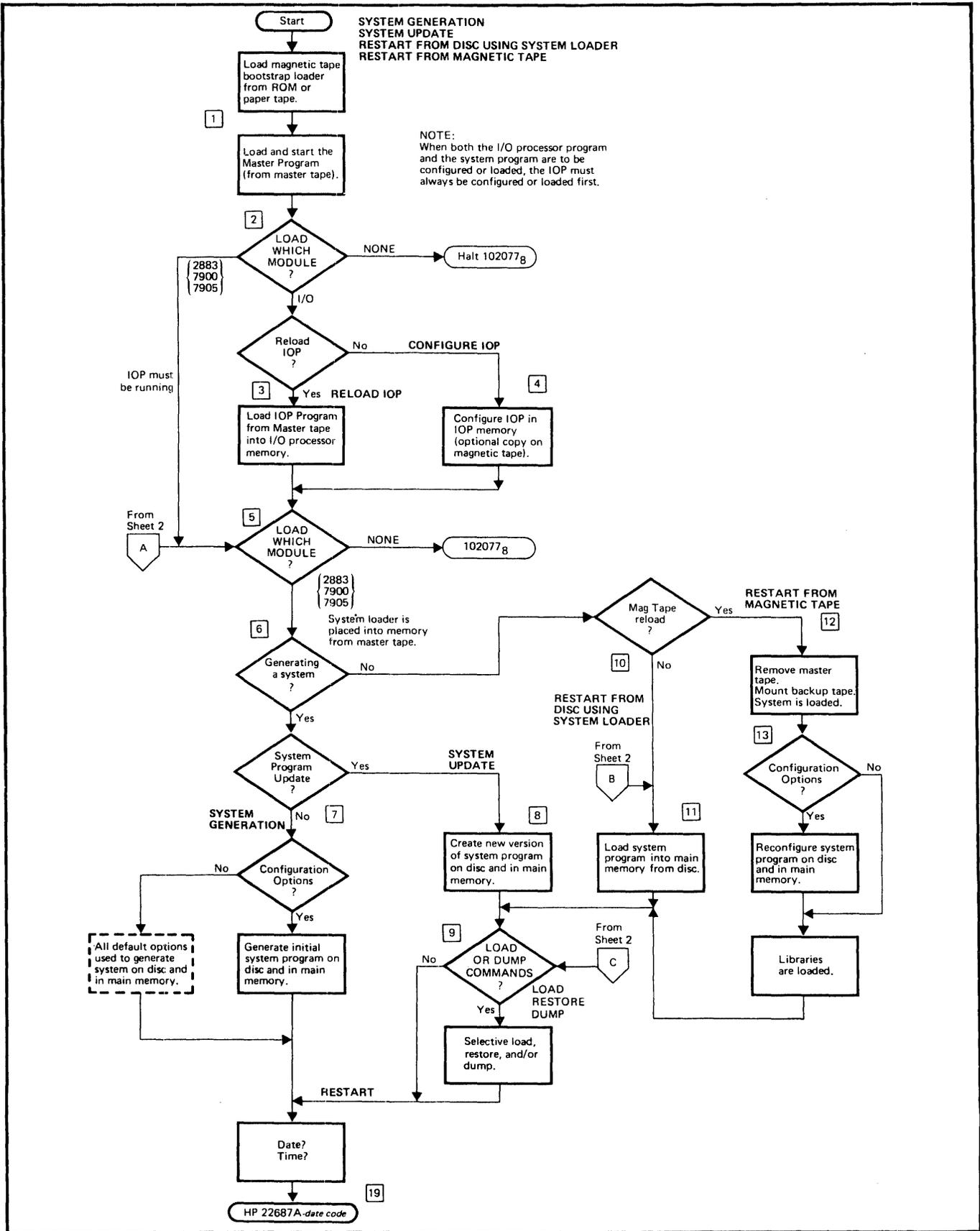
Figure 4-1. Operating Procedures Overview, Flow Diagram (Sheet 1 of 2)
