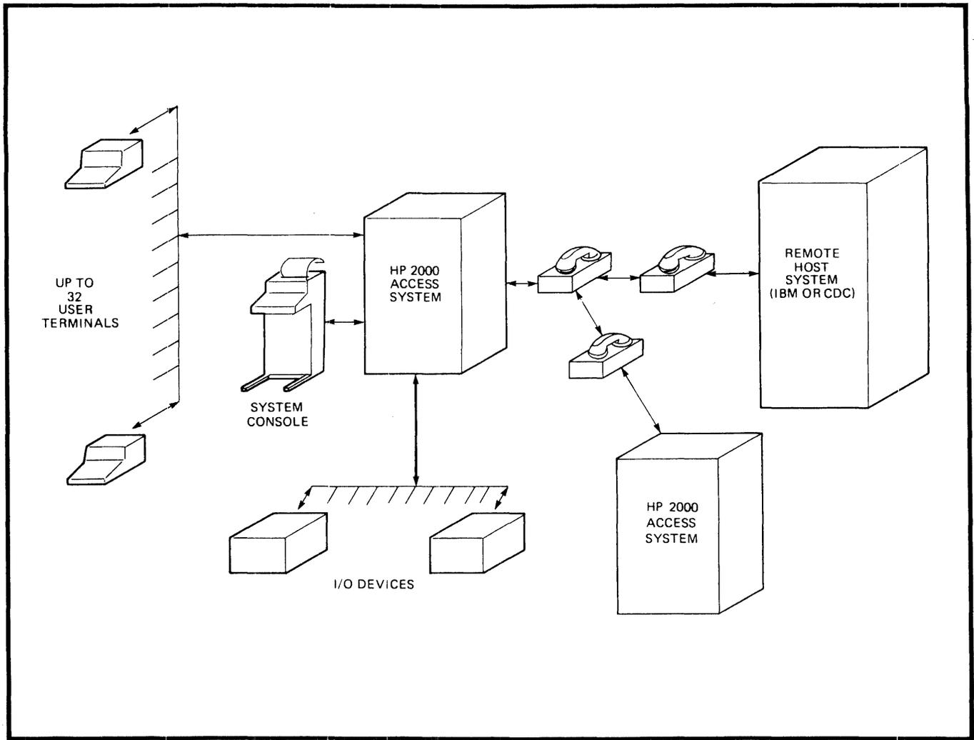
Figure 6-1. Elements of an HP 2000 Access Data Communications Facility
