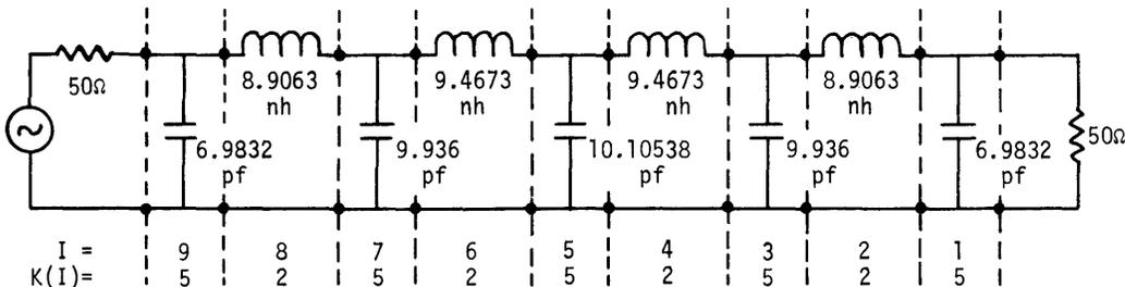
As shown the sub-circuits are numbered from the load toward the generator. The numbers K(I) are the catalog numbers, as found in the catalog section following the example. Each catalog entry shows the exact form of the line needed to input that circuit. Below is the complete input information for this example and the various printout options. Parenthetical explanations have been added later.
