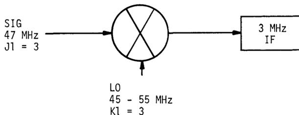
The spurious response readout is always referred to the lower edge of the receiver band. In this case, the signal is swept from 45 MHz to 55 MHz, so that the lower band edge is 45 MHz. Add this to line 776 in the program as shown and proceed as before:
