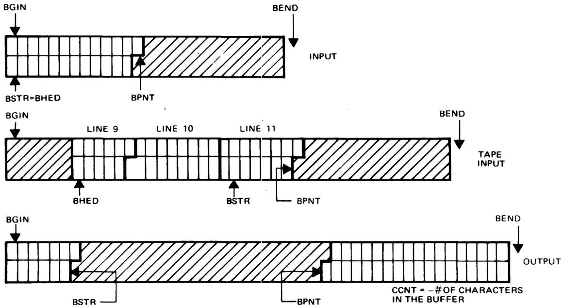
FIGURE 13. INPUT/OUTPUT BUFFERING
