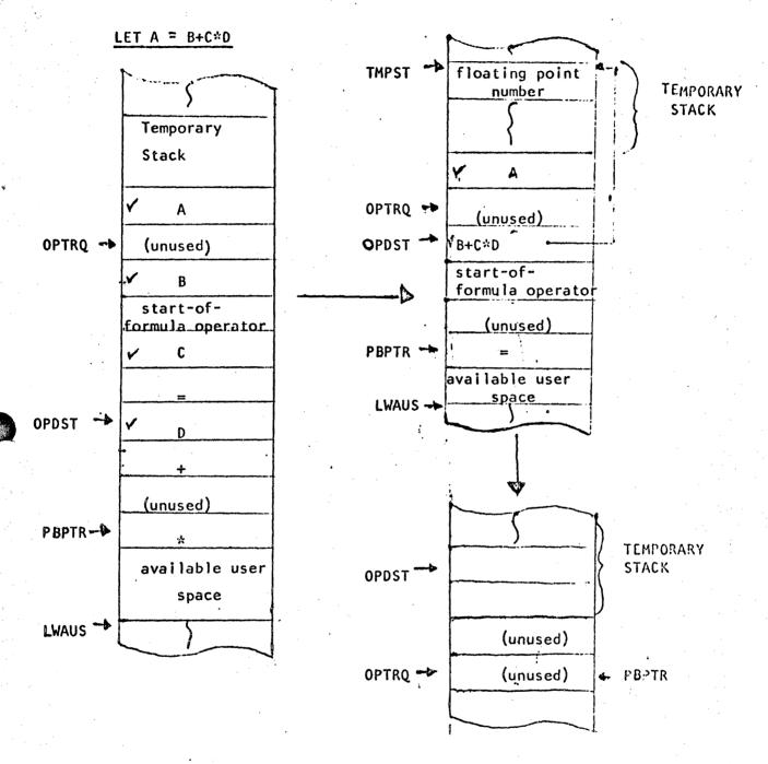
All operands (checked words) are addresses (i.e., C represents a pointer to the value of the simple variable C). Bits 7 - Ø of an operator entry contain the operators identifying code (See 'Basic Operations' Table) while bits 15-8 contain the operator's priority. Note the alternate-word structure of the stacks. The temporary stack holds intermediate values during the formula evaluation.
