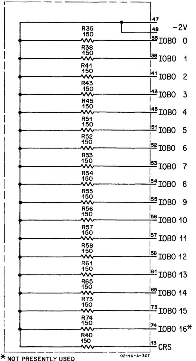
Figure 5-1. Resistance Load Card
