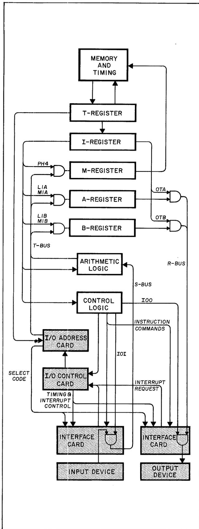
Figure 2-2. Block Diagram of System Input/Output Operations
