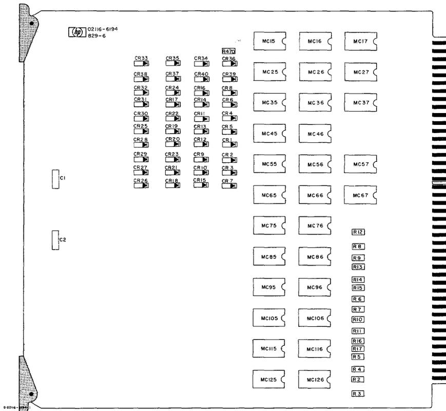
Figure 4-3. I/O Address Card, Component Location
