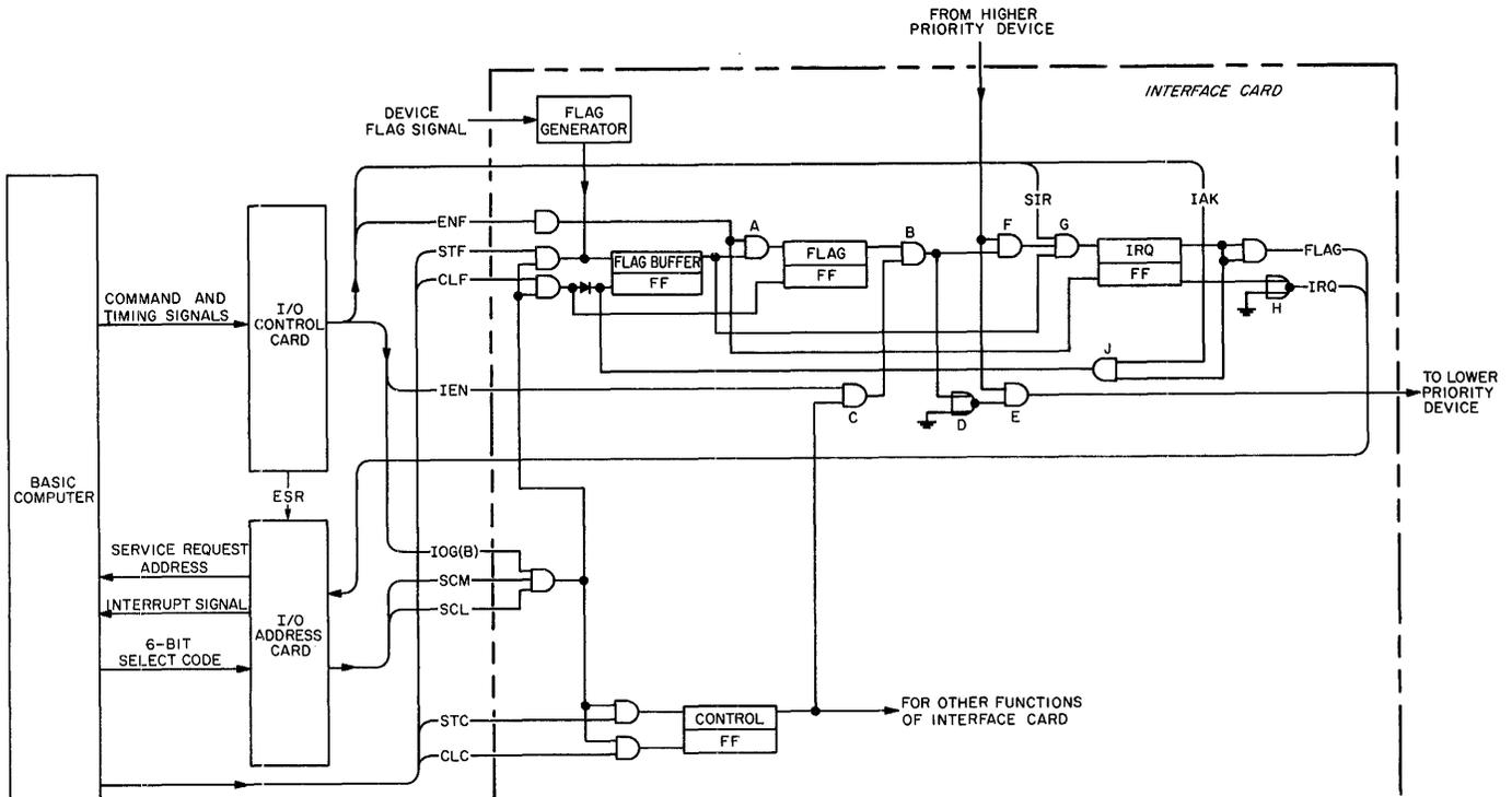
Figure 2-5. Typical Interrupt Logic
