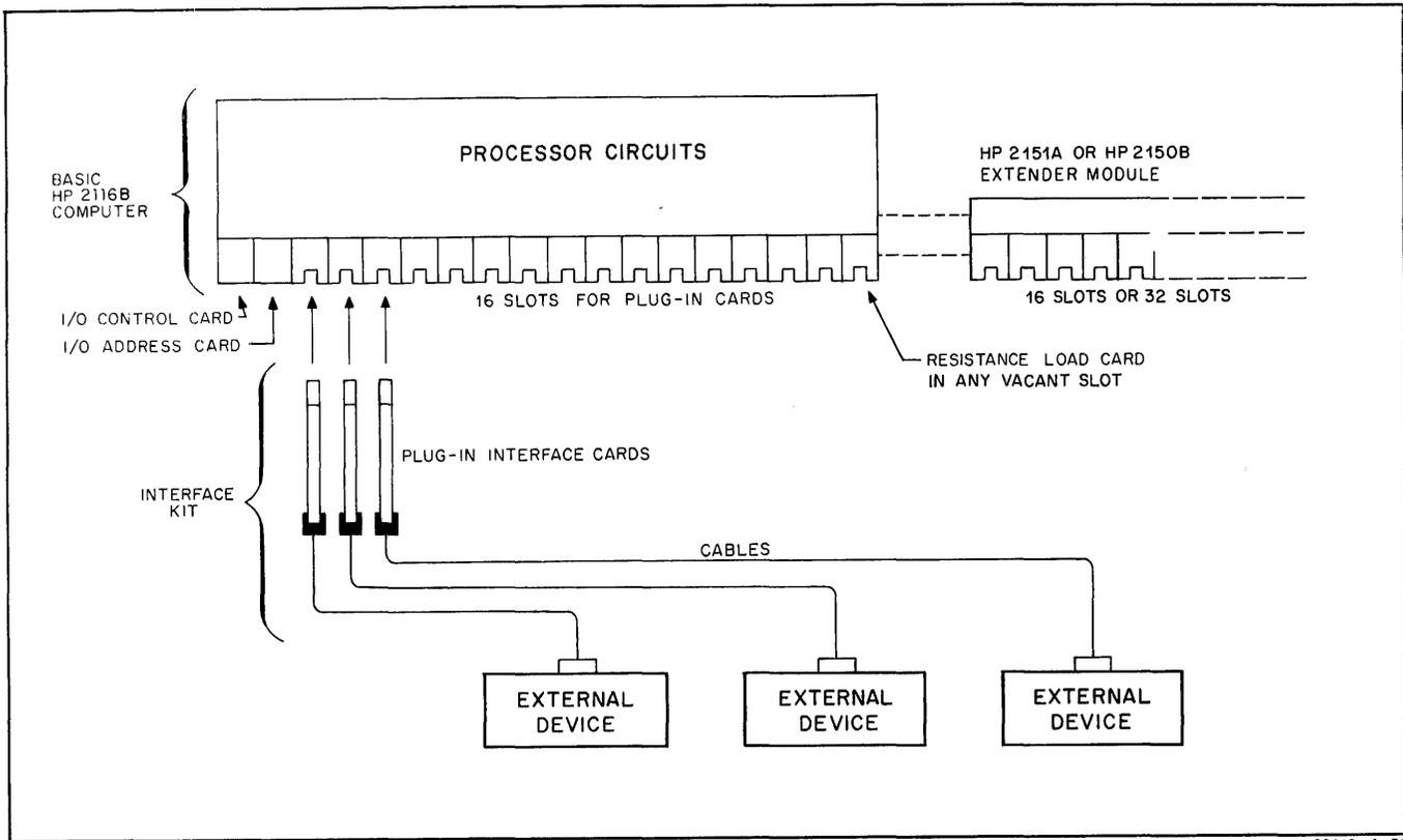
Figure 2-1. Input/Output Structure
