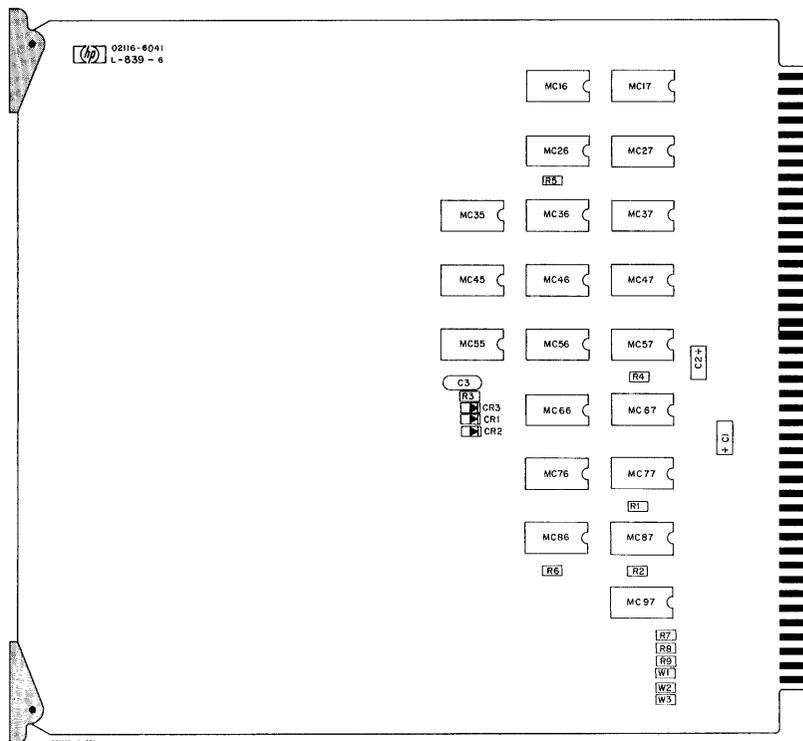
Figure 3-2. I/O Control Card, Component Location
