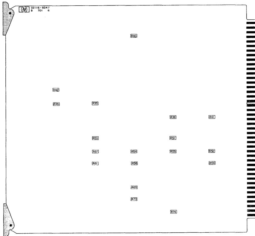
Figure 5-2. Resistance Load Card, Component Location
