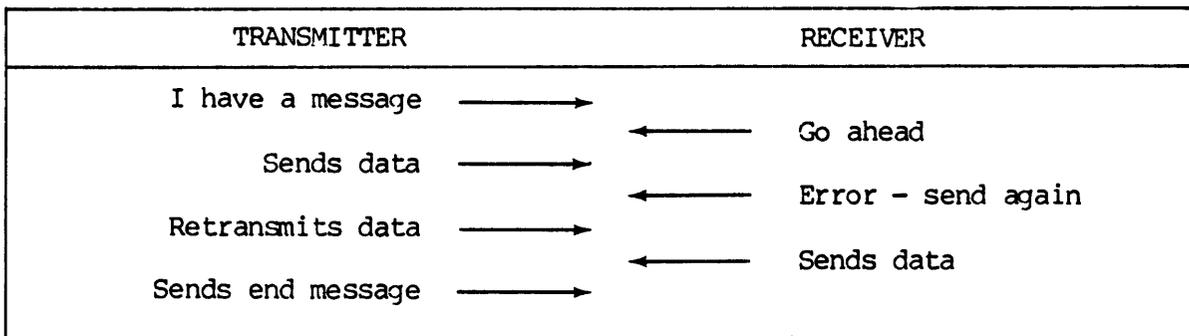
Figure 3-1. Simplified Handshaking Sequence
