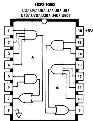
Figure 7-1. Integrated Circuit Base Diagrams (Continued)
