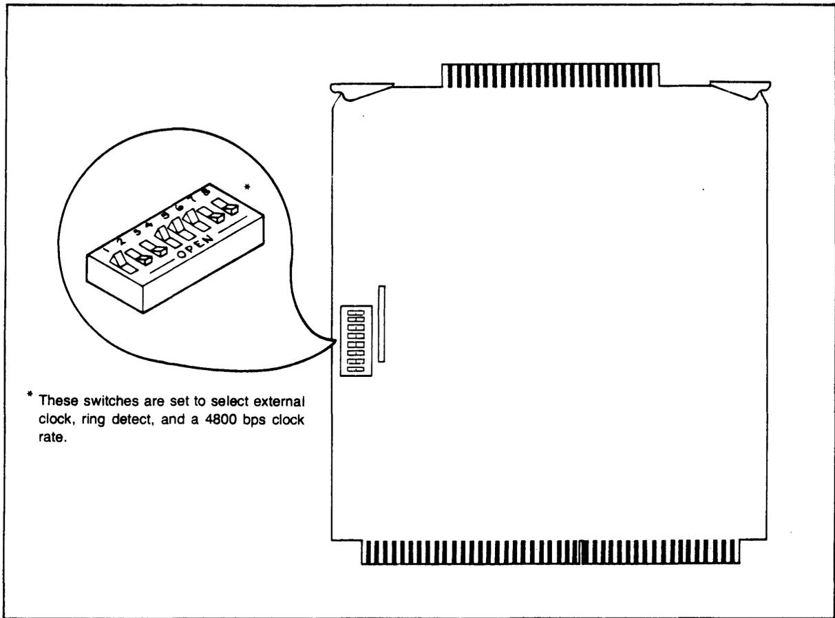
Figure 2-3. DIP Switch Position and Configuration
