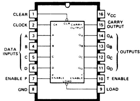
Figure 7-1. Integrated Circuit Base Diagrams (Continued)
