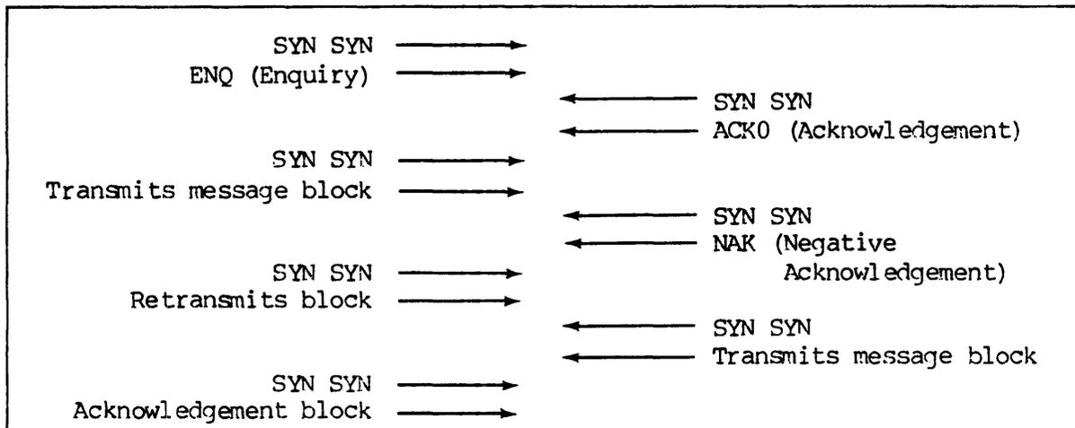
Figure 3-3. BISYNC Handshaking Sequence
