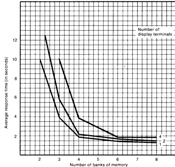
Response Time: Example 2 During Concurrent Processing with Example 1 and Standard Job
