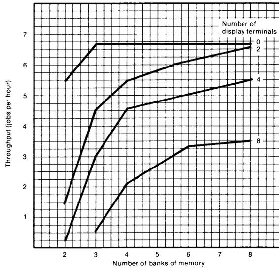
As the number of terminals (half of the terminals performing Example 1 and half performing Example 2) increases, the total throughput of the standard job, running at a lower priority, decreases as shown in the graph above. (Running two standard jobs concurrently with no terminals on an HP 300 with four banks of memory, increased throughput from 6.7 to 9.2 jobs per hour.)
