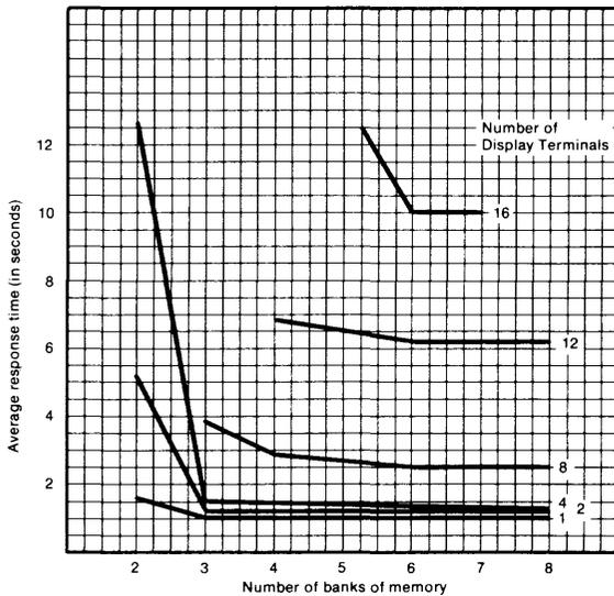
For these complex transactions, performance remained favorable up through eight terminals. (For example, the average response time for eight display terminals operating simultaneously on an HP 300 having three banks of memory was 4.0 seconds. Adding a fourth bank of memory reduced the response time to 2.8 seconds for Example 1.)
