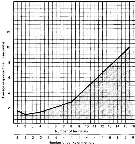
These results show that increasing memory size to three and four banks improves TEST performance, and that TEST speeds are dependent on program size.
