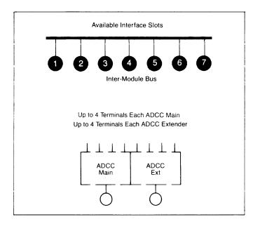
As a result, the options that have been chosen and the interface slots they occupy will be evident at a glance. DO NOT EXCEED THE TOTAL NUMBER OF AVAILABLE INTERFACE SLOTS ON THE INTER-MODULE BUS OR IOP BUS.
