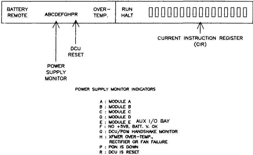
Figure 1-3. System Status and Display Panel (HP 32460B/32468B)
