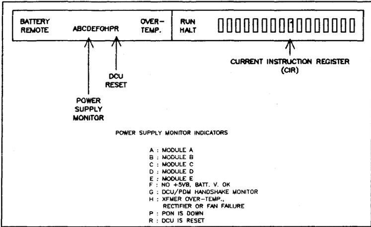
Figure 6-11. System Status Panel Display (SSPD-B)
