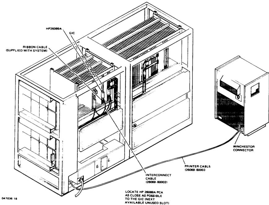
Figure 7-8. HP 2611A/13A/2617A/2619A Printer Installation
