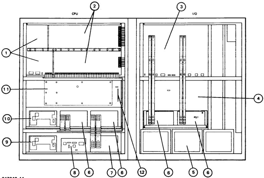
Figure 8-3. CPU and I/O Card Cages Series 64/68 (HP 32460A)
