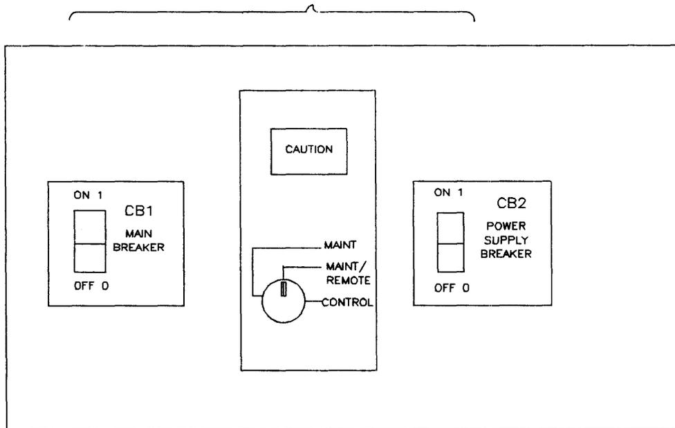
Figure 1-4. Power Control Module (32460A)
