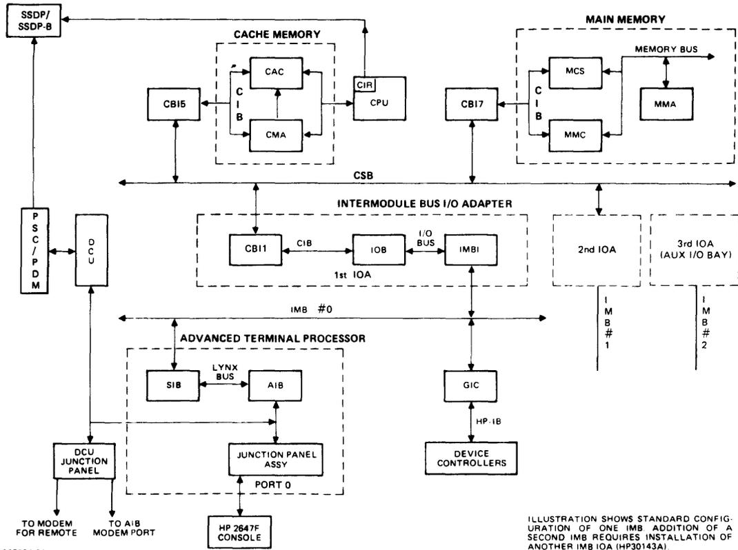
Figure 1-1. HP 3000 Series 64/68 Functional Block Diagram
