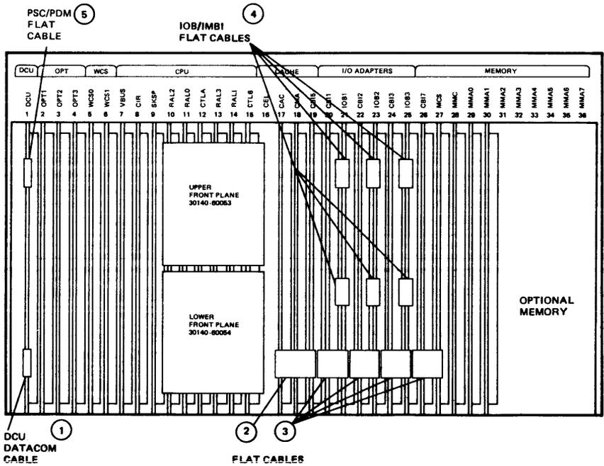
Figure 8-5. CPU Card Cage and Cabling Series 64/68
