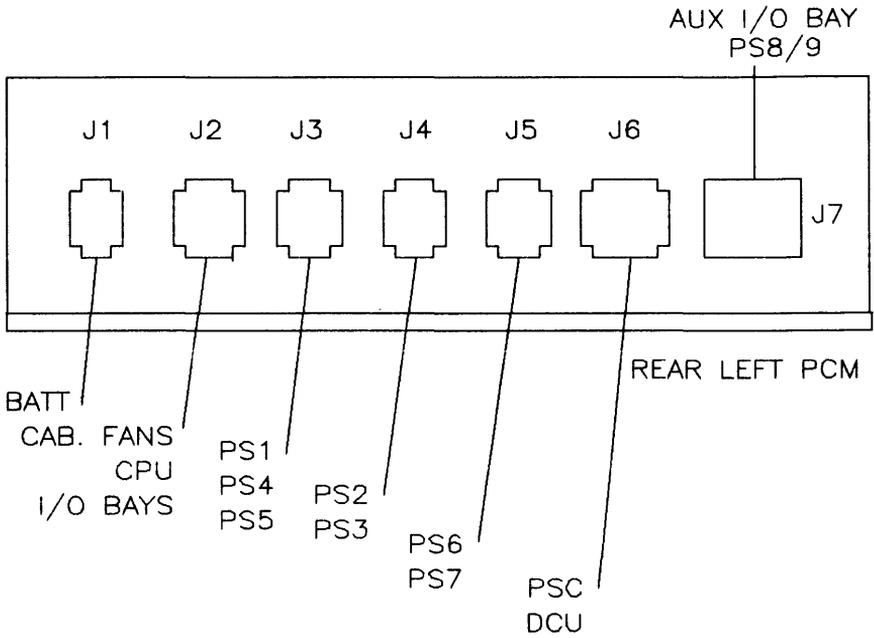
Figure 1-5. PCM Cable Connections (HP 32460A)
