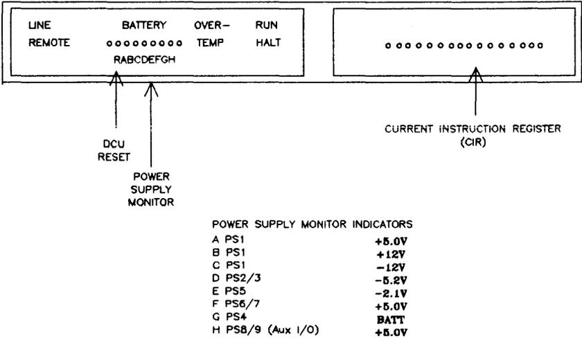
Figure 1-2. System Status and Display Panel (HP 32460A)
