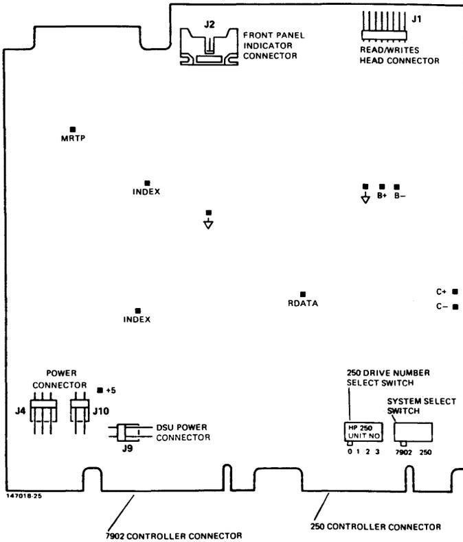
Figure 7-3. HP 9895A Drive Electronics PCA
