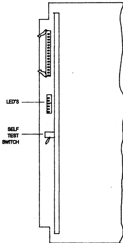
Figure 5-1. DCU Selftest Control & Indicators
