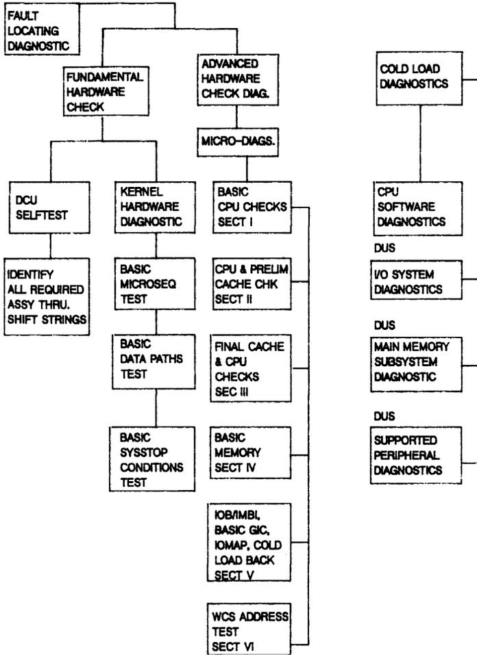
Figure 5-3. Fault Locating Diagnostic Block Diagram
