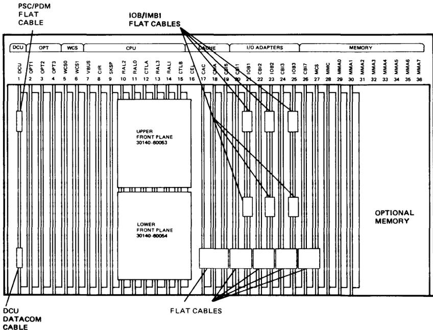
Figure 3-1. CPU Cage and Cabling Assignment
