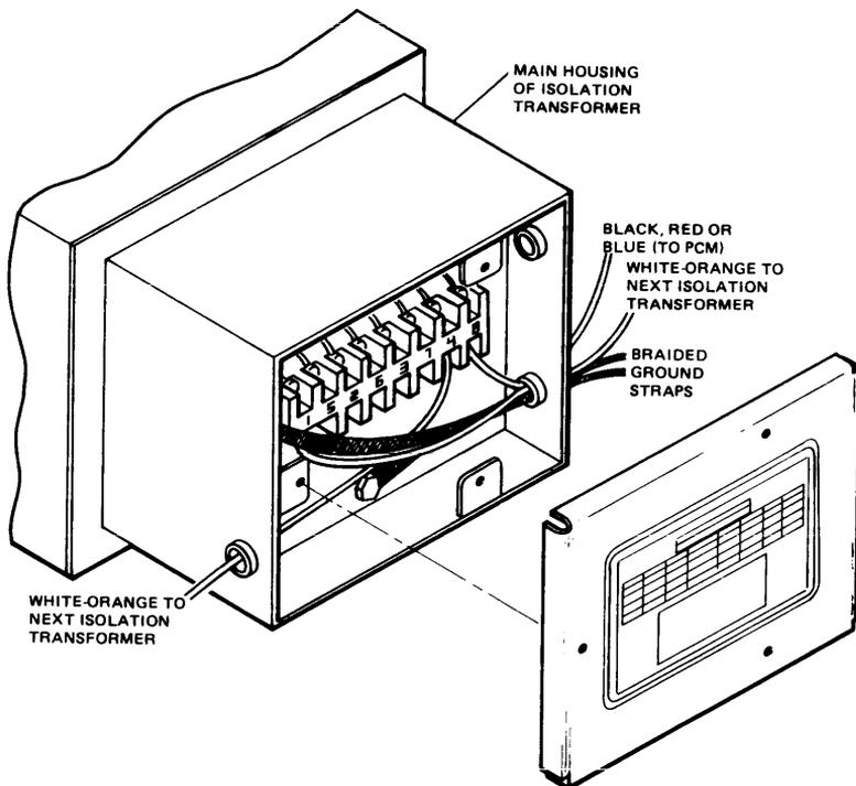
Figure 6-1. Transformer Strapping
