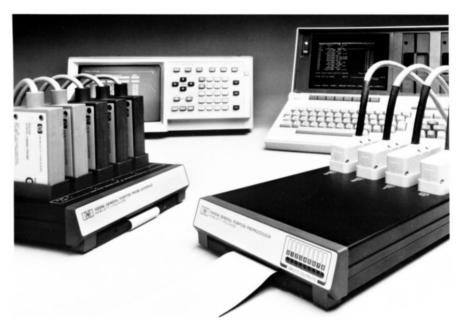
Inverse assembly software translates microprocessor code into the processor mnemonics to generate disassembled trace listings. For the 64000 System, the software is provided on flexible disc with each microprocessor-specific interface. The appropriate inverse assembler for the HP 10269A Probe Interface is included with the interface option, and is stored on a minicassette that is used with the HP 82161A Digital Cassette Drive.
