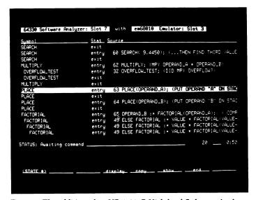
**Figure 5.** The addition of an HP 64334B High-level Software Analyzer provides source code level debugging.
