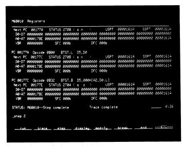
**Figure 4.** Register displays are labeled for easy interpretation of all registers and status bits.
