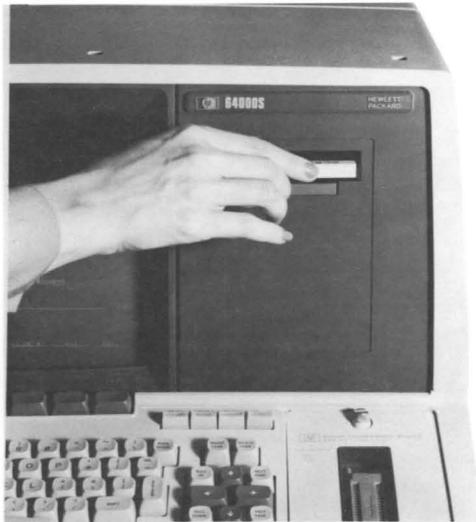
**Figure 2-29. System Tape Installation**
