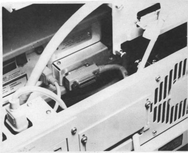
Figure 2-34. 13037 Disc Controller Rear Panel
