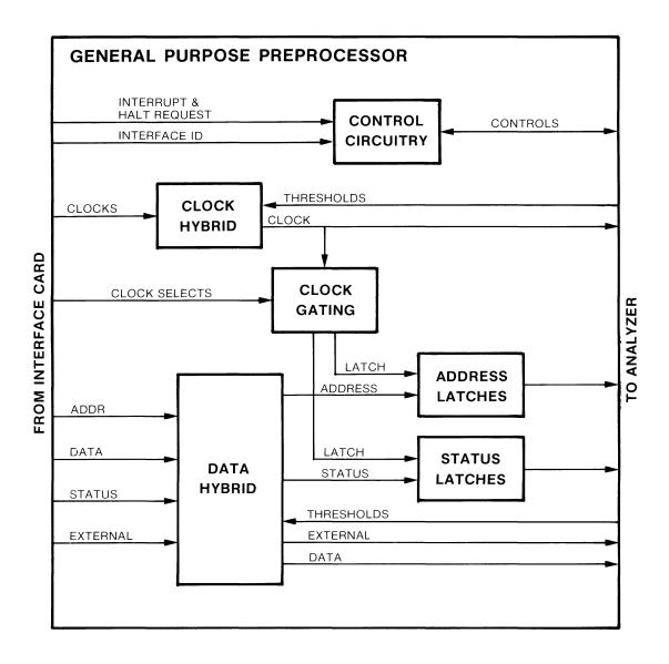
Figure 4-1. Preprocessor Block Diagram
