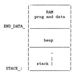
The transfer address will have been set by the linker so that simply loading the absolute file, and stepping or running the program is all that is required. Note that program execution does not start at address 0000H if the program contains local procedures or functions. However, the cprogram name identifier in the program heading is a global symbol and the label of the program transfer address. This program may be executed within emulations by the command:
