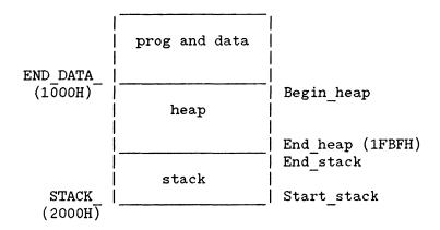
Six bytes are used each time the heap is initialized or marked. When an item of four bytes or less is to be allocated, four bytes will be removed from the free list even if less is needed. Likewise, when an item of four or less bytes in size is deallocated, four bytes will be returned to the free list.
