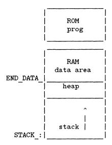
For a program that is designed to run completely in random access memory (RAM), the memory mapping should look like the following:
