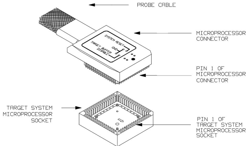
**Figure 3-2. Installing into a 70136 PLCC type socket**
