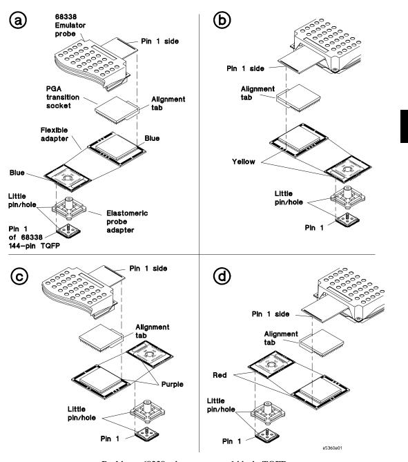
Probing a 68338 microprocessor 144-pin TQFP
