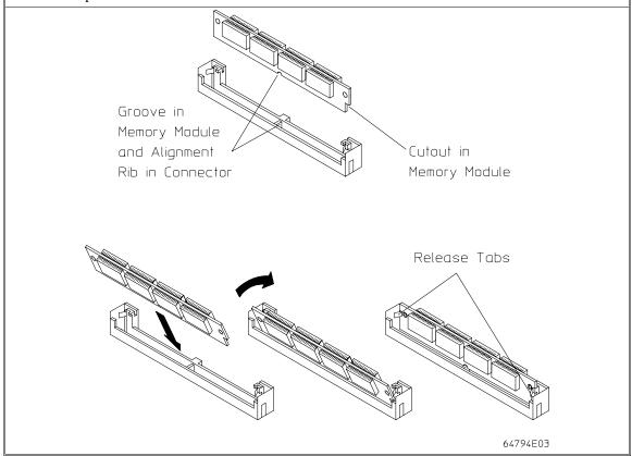
Chapter 1: Preparing the Emulator **Step 4. Install emulation memory modules on emulator probe**
