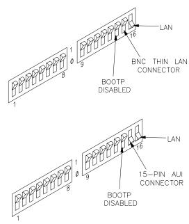
Switch 16 must be set to one (1) indicating that a LAN connection is being made.
