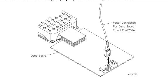
3 If you have not already done so, connect the +5 V power cable to the connector in the HP 64700 front panel. See page 19.
