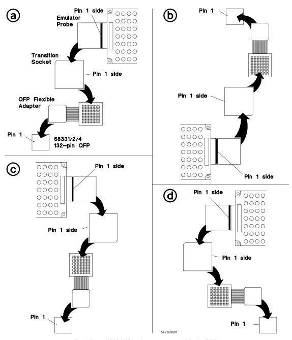
Probing a 68331/2/4 microprocessor 132-pin QFP
