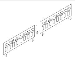
Note that switch settings are read during the power up routine of the HP 64700 card cage. Any changes made to the switches after power-up will not be read until you turn the HP 64700 off and back on again.
