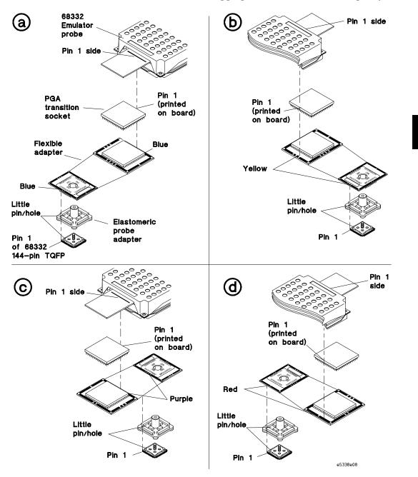
Probing a 68332 microprocessor 144-pin TQFP
