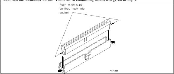
**3** Connect the other ends of the cables to the emulator probe. Make sure the stainless steel clips on the cable connectors are properly latched within the sockets.
