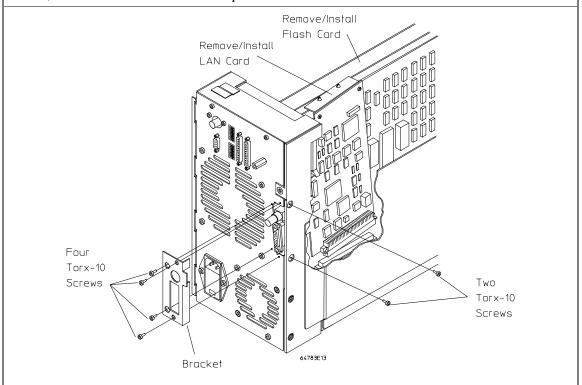
**14** This step applies only to the HP 64700A. If you wish to install the flash card (used for updating firmware, see chapter 5), refer to the diagram above. Install the flash card in any available slot between the 80-channel analyzer card and the HP 64748C control card in the cardcage. Insert the flash card in the plastic guides. Make sure the connectors are properly aligned. Then press the card into the mother board sockets. Make sure the card is seated all the way into the sockets.
