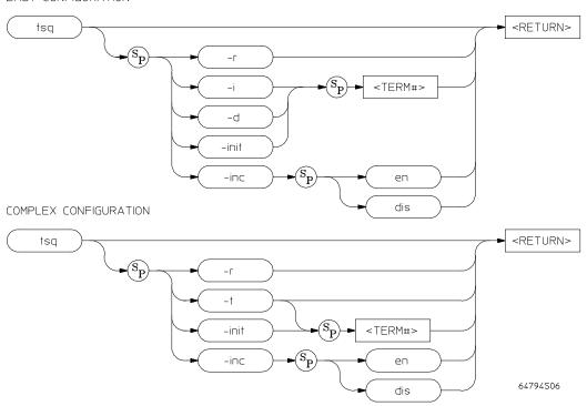
The **tsq** command allows you to manipulate or display the trace sequencer. Note: the **tif** and **telif** commands are used to define each sequencer state specification.
