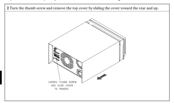
Chapter 6: Installation and Service Step 2. Install the deep analyzer card in the HP 64700A card cage
