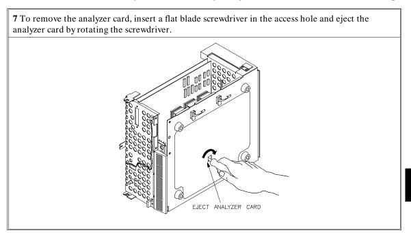
Do not remove the system control card. This card is used in all HP 64700 emulation and analysis systems.
