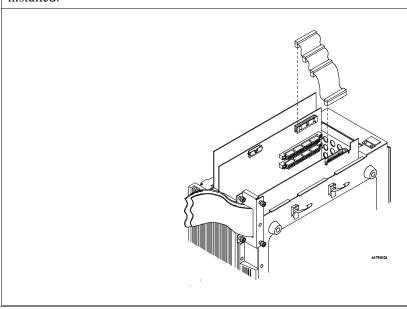
Chapter 6: Installation and Service Step 2. Install the deep analyzer card in the HP 64700A card cage
