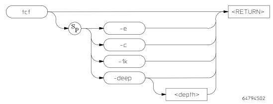
The **tcf** command is used to set the configuration for the emulation-bus analyzer.
