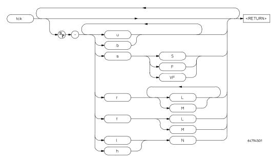
The **tck** (trace clock) command allows specification of clock qualifiers and clock edges for the master clocks used by the deep analyzer. The **tck** command also allows specification of maximum clock speed; the clock speed specifications are only included for compatibility with the 1K analyzer. Clock speed has no effect in the deep analyzer.
