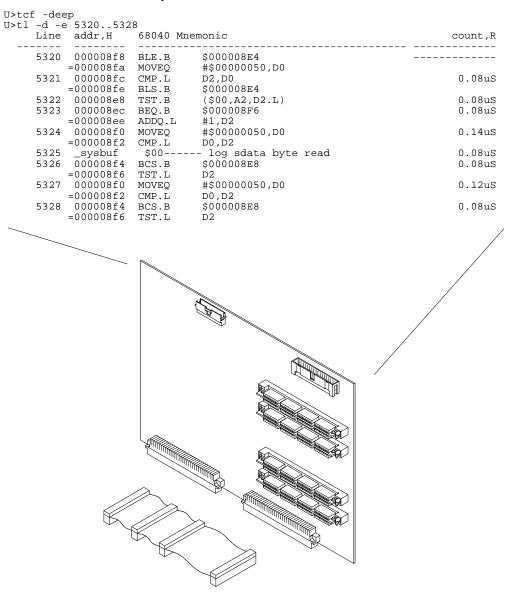
This chapter describes the HP 64794 Emulation-Bus Analyzer with deep trace memory, and lists differences between it and the HP 64703, HP 64704, and HP 64706 Emulation-Bus Analyzers with 1K trace memories it is designed to replace.
