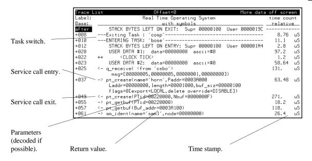
Note that there are entry and exit arrows on the left of the screen to show when a service call is entered and, on a separate line, to show when a service call is exited. This is important since an OS service call may switch to another task while in the OS and NOT return to the calling service call for a long time, if ever.
