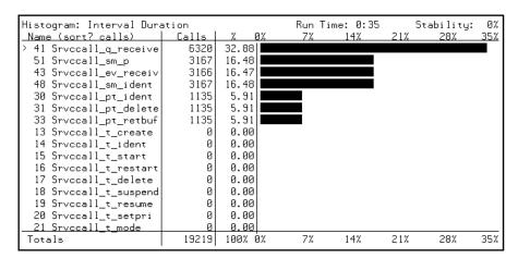
This displays a histogram of the number of times each service call is invoked from a single task.
