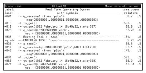
Notice that the time stamp on the right hand side of the screen gives a useful indication of the time between task exit and the next entry into this same task. In this example, the elapsed time was 5.73 milliseconds.
