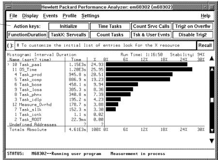
is called can be displayed, providing valuable information on system "thrashing". Also, the number of times each OS service call is invoked from your application can be tracked, helping to isolate bottlenecks from over-utilized system features.
