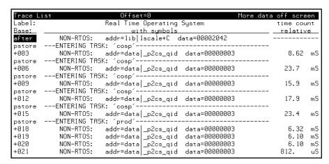
All tasks that access a specific variable can be tracked with this measurement.
