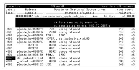
This measurement allows you to see when a specific variable is accessed by a specific task and the source code context under which the variable is accessed.
