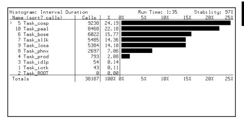
The histogram shows the the number of times each task is entered (and exited). This can be very useful for detecting system "thrashing" between tasks.
