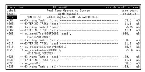
The command above traces only events and task switches so you can see what tasks use events and how they effect system flow.
