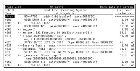
This action key is used so that service calls, task switches, clock ticks, stack activity, and user-defined events are all tracked and displayed in the trace.
