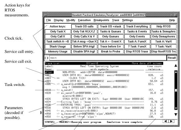
RTOS measurements are easy to set up and use. To set up a measurement you simply point and click on the appropriate action key (which runs a command file), and the setup is done automatically. If parameters are required, you are prompted for them. In the graphical interface, these prompts appear as dialog boxes in which you can either type or cut-and-paste the required parameters.
