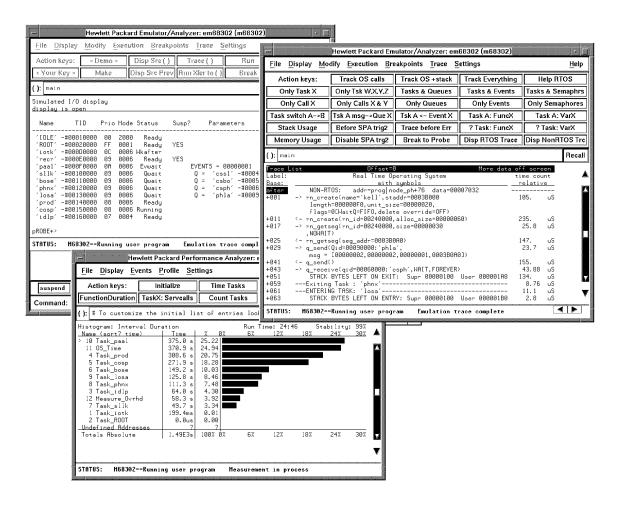
The RTOS Measurement Tool is a collection of files that are used with your real-time OS application and the HP 64700 emulation/analysis system to view program execution in the context of the real-time OS. For example, you can view service calls and their parameters, task switches, clock ticks, and dynamic memory usage.
