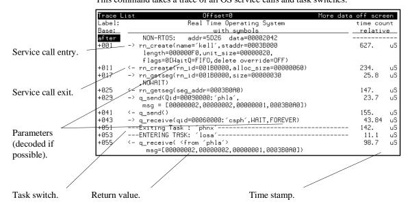
Note that there are entry and exit arrows on the left of the screen to show when a service call is entered and, on a separate line, to show when a service call is exited. This is important since an OS service call may switch to another task while in the OS and *not* return to the calling service call for a long time, if ever.
