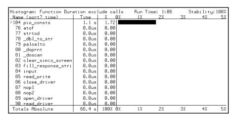
This performs a normal function duration profile measurement.
