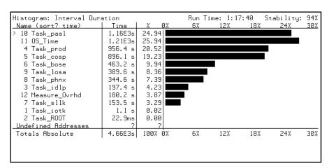
You see that the task names are listed in SPA, and a histogram showing the amount of time each task is taking is being displayed. This is very useful for detecting system bottlenecks.
