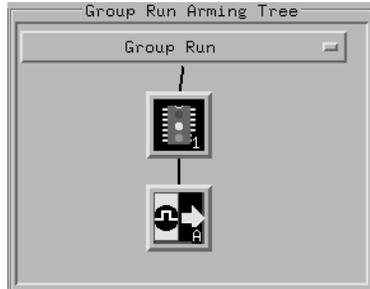
Clicking the **Group Run** button (at the very top of the Intermodule window or a logic analyzer window) will start the analyzer running. The analyzer will then wait for an arm signal. Now when the emulation module transitions into “Monitor” from “Running” (or from “Reset”), it will send the arm signal to the analyzer. If the emulation module is “In Monitor” when you click **Group Run**, you will then have to go to the emulation module or your debugger interface and manually start it running.
