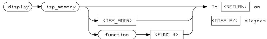
**Function** `display isp_memory` can display the contents of the ISP microprogram memory in mnemonic format. You can specify a function number to display instructions of an ISP function.
