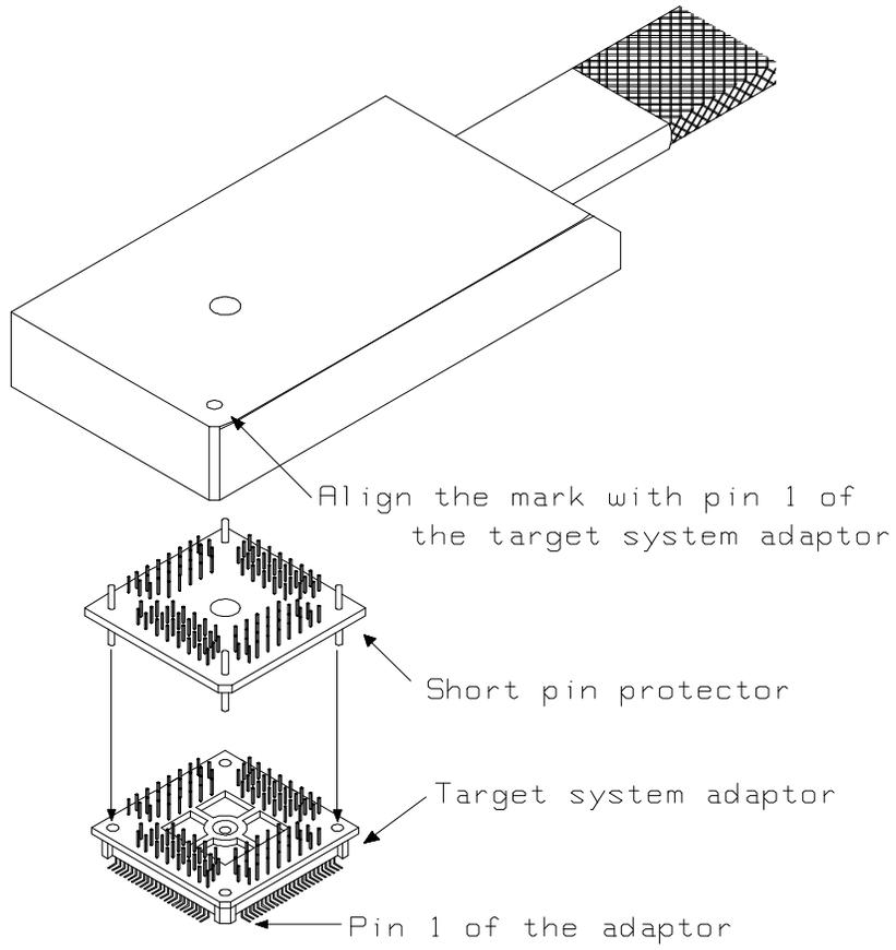
**Figure 3-1. Installing Probe into the Target System**
