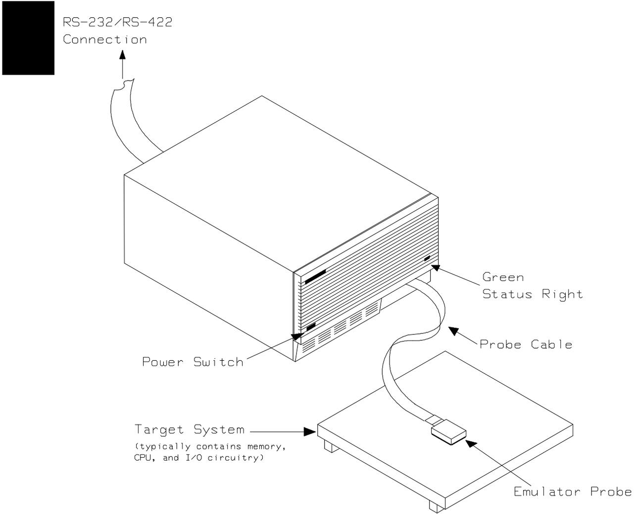
**Figure 1-1. HP 64732 Emulator for the H8/510 Processor**
