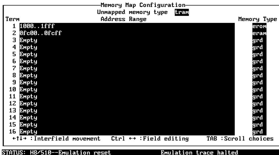
Use the TAB and Shift-TAB keys to pick memory type for mapped range.
