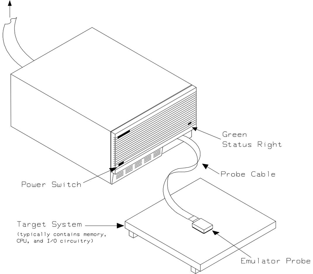
**Figure 1-1. HP 64739 Emulator for the H8/536 Processor**
