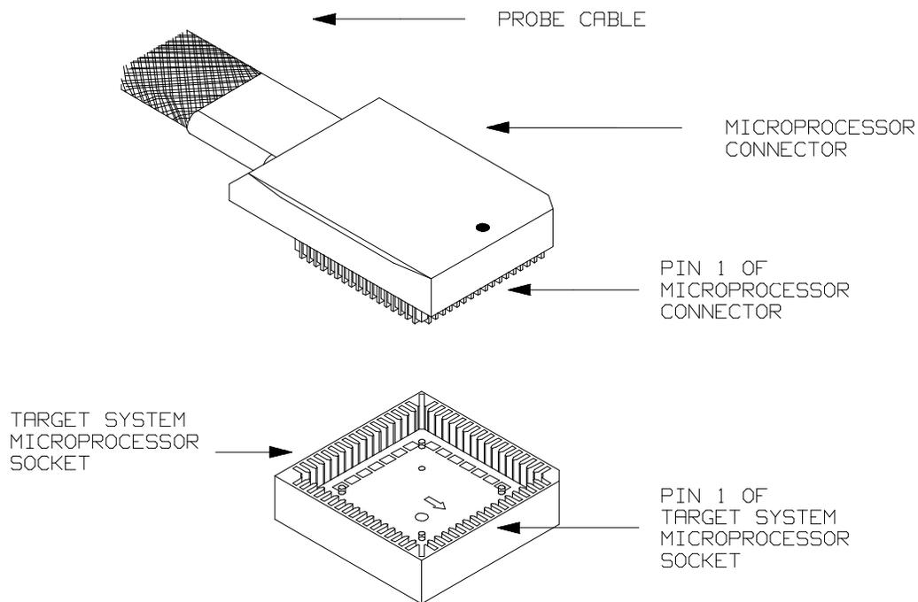
**Figure 3-8. Installing into a PLCC type socket**
