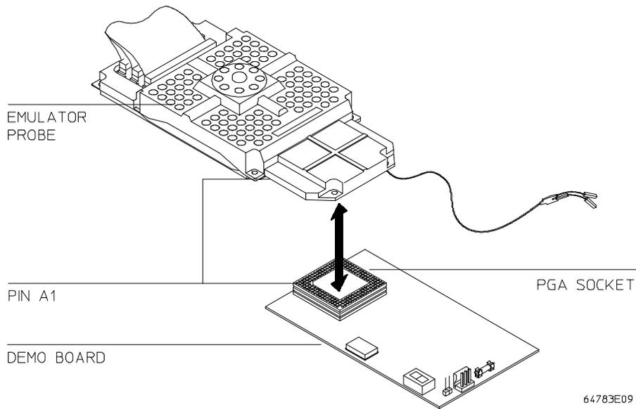
**2** Connect the power supply wires from the emulator to the demo target system. The 3-wire cable has one power wire and two ground wires. **When attaching the 3-wire cable to the demo target system, make sure the connector is aligned properly so that all three pins are connected.**
