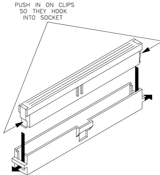
**3** Connect the other ends of the cables to the emulator probe. Again, make sure the stainless steel clips on the cable connectors are properly latched within the sockets, as shown in step 2.
