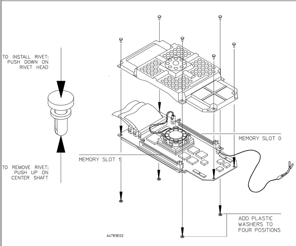
**2** Determine the placement of the emulation memory modules. Three types of modules may be installed: 256 Kbyte (HP 64172A), 1 Mbyte (HP 64172B), and 4 Mbyte (HP 64173A). Any of the emulation memory modules can be installed in either memory slot on the probe. Do not use HP 64171A/B modules; they are too slow.
