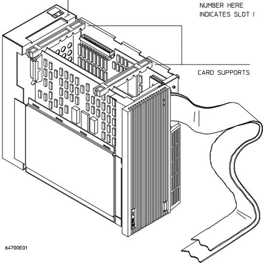
**15** To install the side cover, insert the side cover into the tab slots and fasten the two latches.
