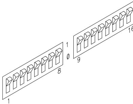
Note that switch settings are read as part of the HP 64700 power-up procedure. Any changes made to the switches after power-up will not be read until you turn the HP 64700 off and back on again.
