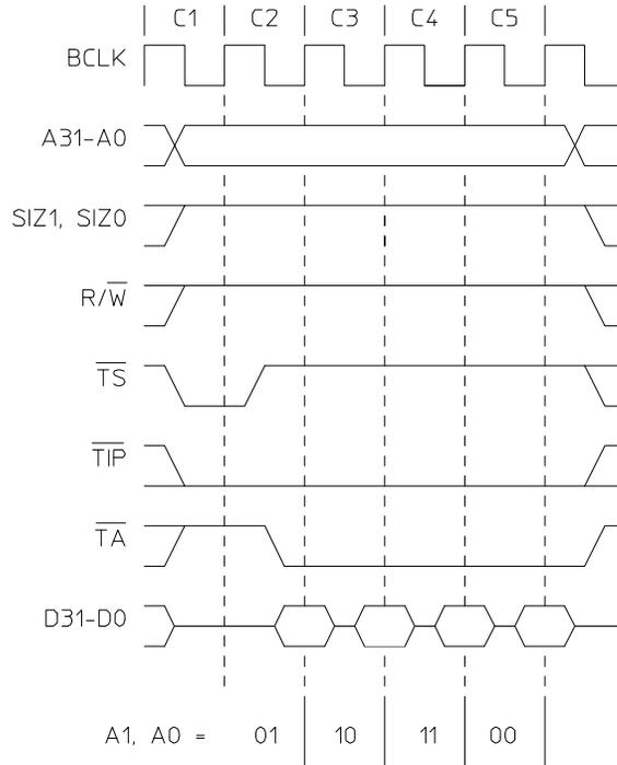
Note: The selected device increments the value of A3 and A2.
