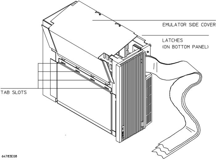
**16** Install the top cover in reverse order of its removal, but make sure that the side panels of the top cover are attached to the side clips on the frame.
