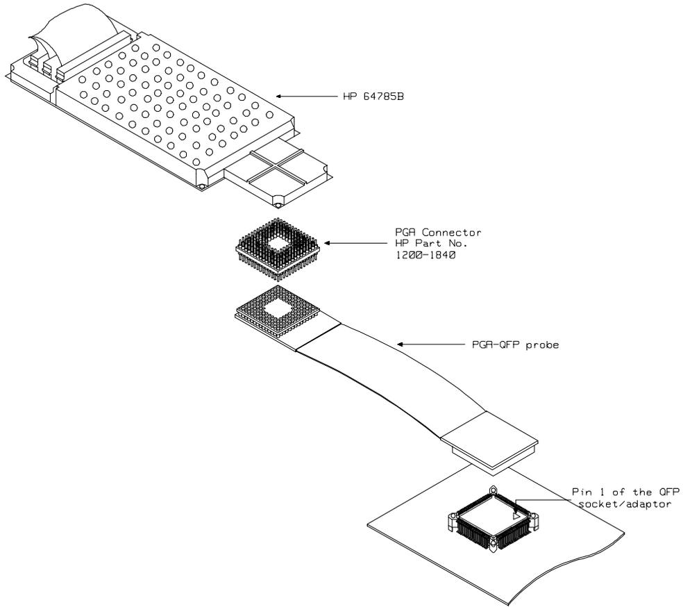
**Figure 4-6 Installing into a target system board**
