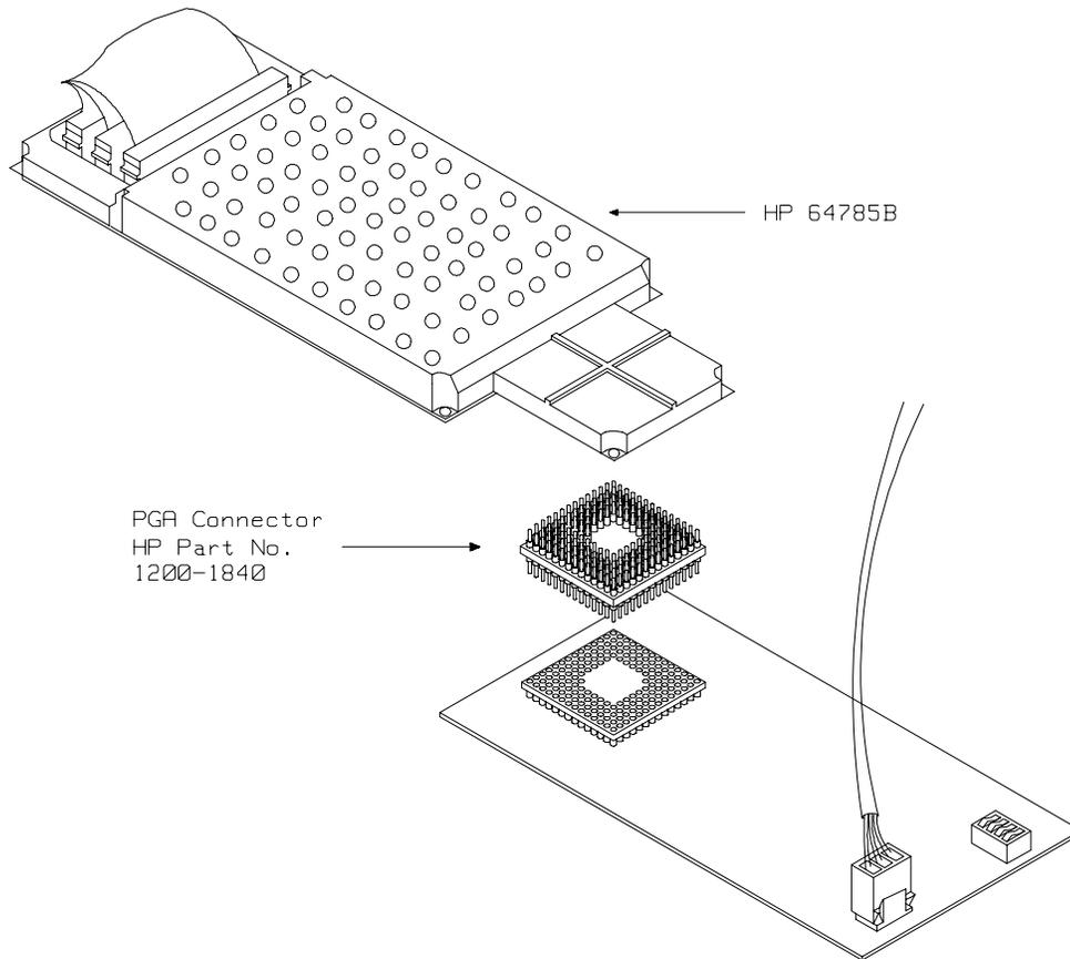
**Figure 4-5 Installing the demo target board**
