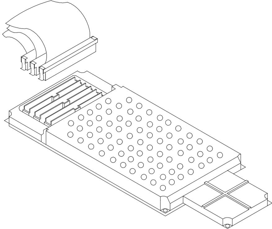
**Figure 4-3 Installing cables to the emulation probe**
