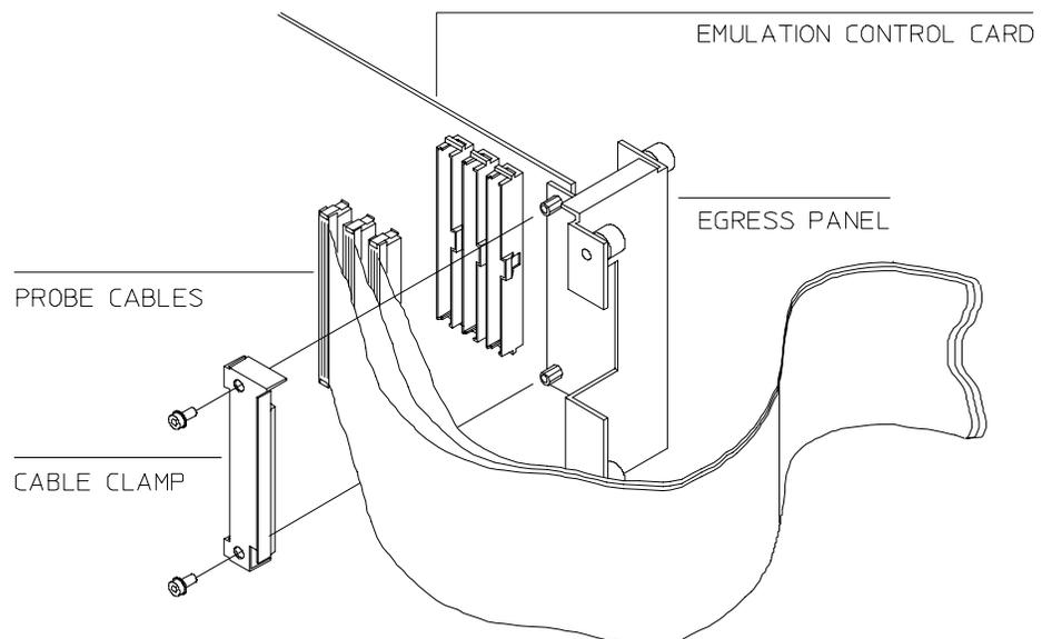
**Figure 4-1 Installing cables to the control board**
