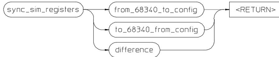
The **sync\_sim\_registers** command synchronizes the 68340's system integration module (SIM) registers to the emulator's CF\_SIM registers.
