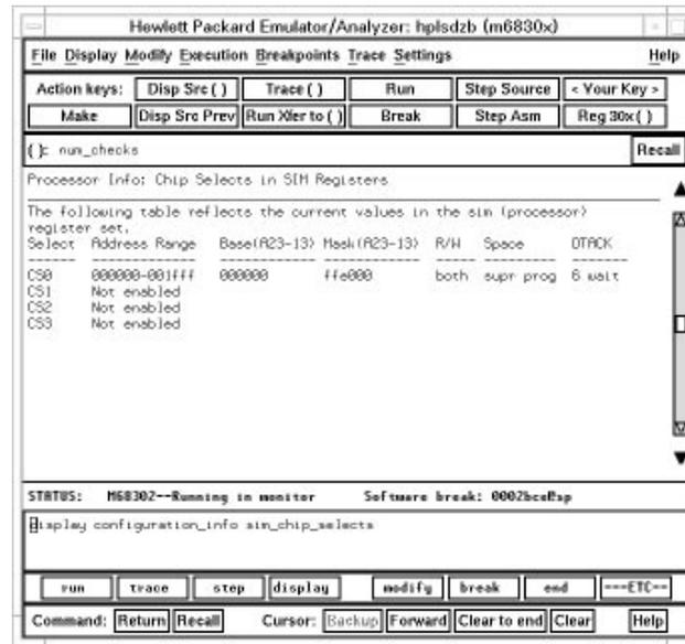
To display information about chip selects from the emsim (emulator) register set, choose **Display**→**Configuration Info**→**Chip Selects (Emulator SIM)** from either the configuration interface the emulator/analizer interface pull-down menu.
