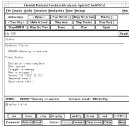
The first line of the emulation trace status display shows the user trace has been "completed"; other possibilities are that the trace is still "running" or that the trace has been "halted".
