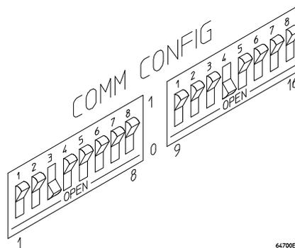
Notice that switches 1 through 3 are set to 001, respectively. This sets the baud rate to 19200.
