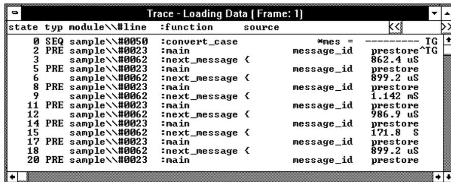
You can see how prefetching affects tracing by choosing the Display→Mixed Mode (ALT, -, D, M) command from the Trace window's control menu.
