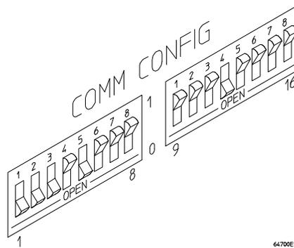
Notice that switches 1 through 3 are set to 111, respectively. This sets the baud rate to 230400.
