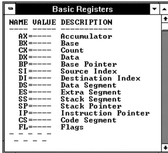
Notice that register contents are replaced with "----" in the display. This shows the debugger cannot update the register display. In order for the emulator to update its register display, the emulation monitor must interrupt target program execution while it reads the registers.
