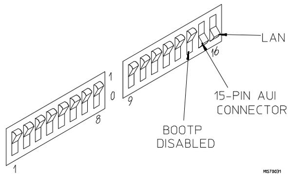
Switch 16 must be set to one (1) indicating that a LAN connection is being made.
