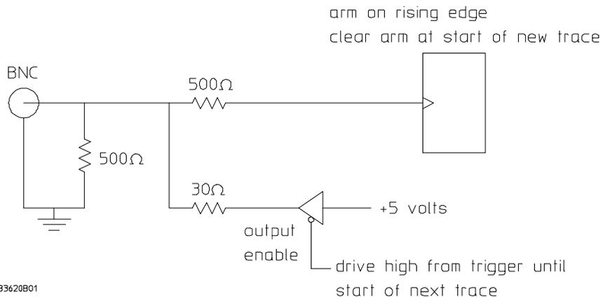
When a trace starts, it stops driving the output (so if nothing else is driving the line, it will fall low due to the 500 ohm pull-down resistor).
