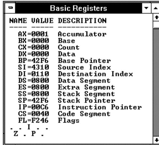
The screenshot shows a window titled "Basic Registers" with a table of register information. The table has three columns: NAME, VALUE, and DESCRIPTION. The registers listed are AX, BX, CX, DX, BP, SI, DI, DS, ES, SS, SP, IP, CS, and FL. Below the table, there are two lines of status flags: ". . I . ." and "Z . P .".
