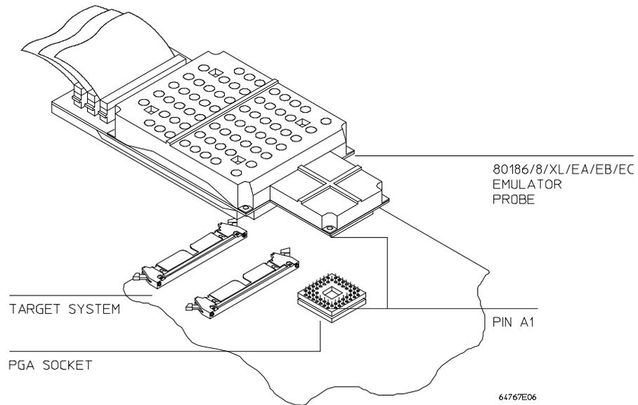
You can also use the supplied PGA to PLCC adapter or other QFP or PQFP adapters. Always make sure that pin 1 and other pins of the adapters and connectors are properly aligned; otherwise, damage to the emulator will result.
