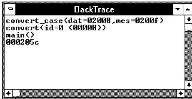
The BackTrace window is updated when program execution stops at an occurrence of breakpoint, break, or Step command.
