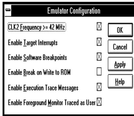
**CLK2 Frequency > 42 MHz** Specifies whether one wait state should be added for accesses to memory mapped into 4-Mbyte SIMMs. Note that CLK2 is the oscillator frequency to the Intel80386EX. It is twice the frequency of the usually-quoted value. For example, a "20 MHz Intel80386EX" has a CLK2 of 40 MHz.
