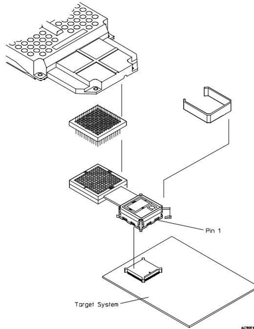
You can also use the supplied PGA to PGA adapter or other PQFP adapters. Always make sure that pin 1 and other pins of the adapters and connectors are properly aligned; otherwise, damage to the emulator will result.
