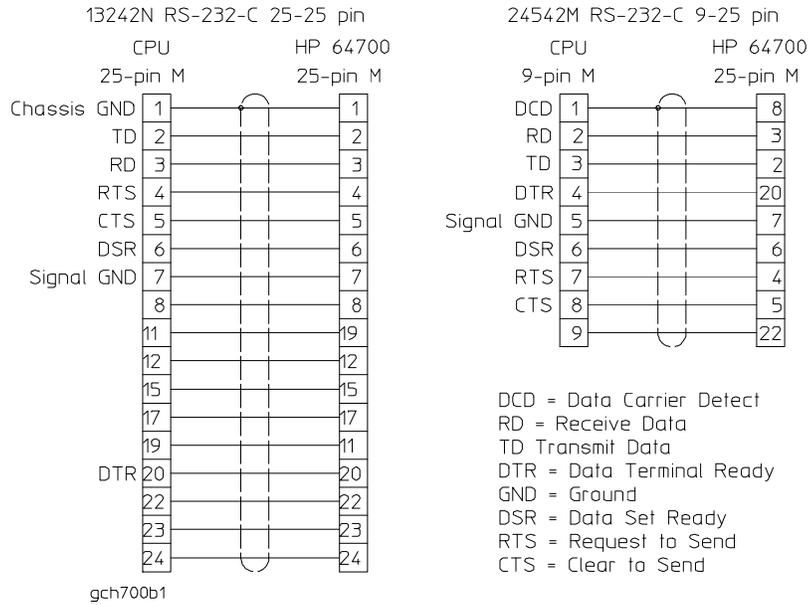
You can also use an RS-232C printer cable, but you must set HP 64700 configuration switch 4 to 1.
