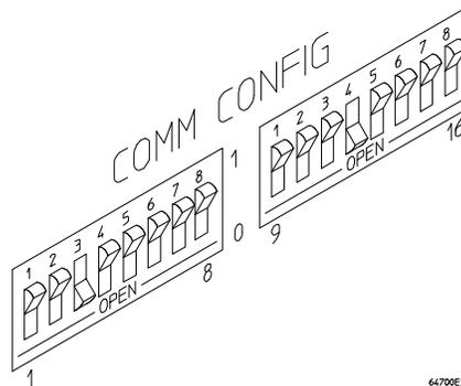
Notice that switches 1 through 3 are set to 001, respectively. This sets the baud rate to 19200.
