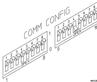
Notice that switches 12 and 13 are set to 1 and 0, respectively. This sets the RTS/CTS hardware handshake, which is needed to make sure all characters are processed. Switches 1, 2, and 3 are set to 0. This sets the baud rate to 9600. Switch settings are read during the HP 64700 power up routine.
