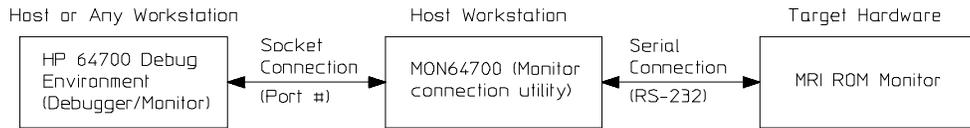
Mon64700 allows your workstation to simulate (act in place of) an HP 64700 emulator. When the debugger graphical interface is connected to mon64700, it works just as if it were connected to an emulator or a simulator. Mon64700 accepts the emulator commands generated by the debugger interface and translates them into the equivalent ROM monitor commands.
