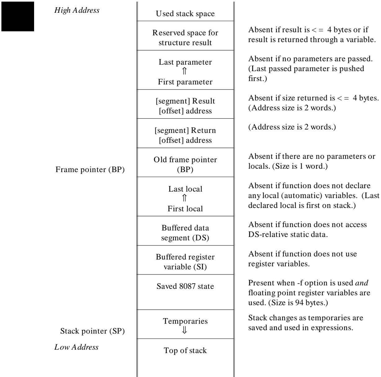
**Figure 15-3. Stack for Large Memory Model**
