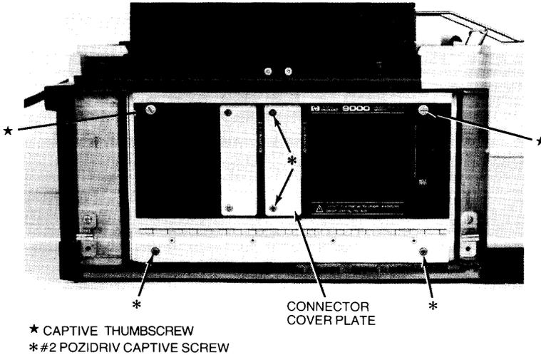
Figure 2. Series 500 Computer Stack Door Removal.
