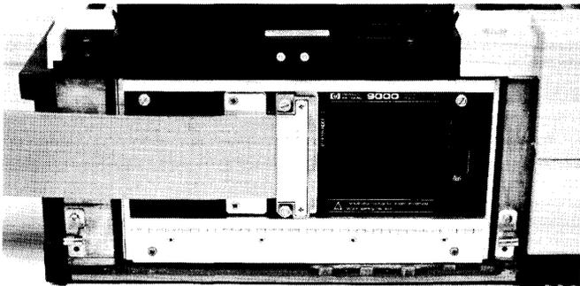
Figure 5. IOP Connector Attached to Door.
