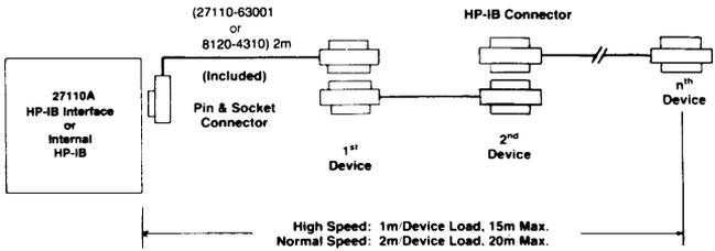
**HP 27110A HP-IB Interface Cabling**
