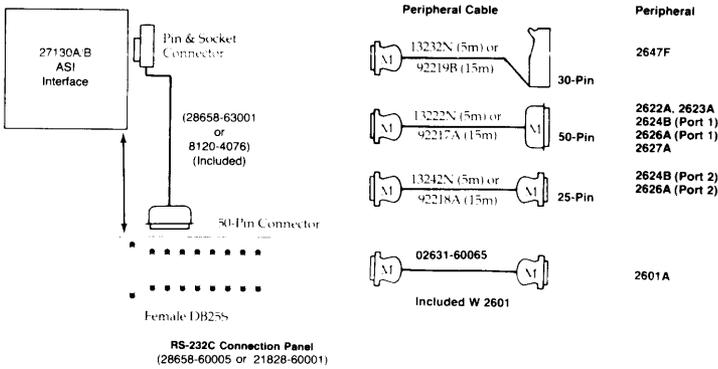
HP 27130A/B Asynchronous 8-Channel Multiplex Cabling
