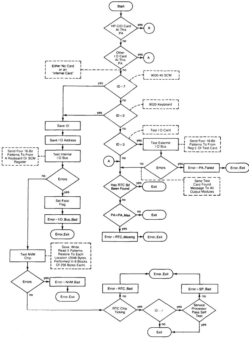
Loader ROM Test Module Flowchart
