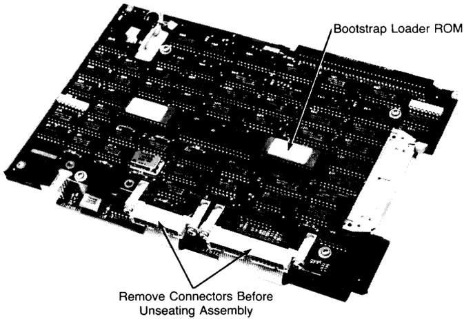
Figure 2. Fixed Disc Controller Assembly
