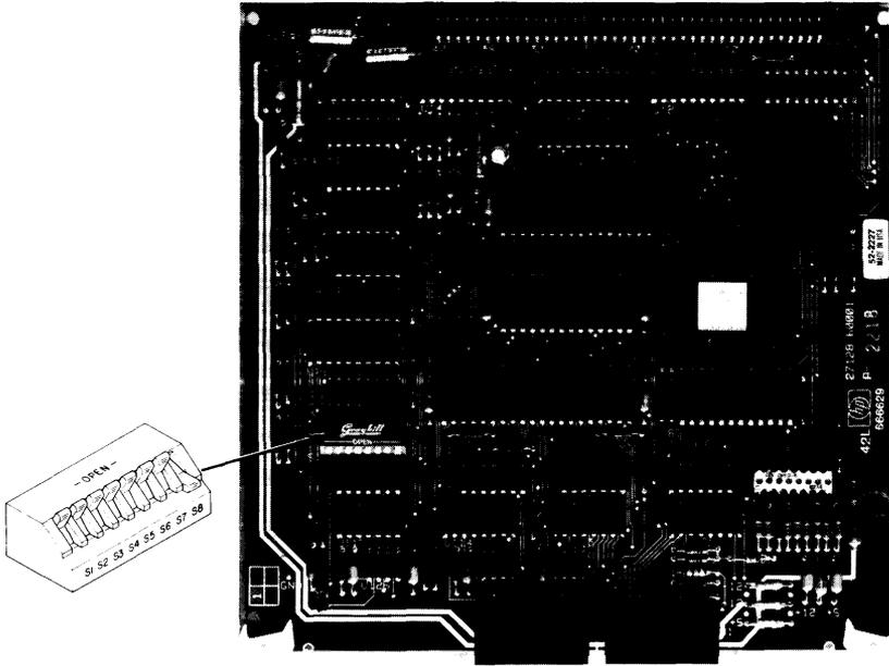
HP 27128A Asynchronous Serial Interface (ASI) Card
