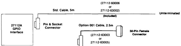
**HP 27112A GPIO Interface Cabling**
