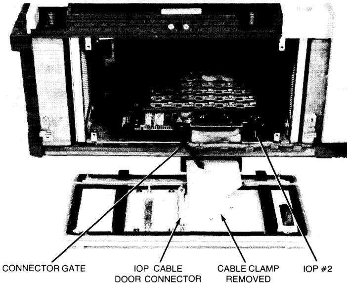
Figure 3. Series 500 Computer IOP Installation.
