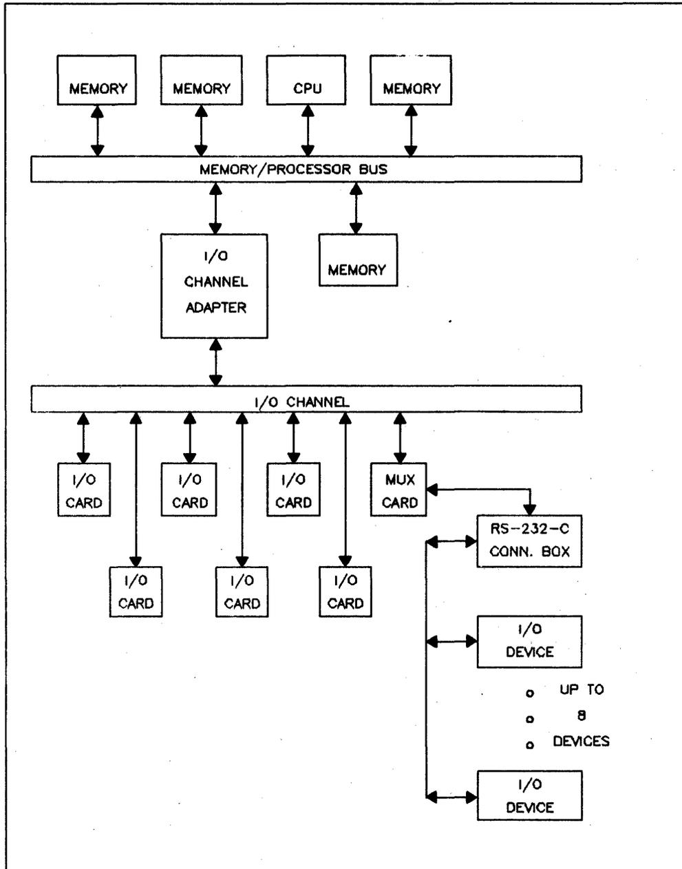
Figure 1-2. MUX in a Typical Hewlett-Packard Computer System
