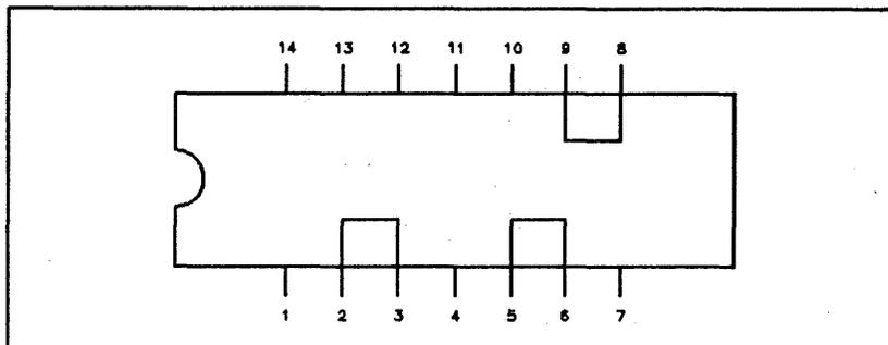
Figure 2-3. Signature Analysis Jumper Internal Connections
