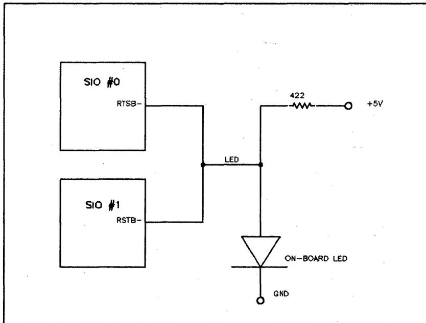
Figure 3-3. Control Circuit for the MUX Card LED
