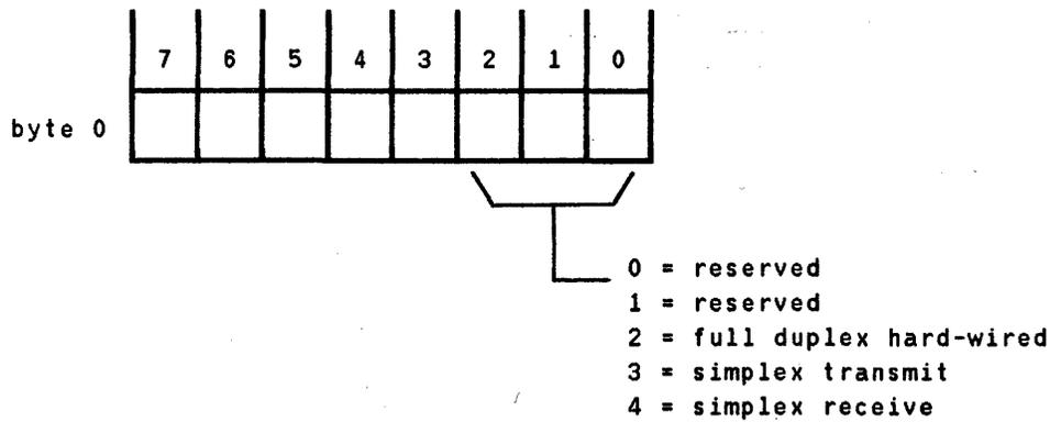
Validation: The parameter value must be within the range 2 through 4, inclusive. The transmission mode must be set before setting the read option. Note that the echo bit will be reset if the transmission mode is not full duplex.
