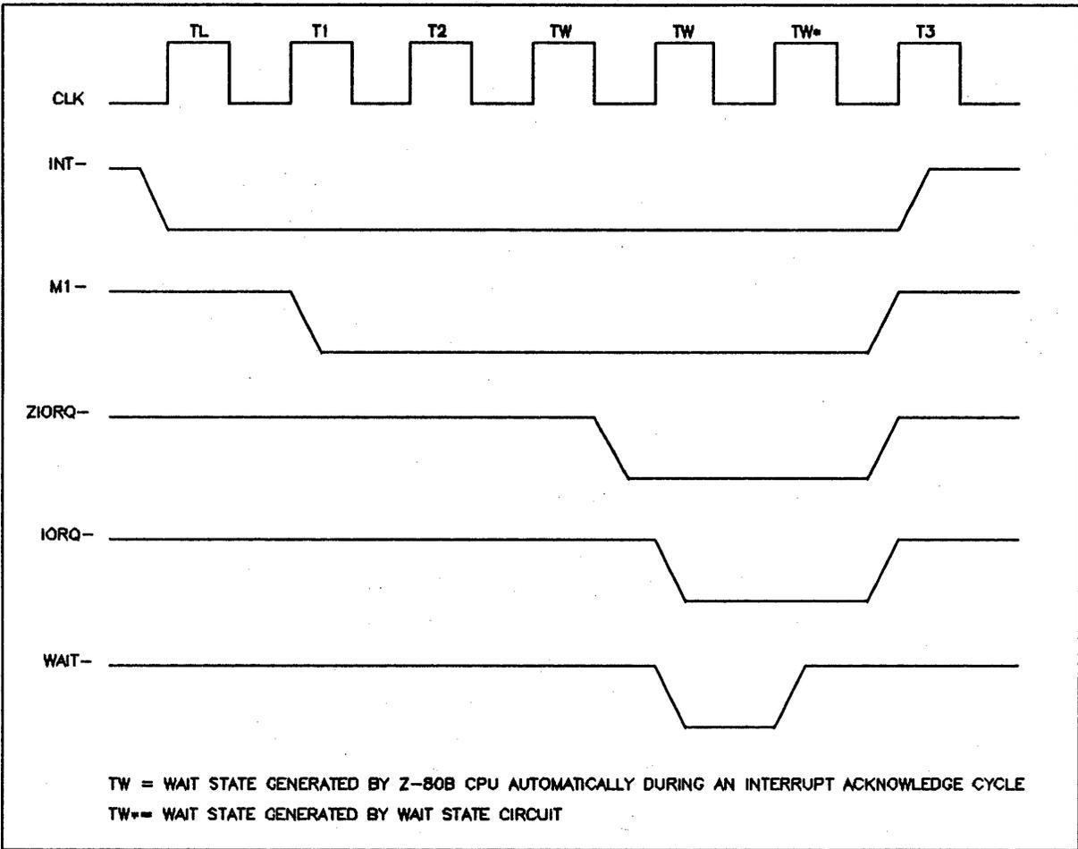
Figure 3-6. Wait State Circuit Timing Diagram
