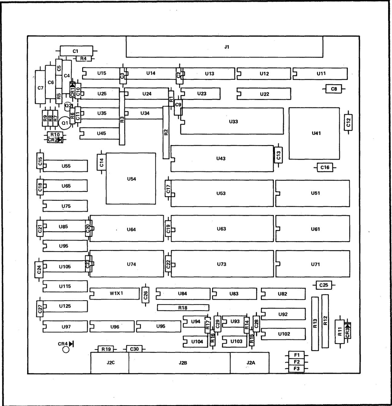
Figure 6-1. HP 27130A Parts Location Diagram
