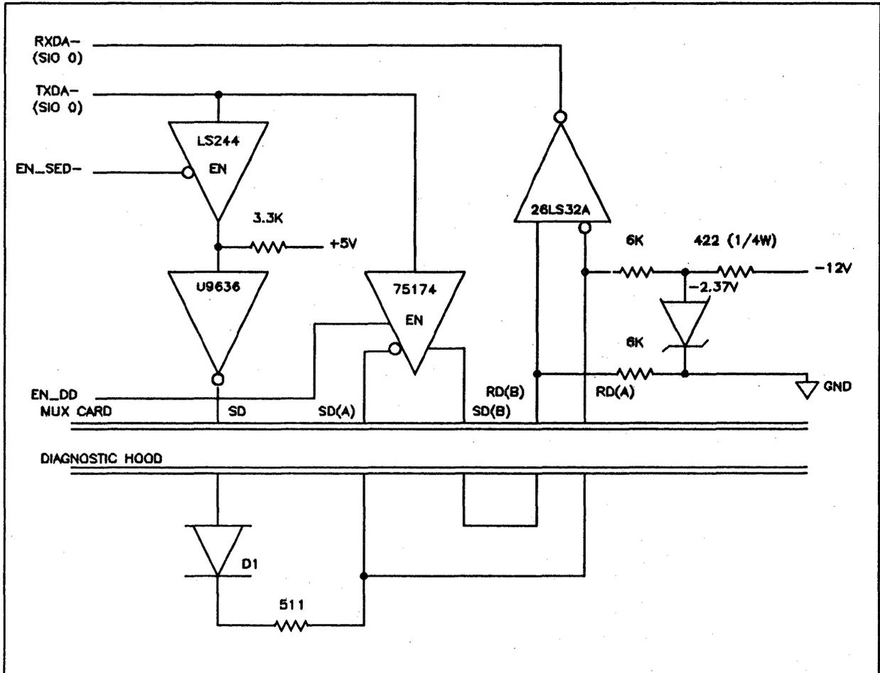
Figure 3-7. Diagnostic Test Hood Schematic Diagram
