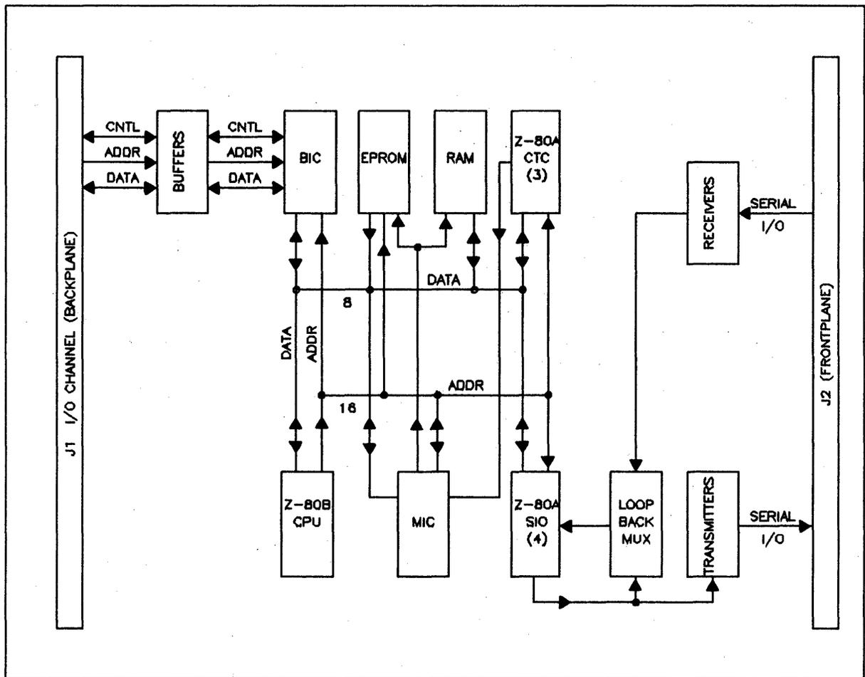
Figure 3-1. MUX Functional Block Diagram
