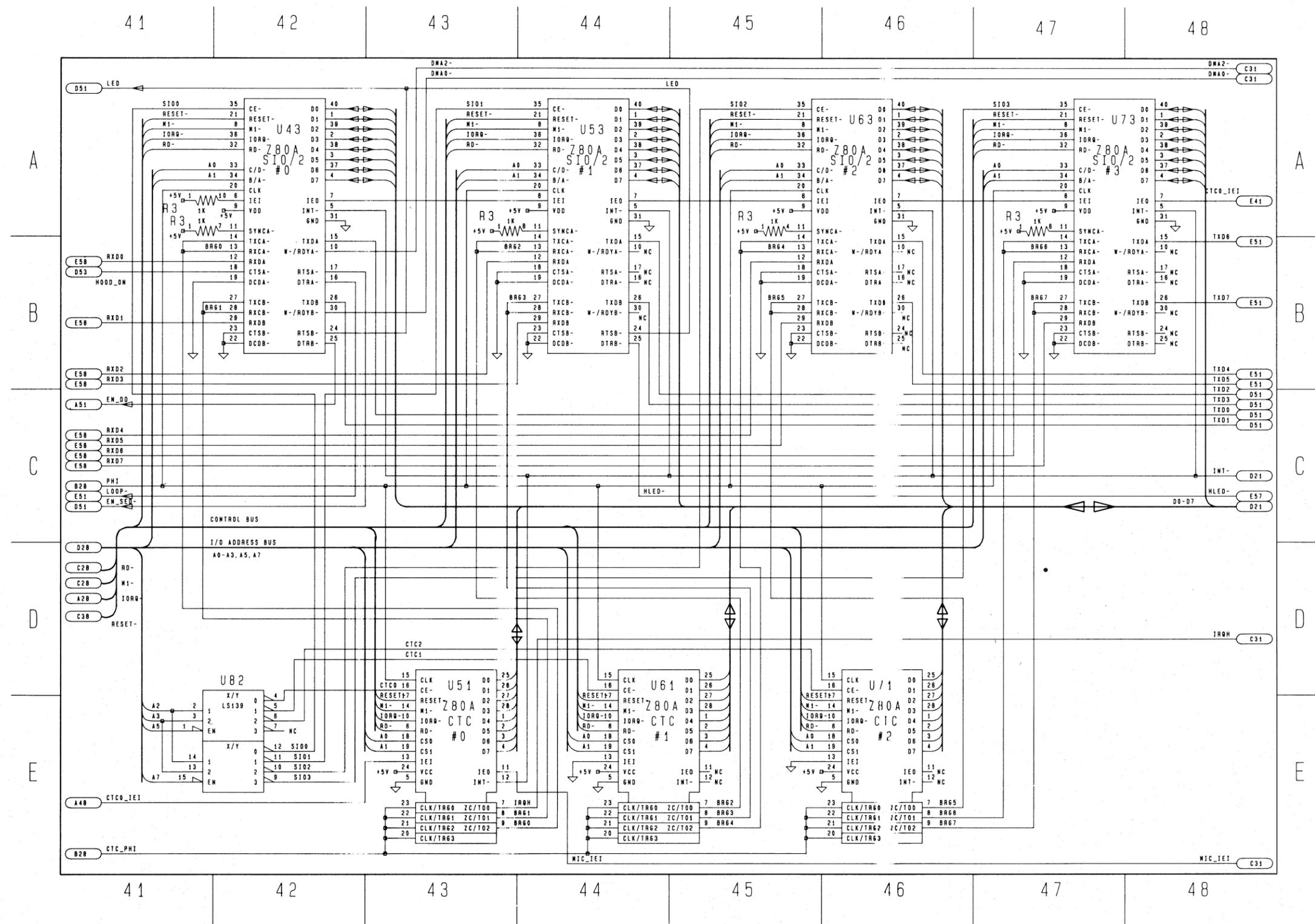
Figure 7-1. MUX Schematic Logic Diagram (Sheet 4 of 5)
