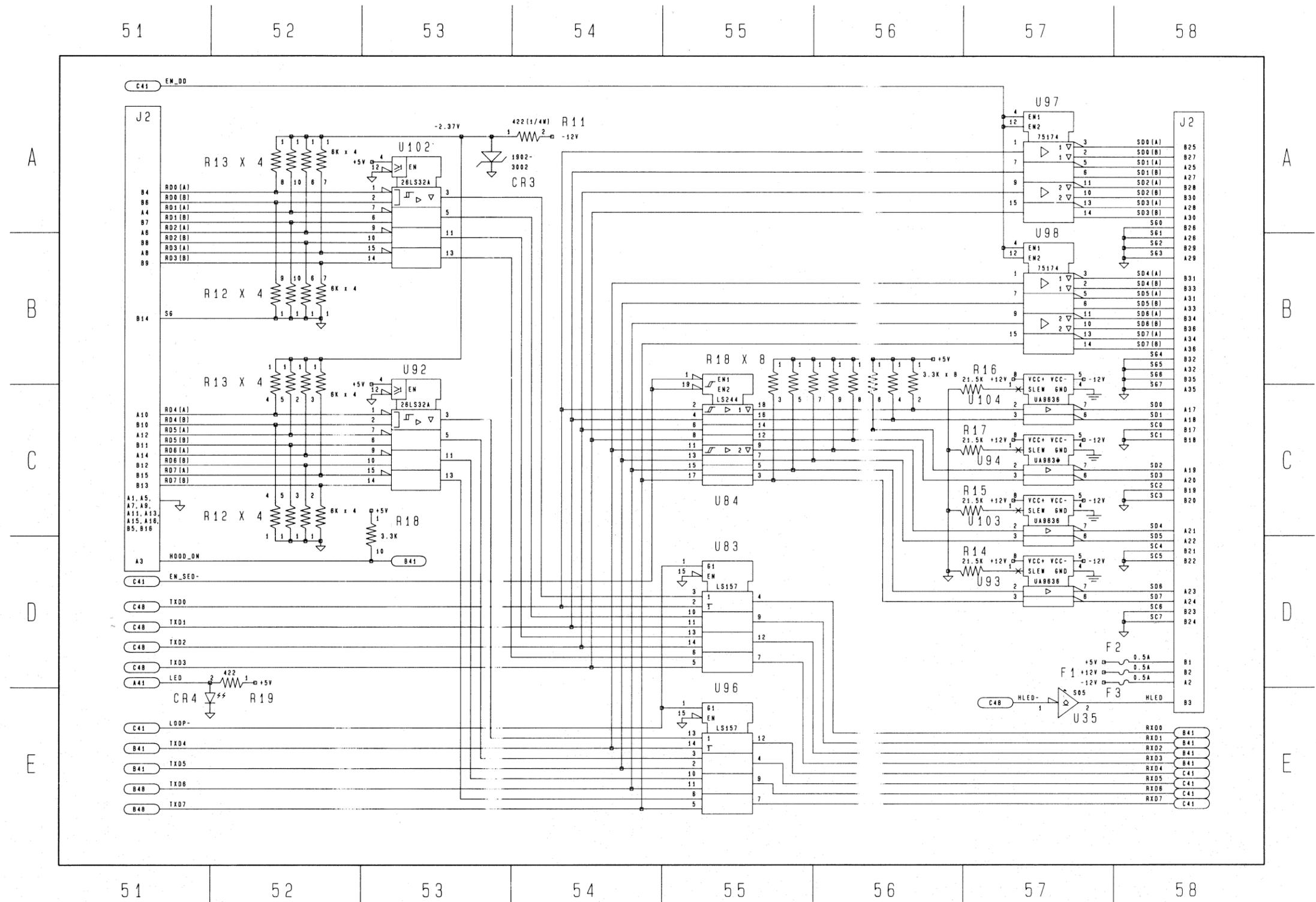
Figure 7-1. MUX Schematic Logic Diagram (Sheet 1 of 5)
