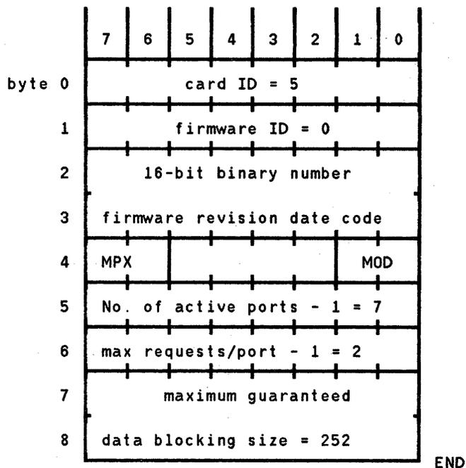
MPX = 1 for in-channel multiplexing
