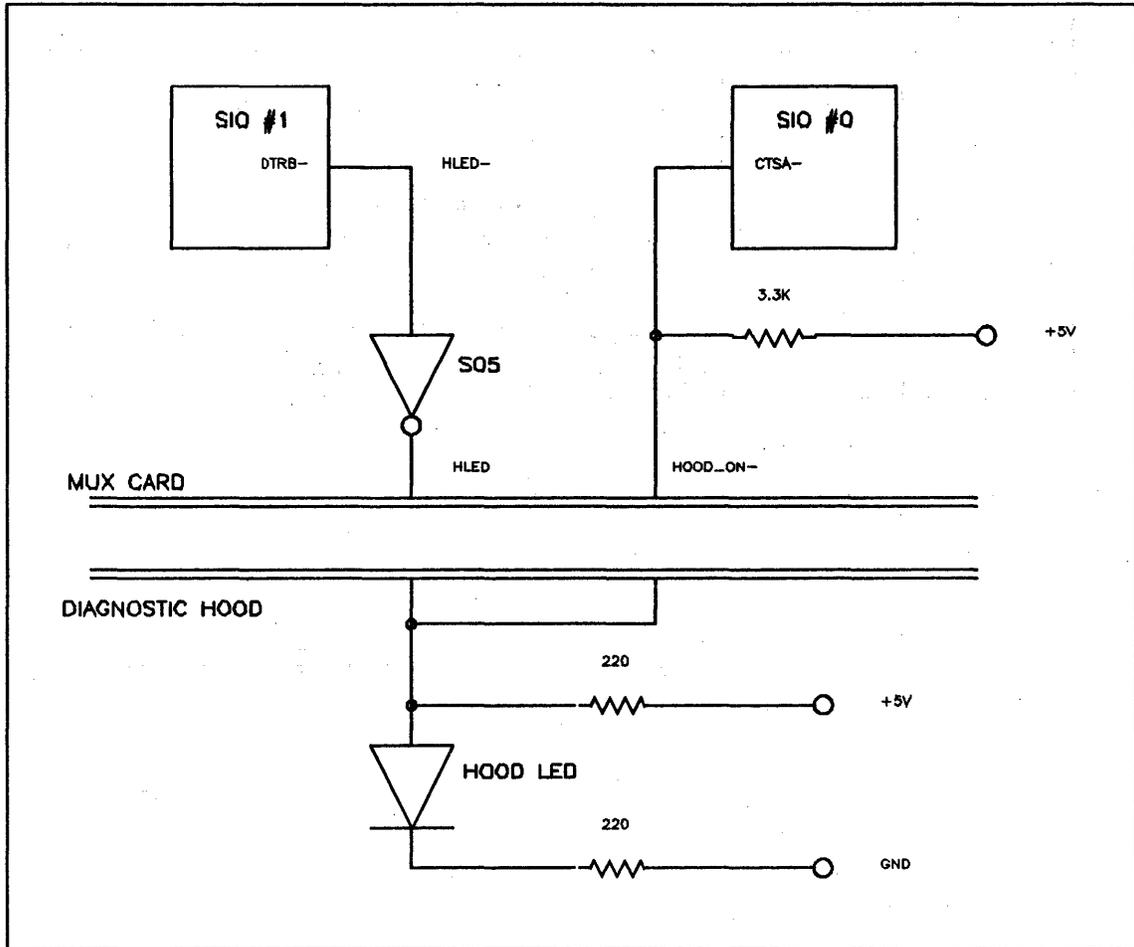
Figure 3-4. Diagnostic Hood LED Control Circuit and Hood Sense Circuit
