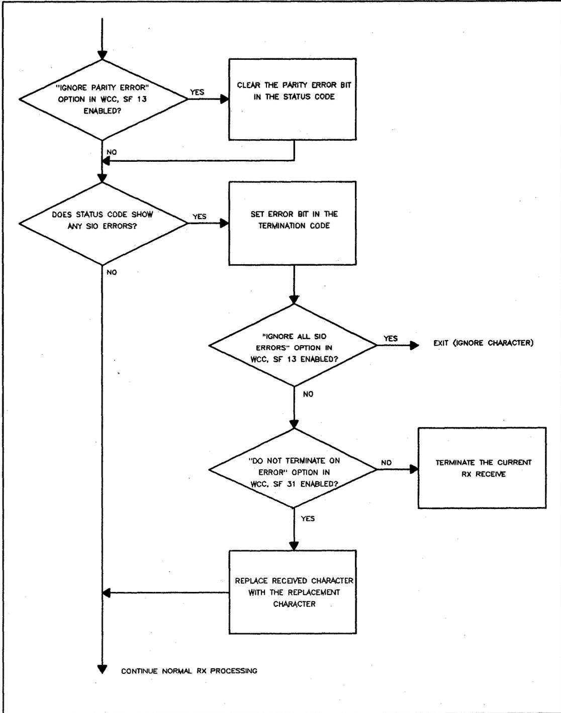
Figure 4-2. Error Handling Flow Chart
