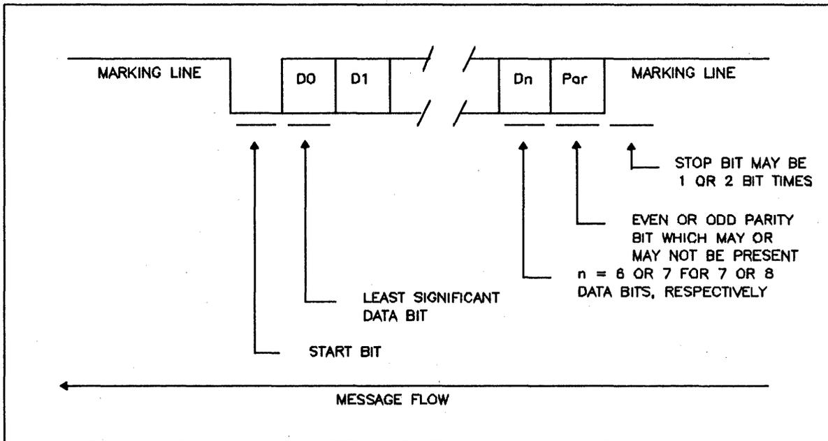
Figure 4-1. Asynchronous Message Format
