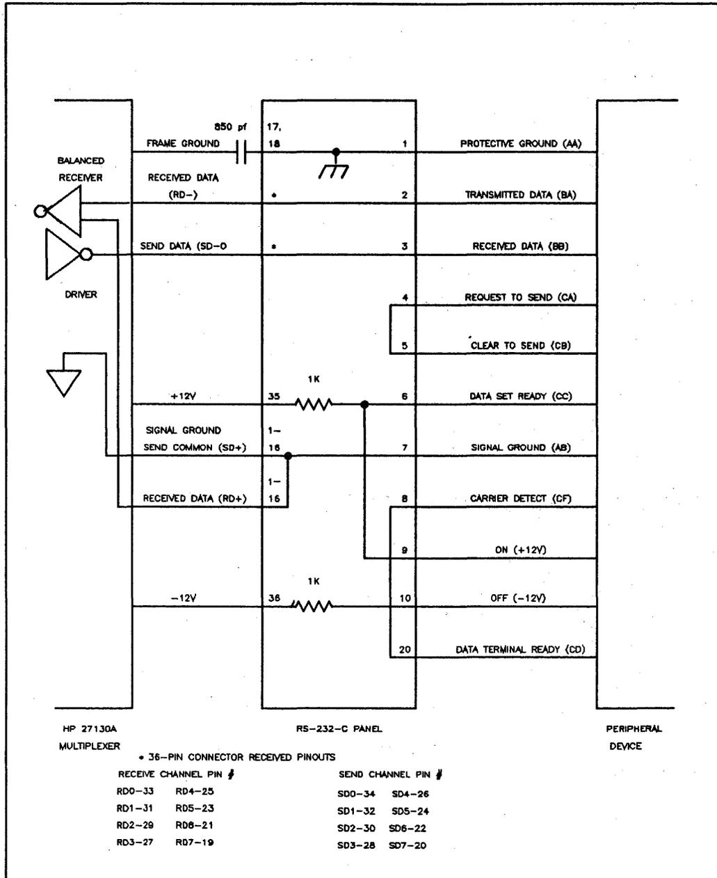
Figure 2-4. Connections from MUX to Connection Box to Device
