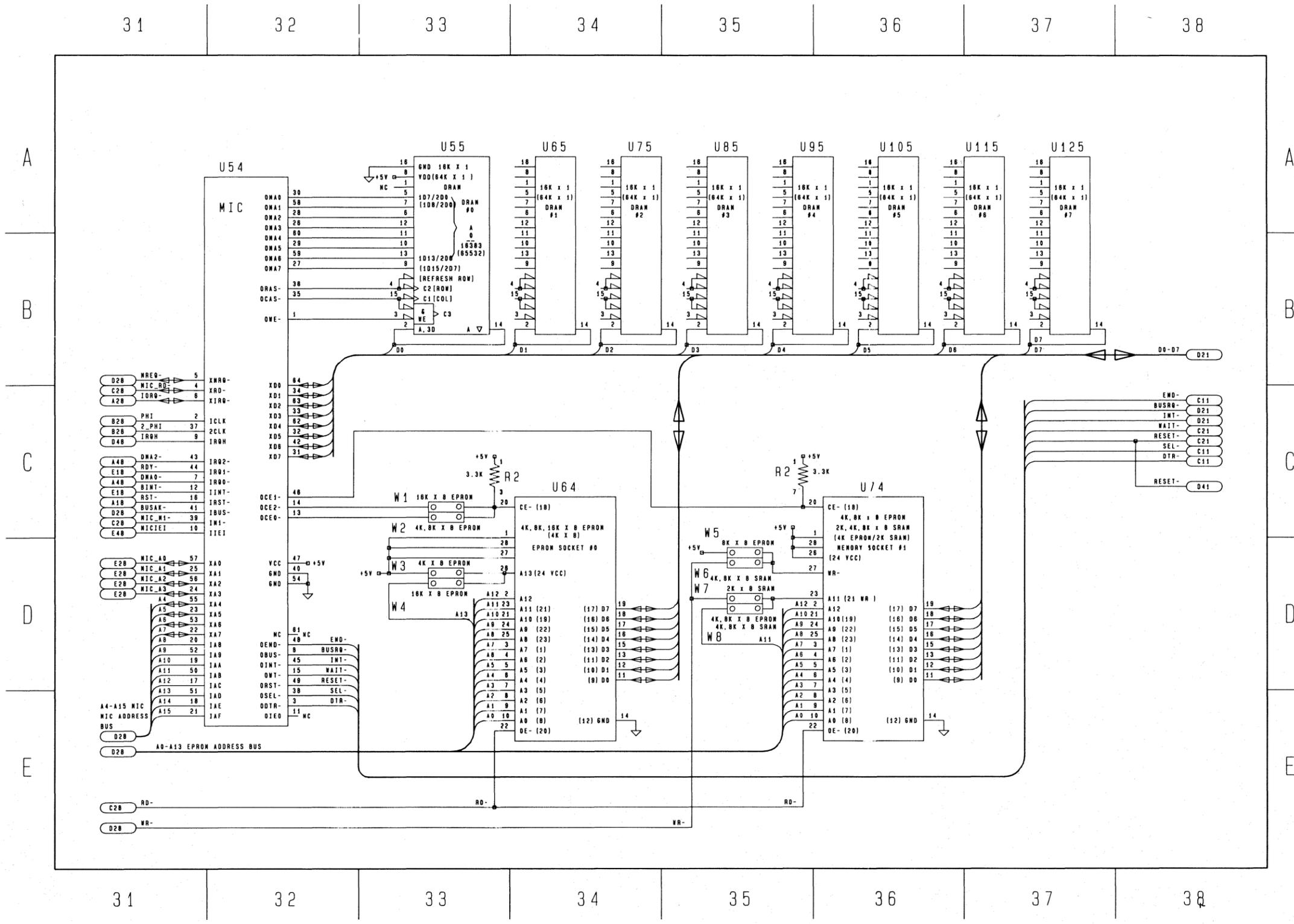
Figure 7-1. MUX Schematic Logic Diagram (Sheet 3 of 5)
