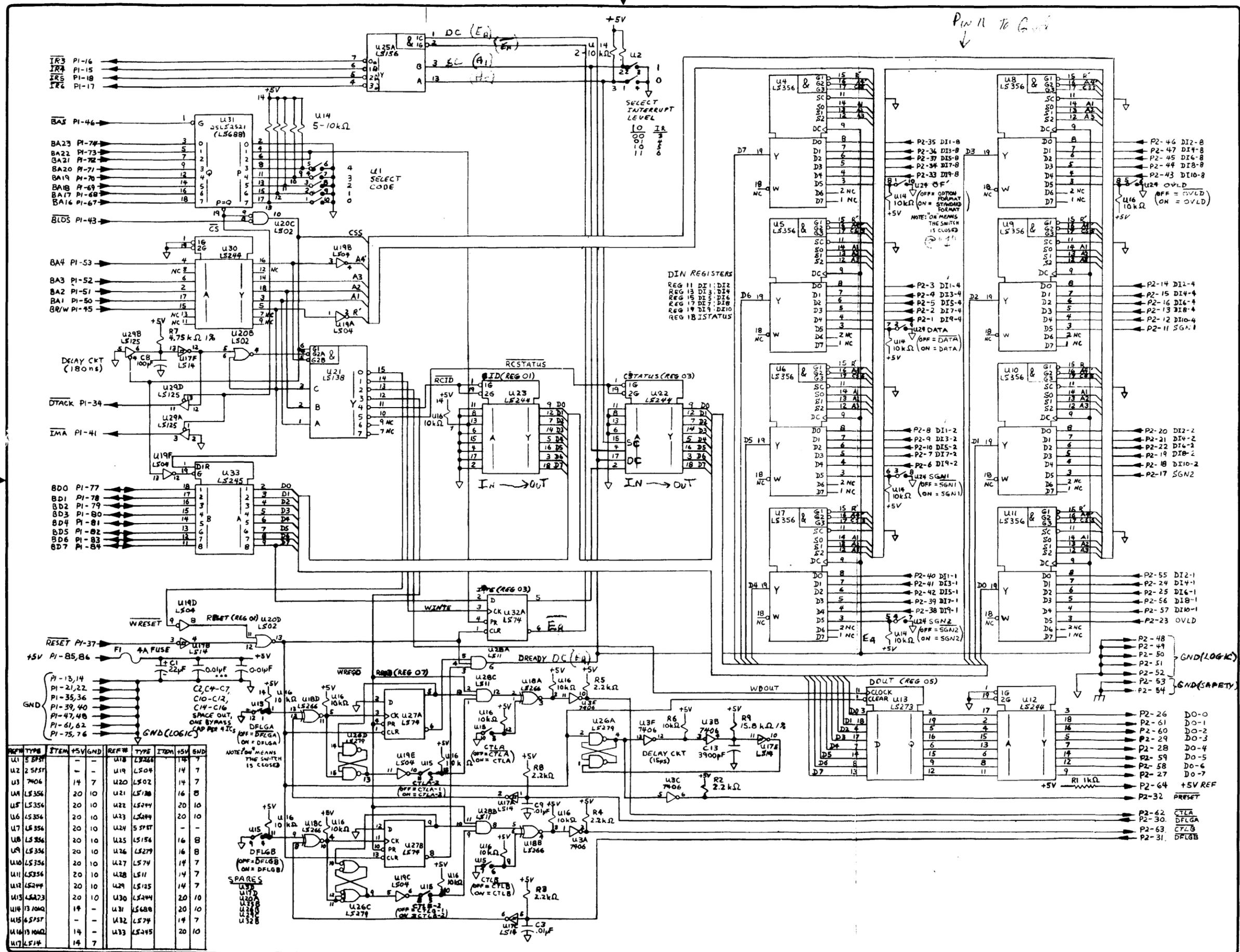
Figure 2. BCD Interface Card Schematic Diagram
