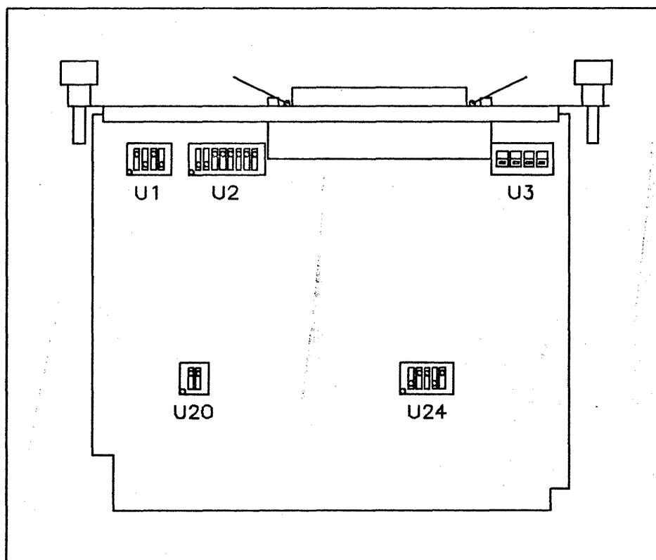
FIGURE #4 - 98626-66501 SHIPPING SWITCH POSITIONS
