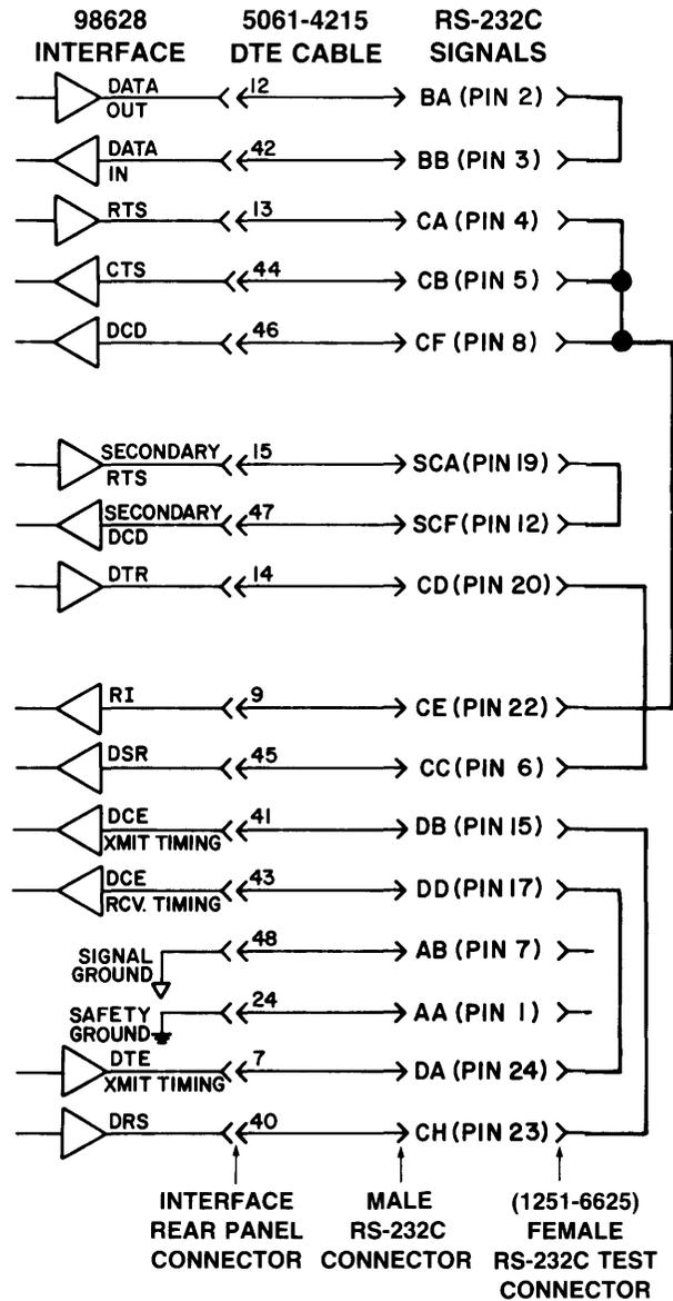
Option 001 DTE Interface Cable and Test Connector
