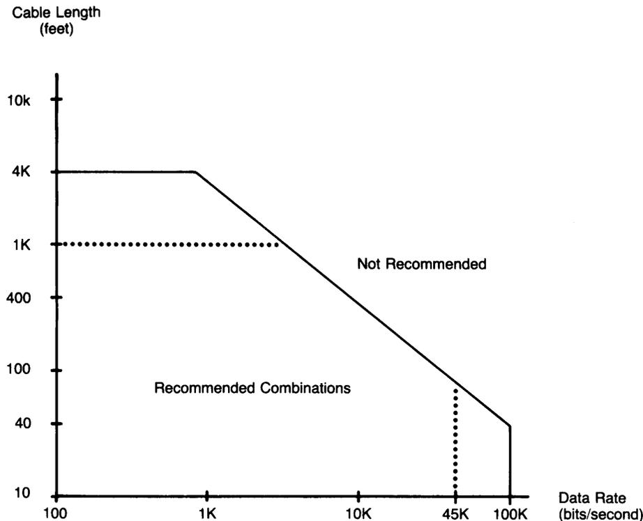
**RS-423 Modulation Rate Versus Cable Length**
