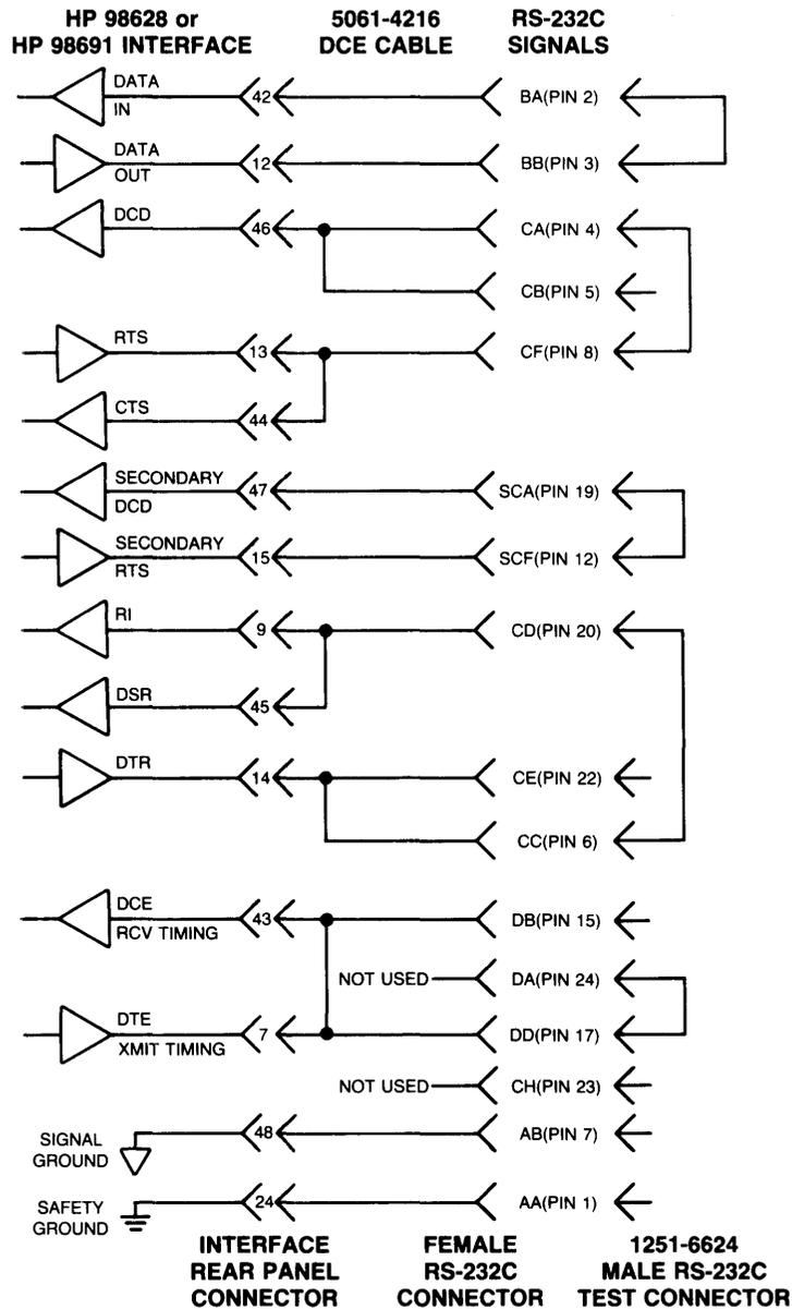
Option 002 DCE Interface Cable and Test Connector
