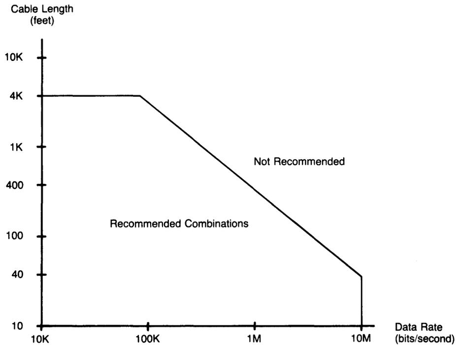
RS-422 Modulation Rate Versus Cable Length
