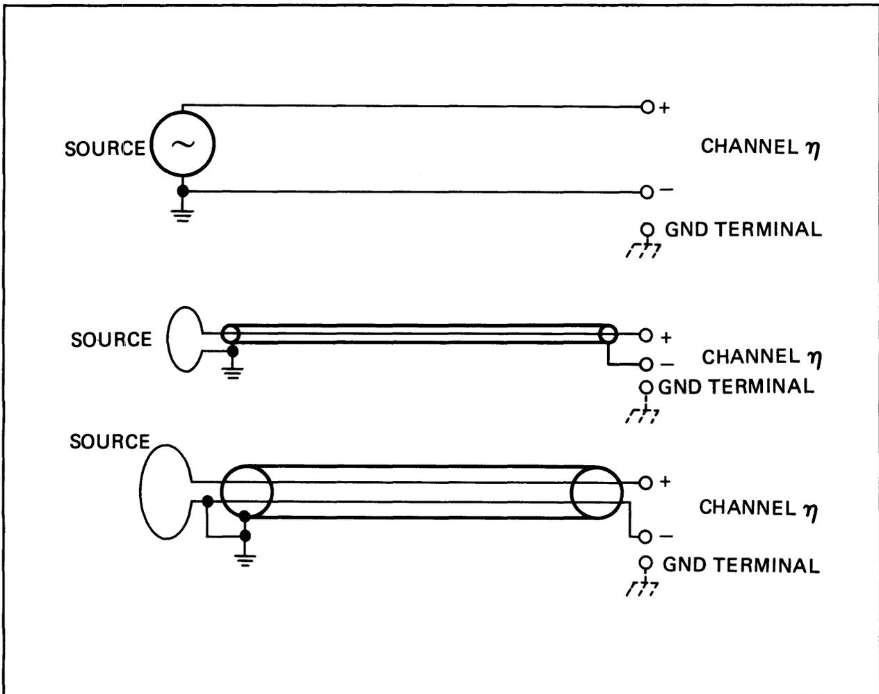
Figure 2-5. Wiring a channel's inputs.
