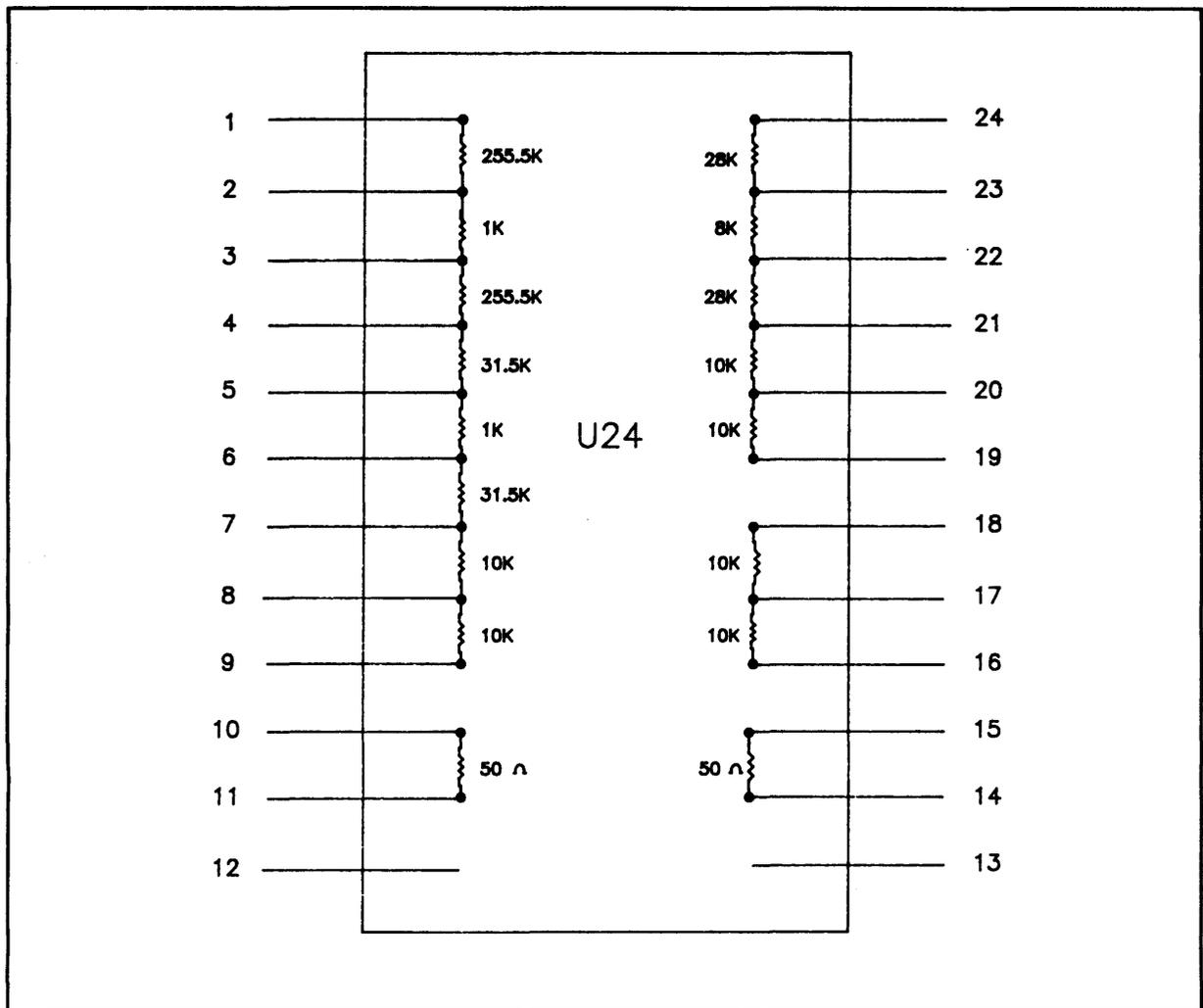
Figure 3-4. Precision resistor network (U24)
