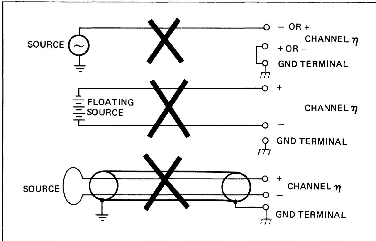
Figure 2-6. Unacceptable wiring of the inputs.
