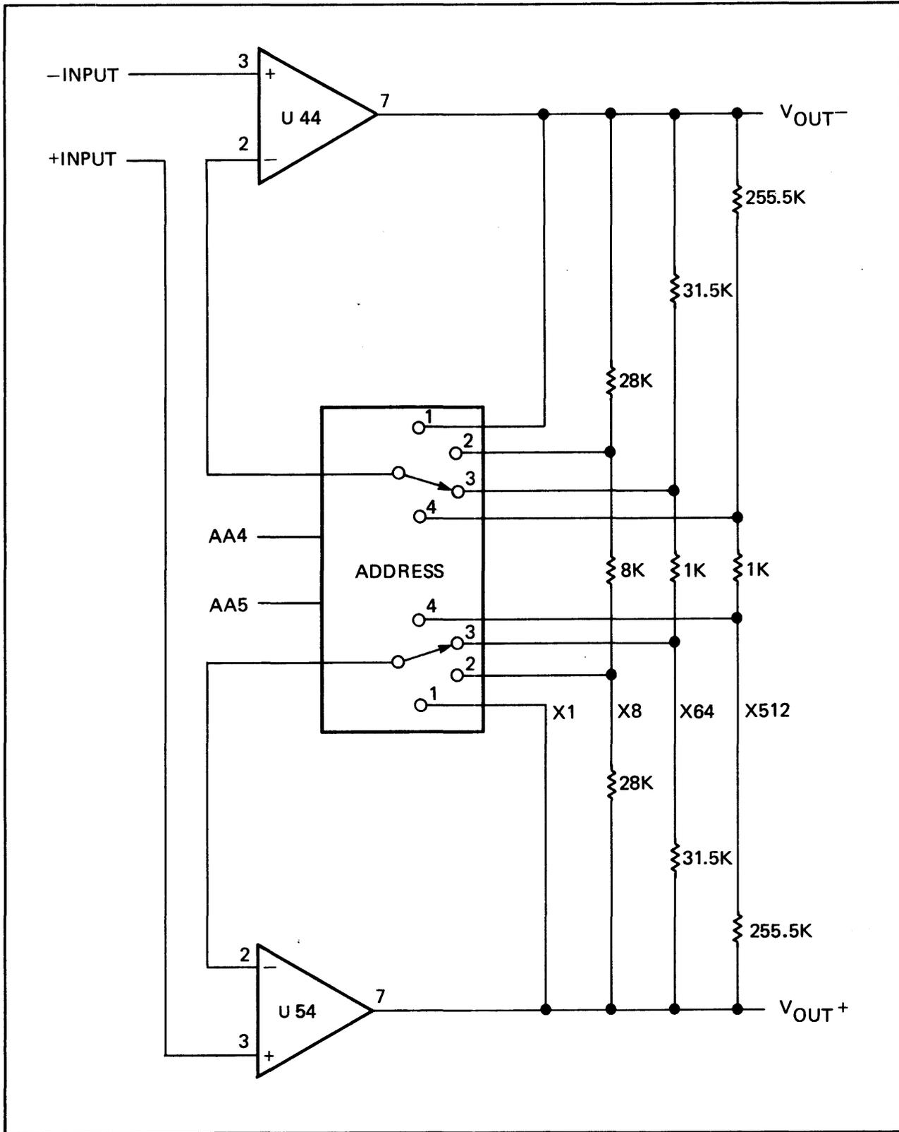
Figure 3-3. Programmable gain amplifier
