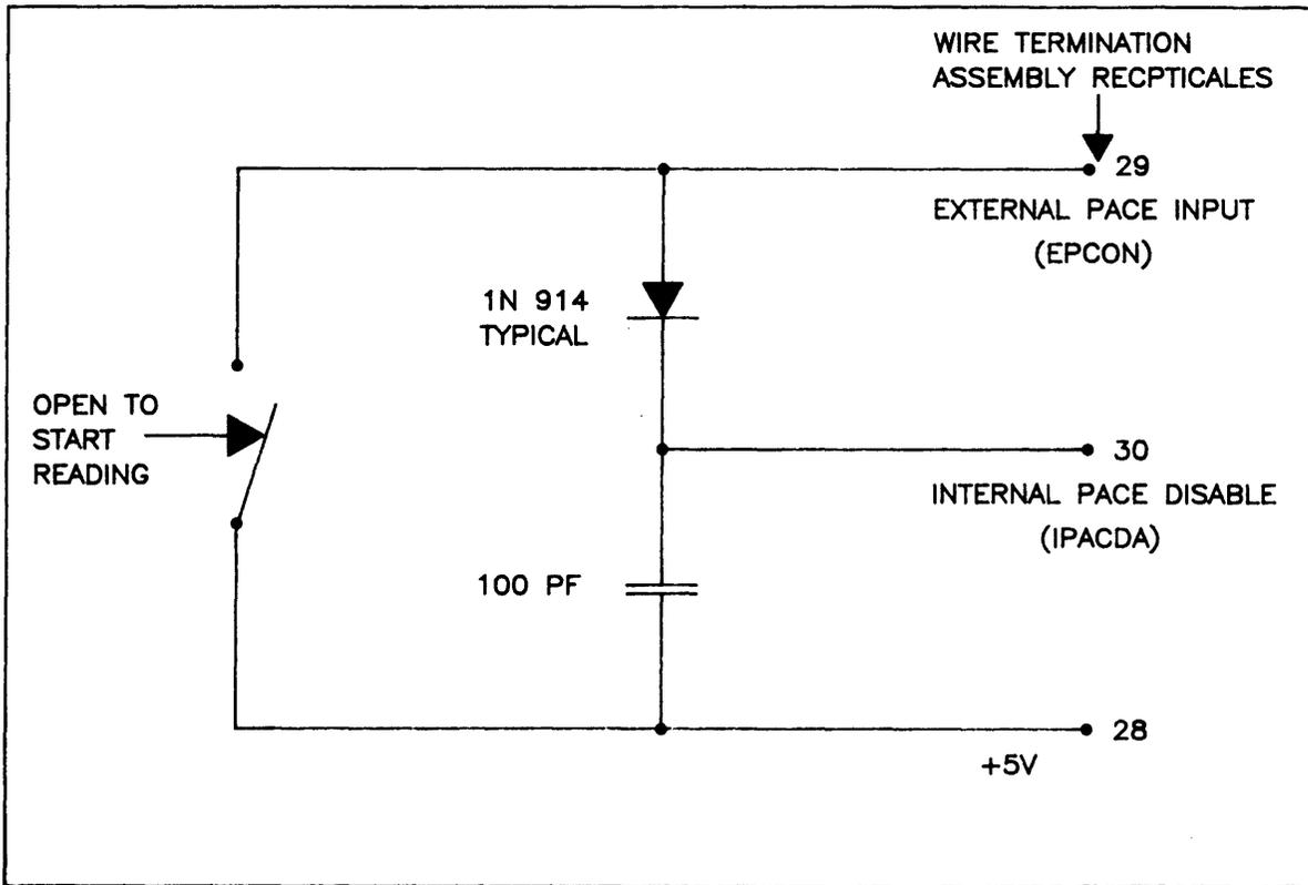
Figure 4-1. IPACDA timing circuit for externally paced burst readings
