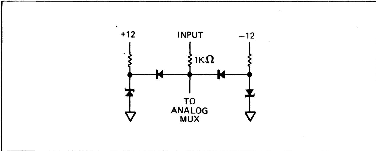
Figure 3-2. Input circuit
