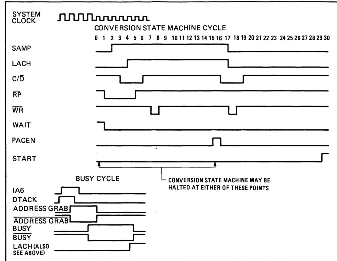
Figure 3-7. Control signal timing, PROM U68 and BUSY state machine.
