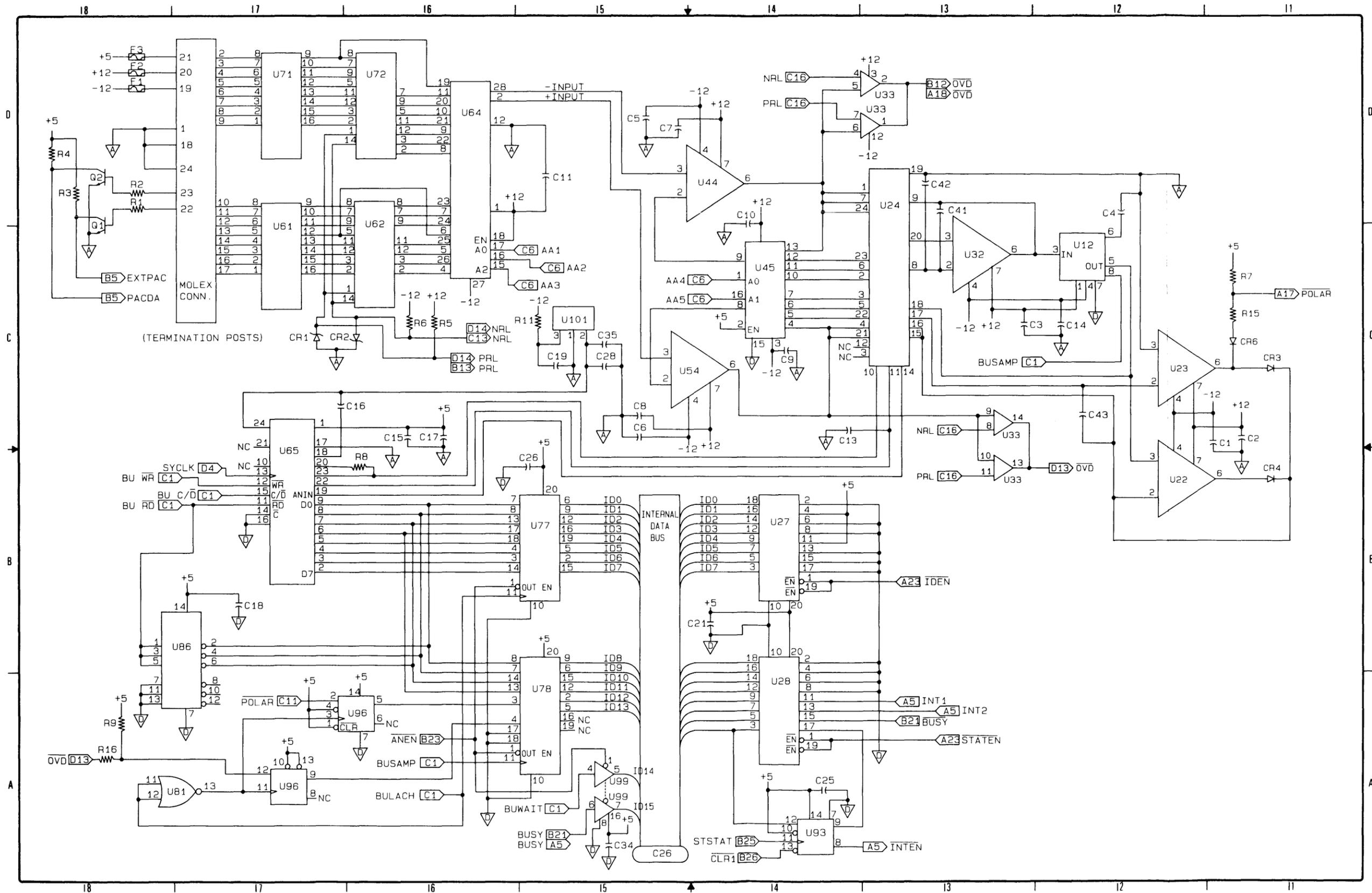
Figure 7-4. A-to-D card schematic diagram, sheet 2 of 3.
