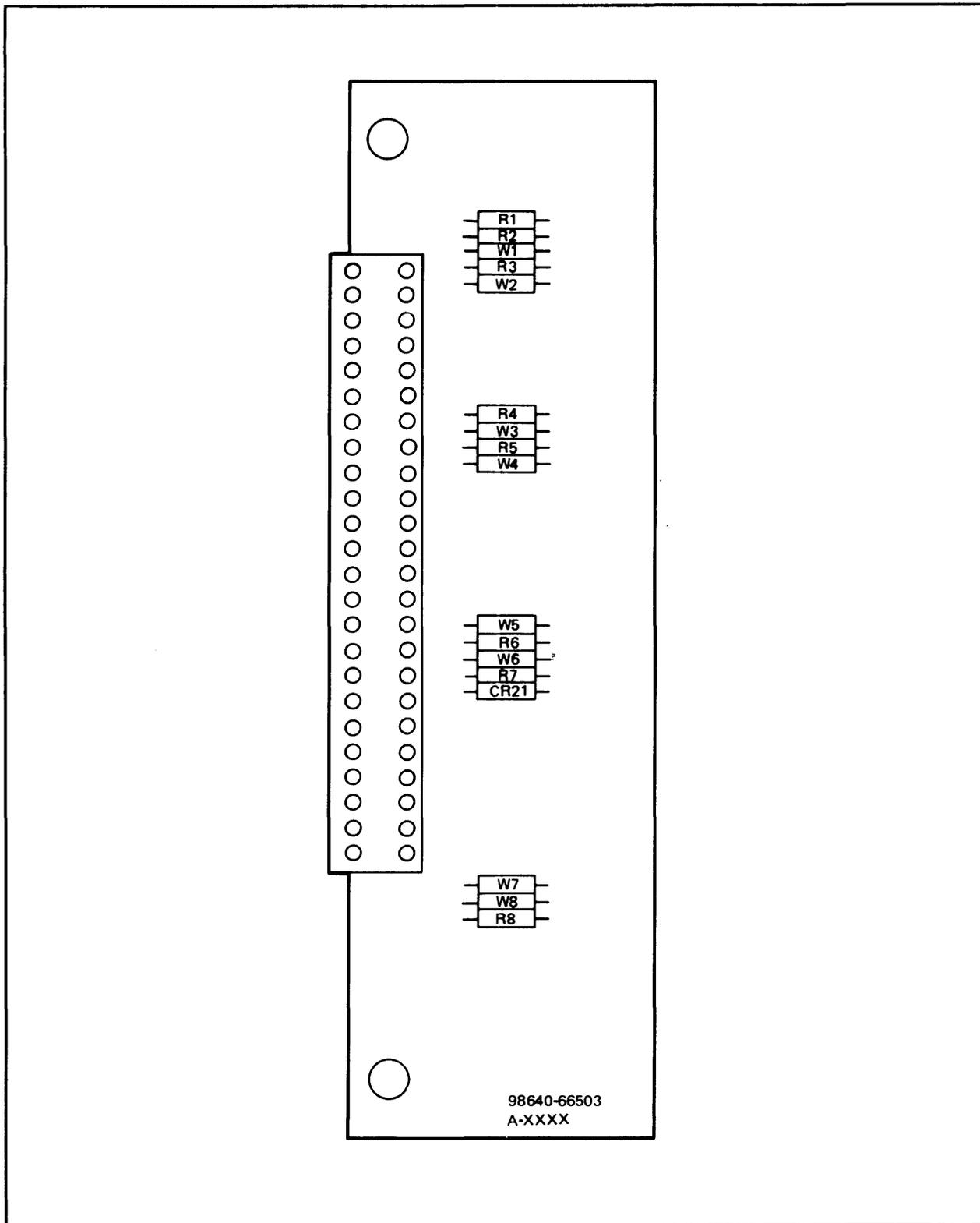
Figure 7-3. Component locations on the test assembly.
