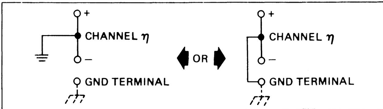
Figure 2-4. Wiring a reference channel.
