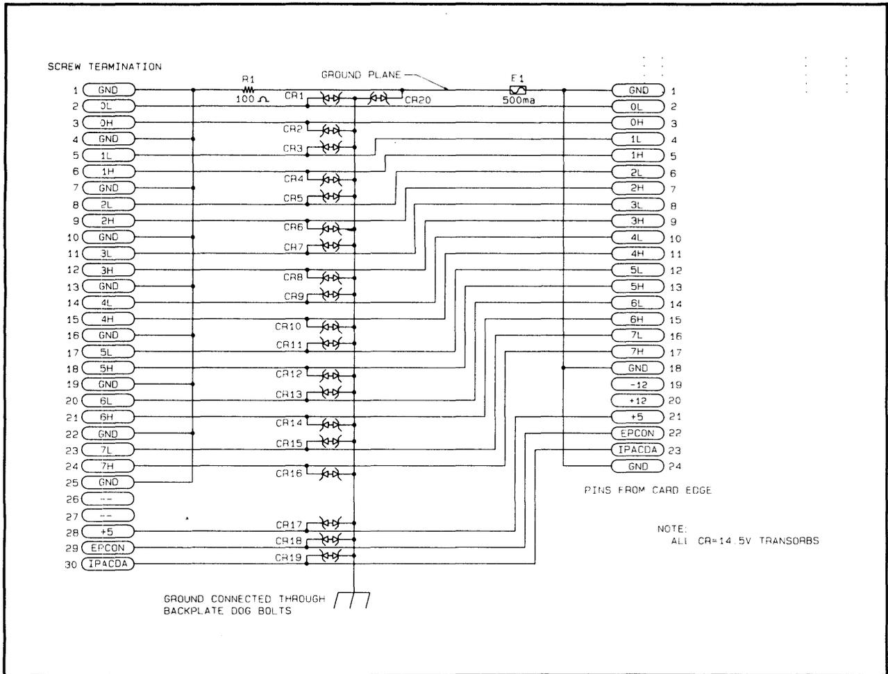
Figure 7-5. Wire termination assembly schematic diagram.
