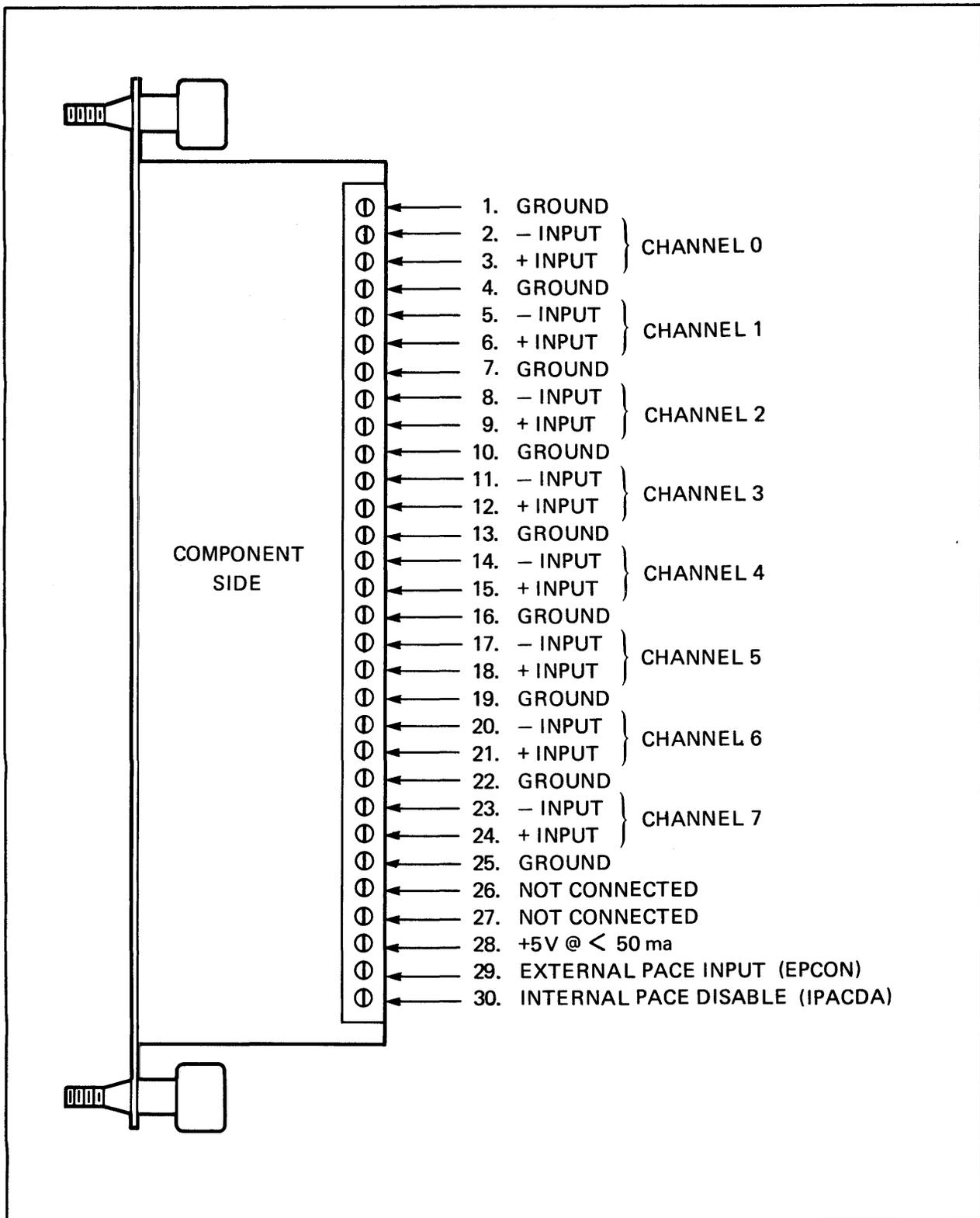
Figure 2-3. Wire termination assembly inputs.
