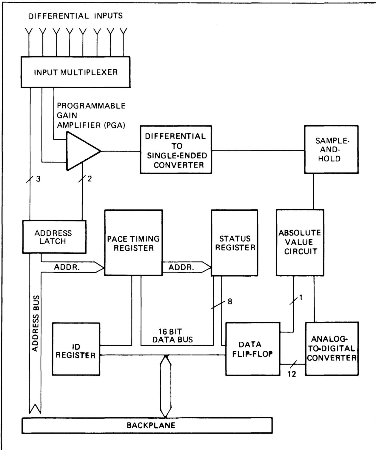
Figure 3-1. A-to-D card functional block diagram
