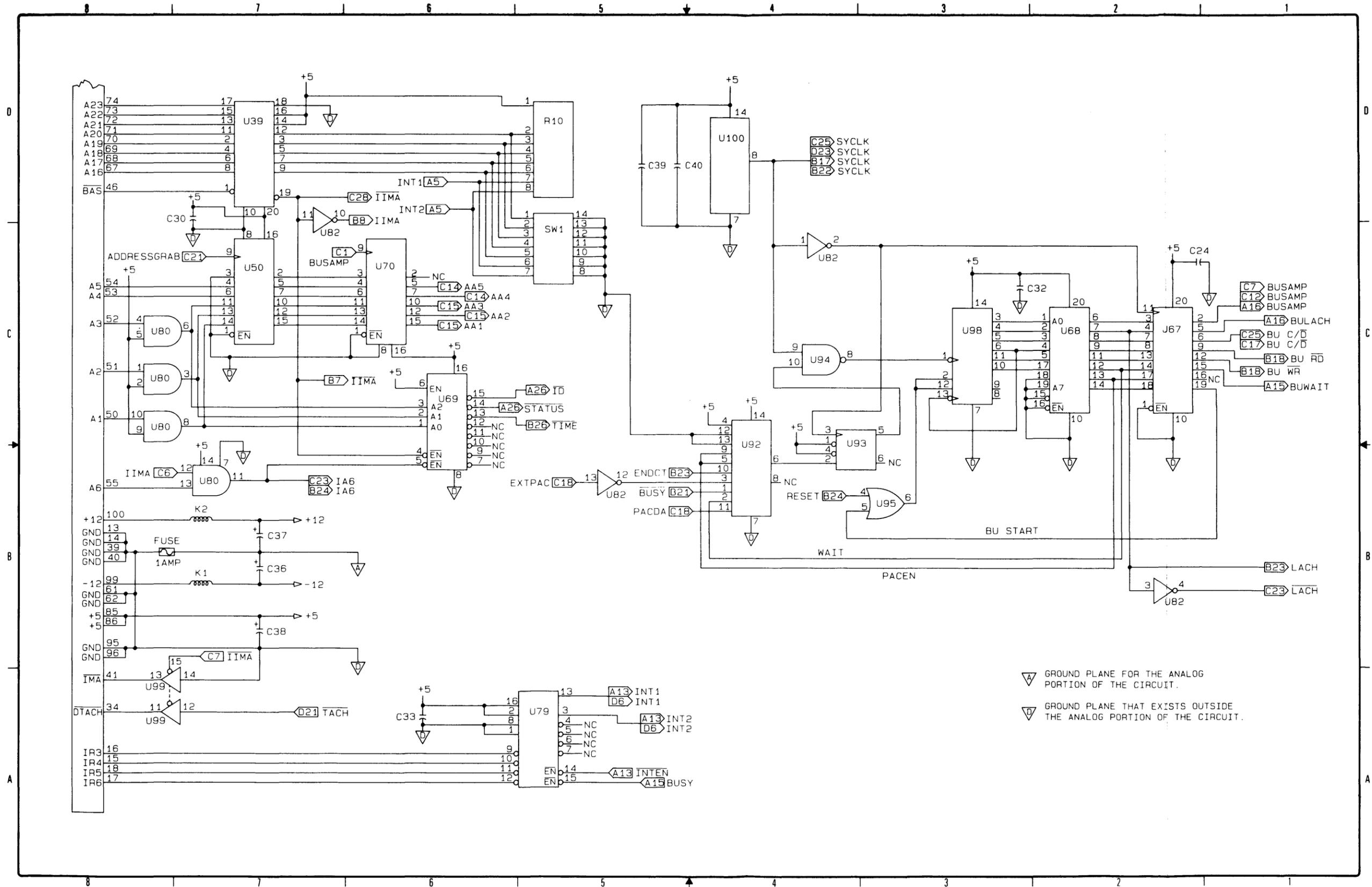
Figure 7-4. A-to-D card schematic diagram, sheet 1 of 3.
