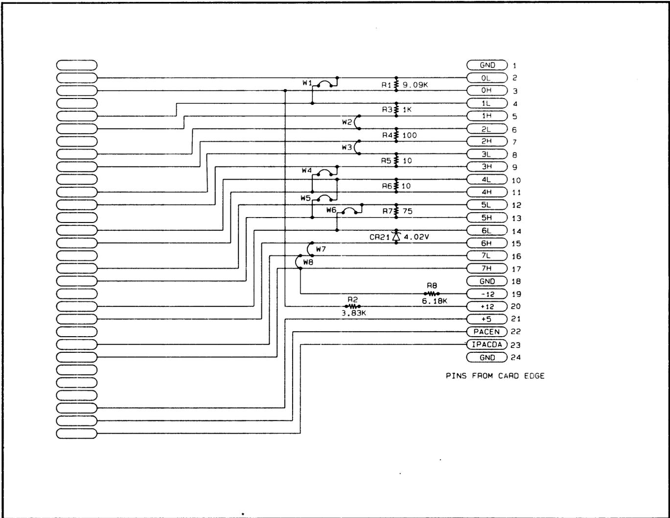
**Figure 7-6. Test assembly schematic diagram.**
