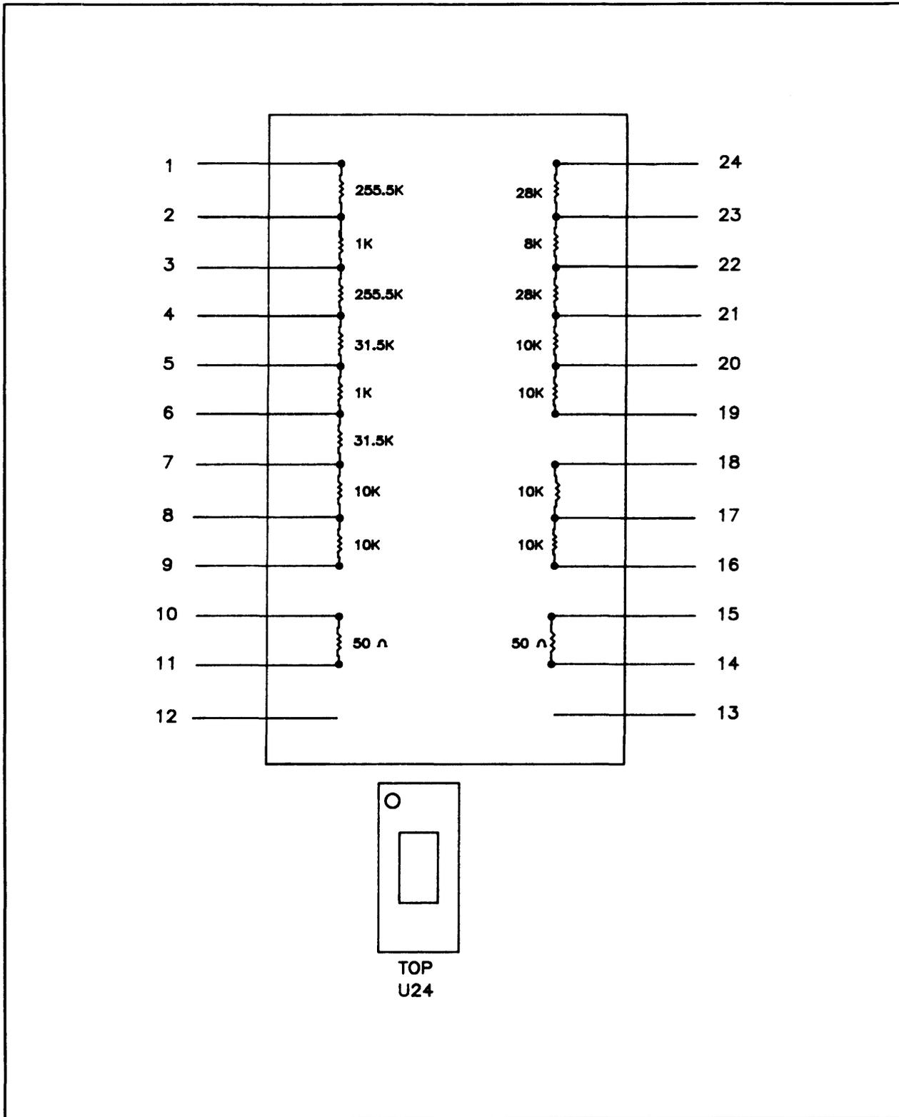
Figure 7-1. Custom resistor network.
