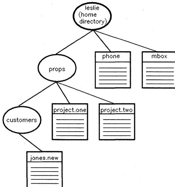
Figure 5-1. A Typical HP-UX Directory Structure
