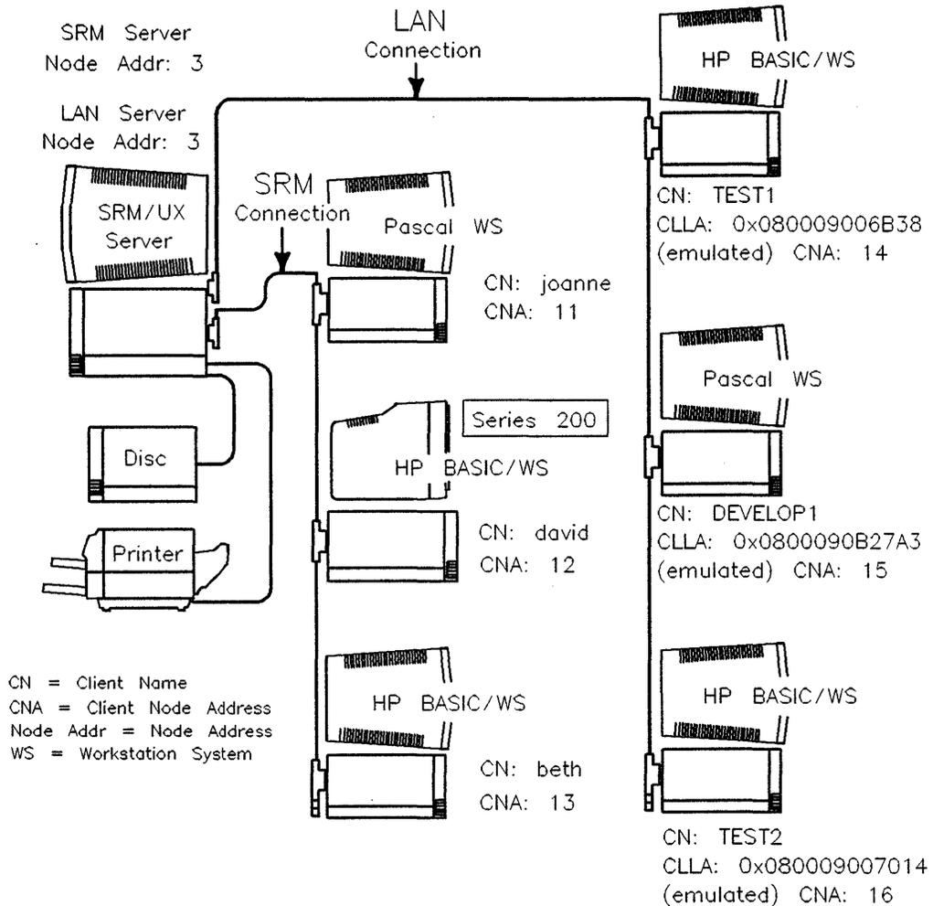
**Figure 2-3. Example SRM/UX System Schematic**
