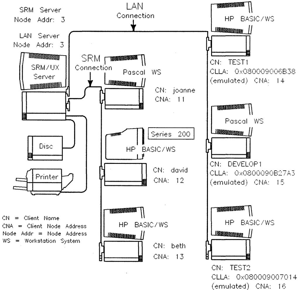
Figure 9-2. Example 2—Multiple Clients on SRM and LAN
