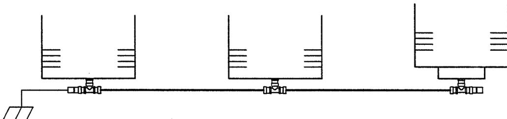
**Figure 3-5. Correct SRM coax connection configuration**
