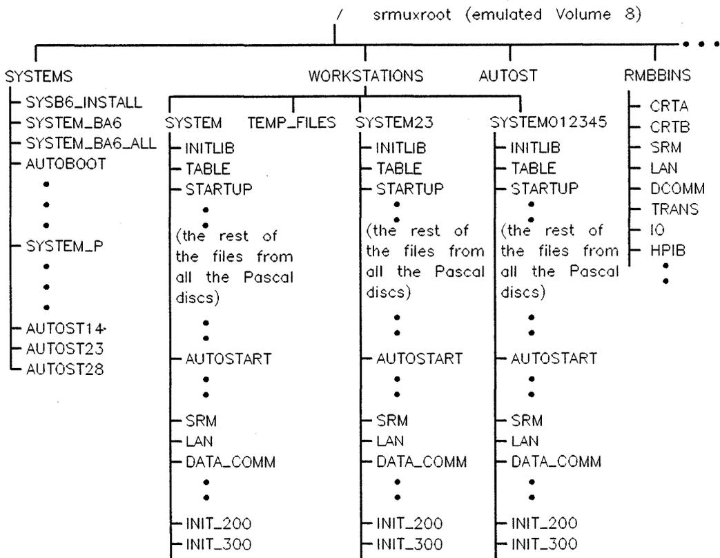
**Figure 4-2. Example SRM/UX File System**
