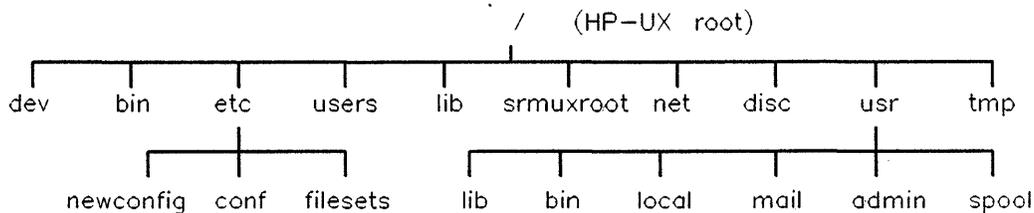
**Figure 2-1. Example HP-UX File System**
