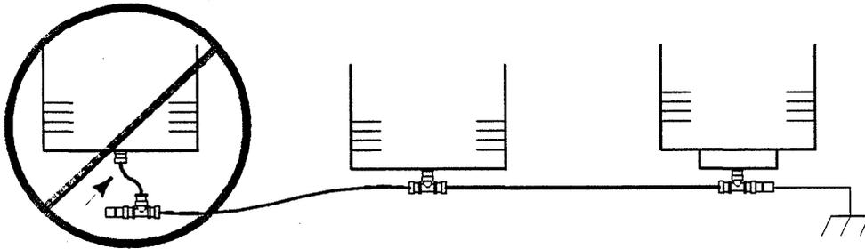
**Figure 3-7. Incorrect SRM coax connection configuration—Example 2**
