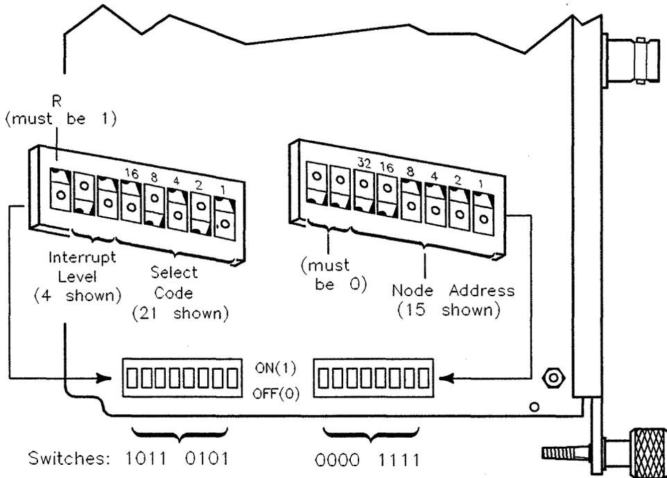
**Figure 3-3. SRM Interface Card—Set Select Code and Node Address**
