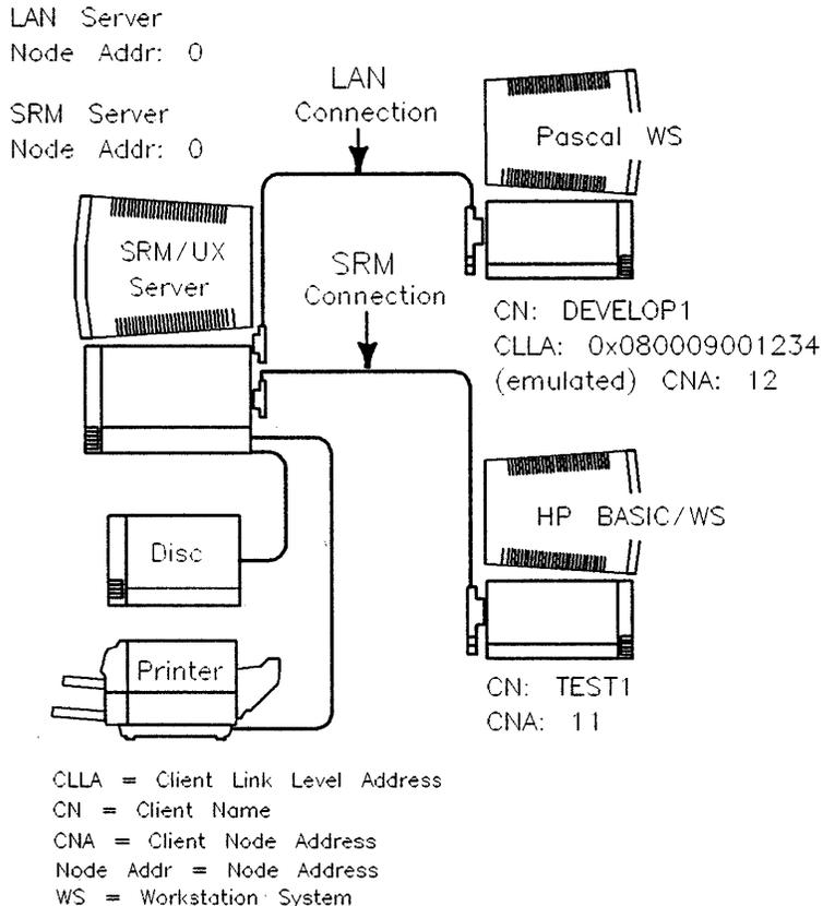
**Figure 9-1. Example 1—A Simple SRM/UX System**
