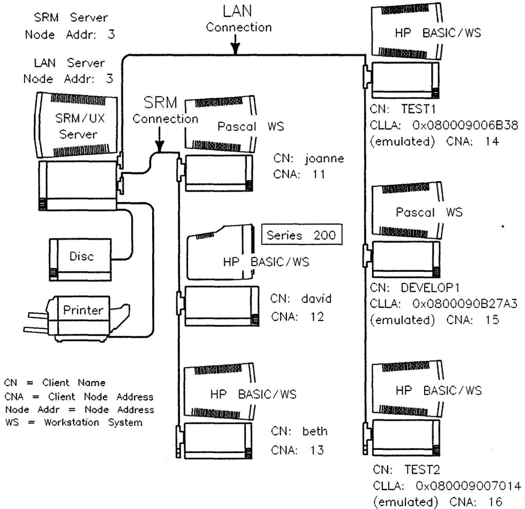
Figure 3-1. Example SRM/UX system (Series 300 server, both connections)
