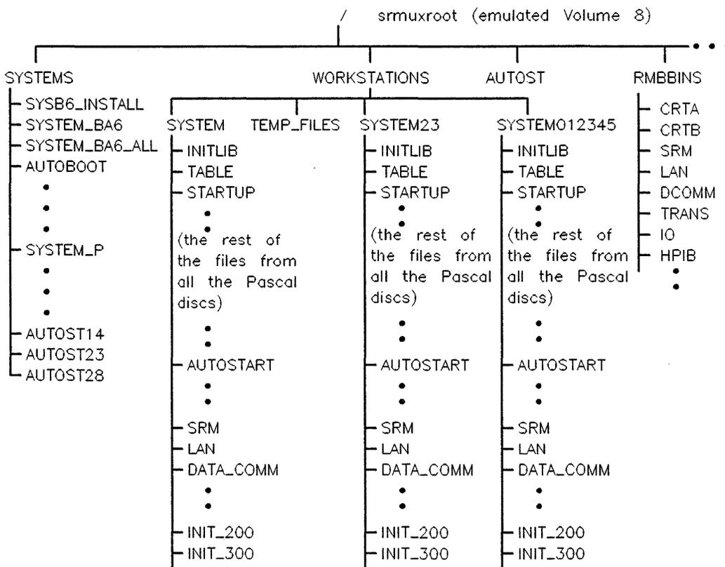
**Figure 2-2. Example SRM/UX File System**
