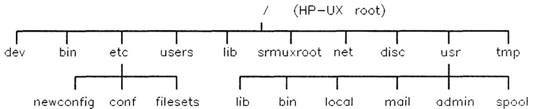
**Figure 4-1. Example HP-UX File System**
