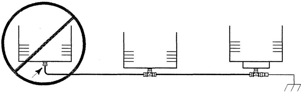
**Figure 3-6. Incorrect SRM coax connection configuration—Example 1**
