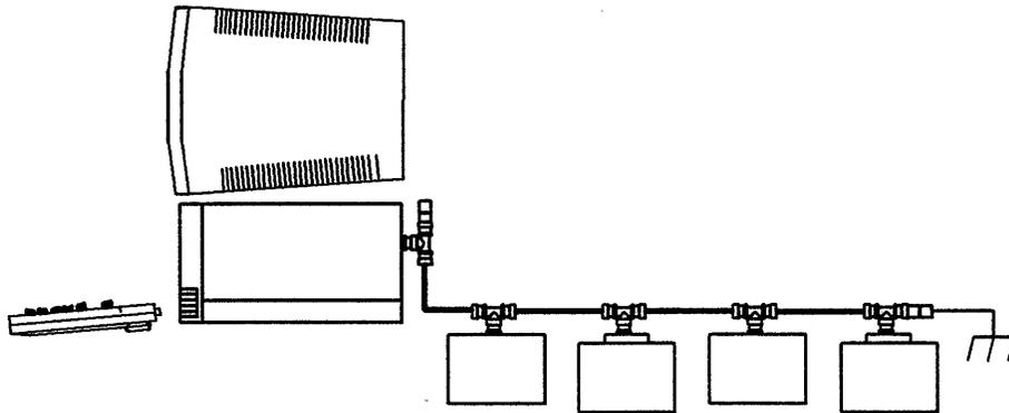
**Figure 3-4. SRM Coax Connection Example**
