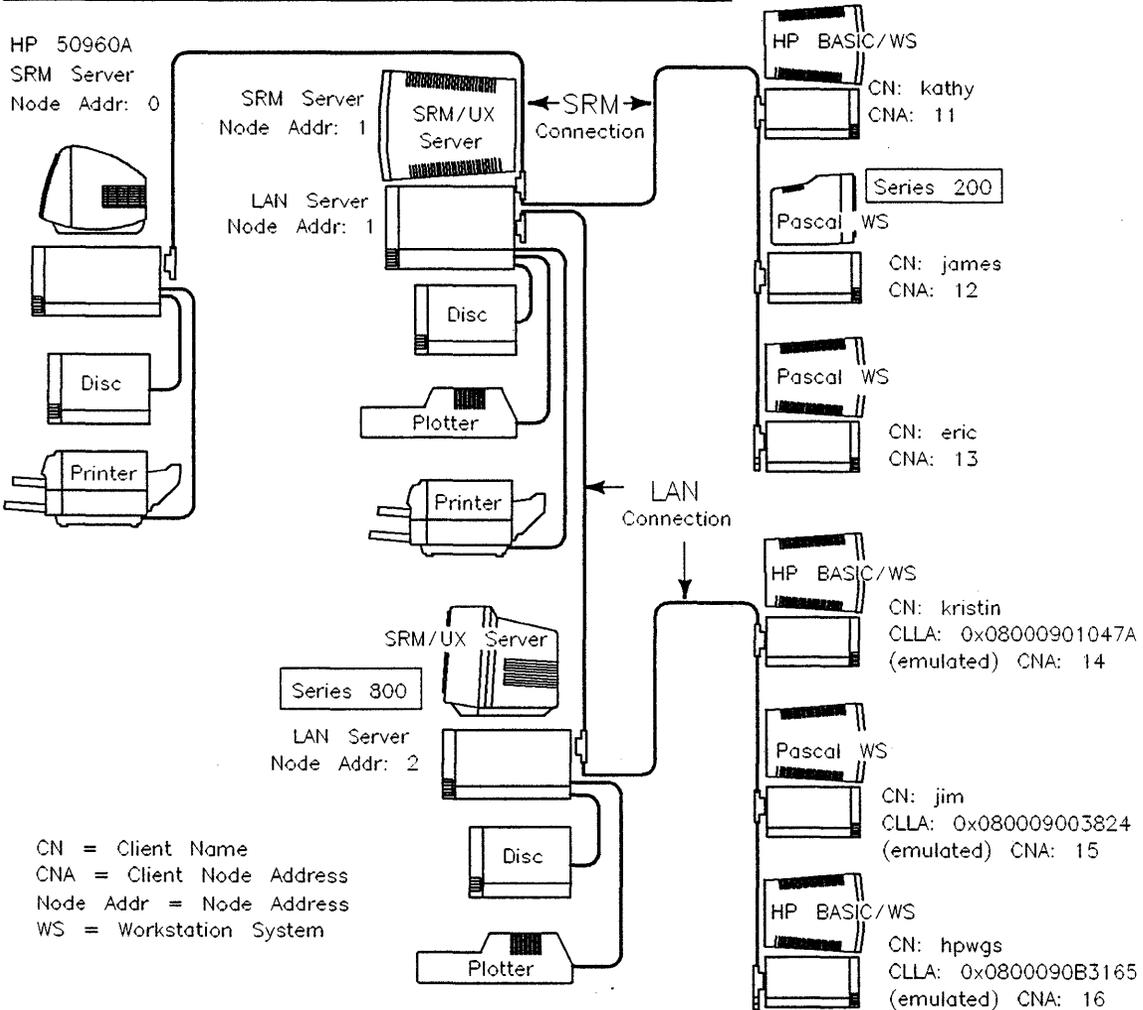
Figure 9-3. Example 3—Multiple Servers, Multiple Clients on SRM and LAN
