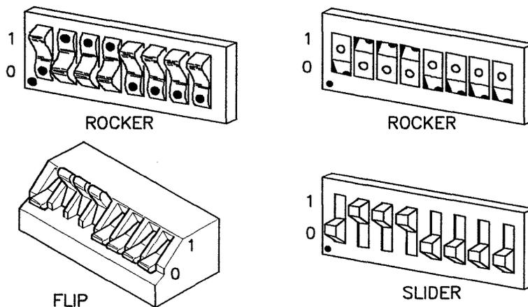
**Figure 3-2. Interface card DIP Switch Types**
