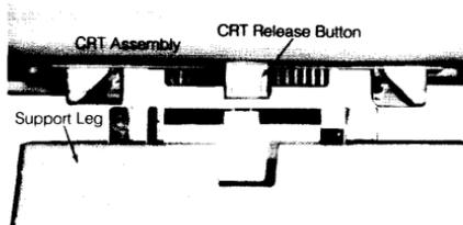
After careful alignment, allow the CRT to rest on the support legs.
