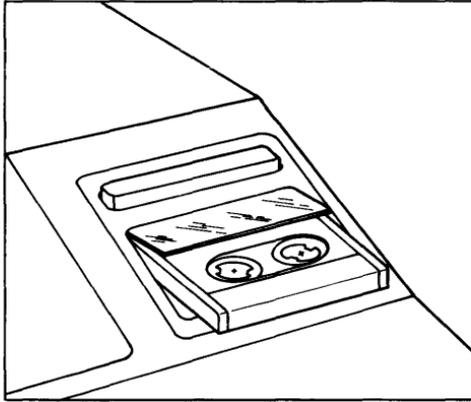
To remove the tape cartridge, press the eject bar. If it is pulled out without pressing the eject bar, another cartridge cannot be inserted until the eject bar is pressed. Do not remove the tape or execute reset while it is moving; damage to the tape may result.
