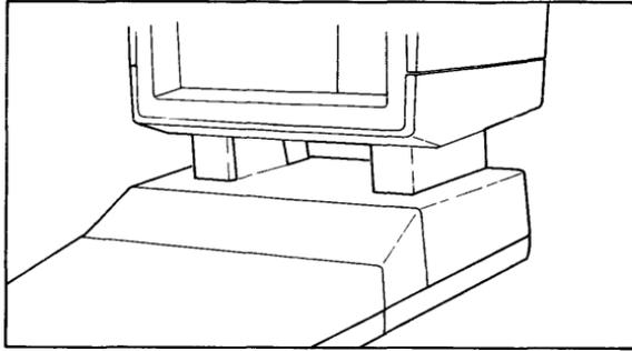
Now push the sliding lock handles in, to secure the CRT to the mainframe.
